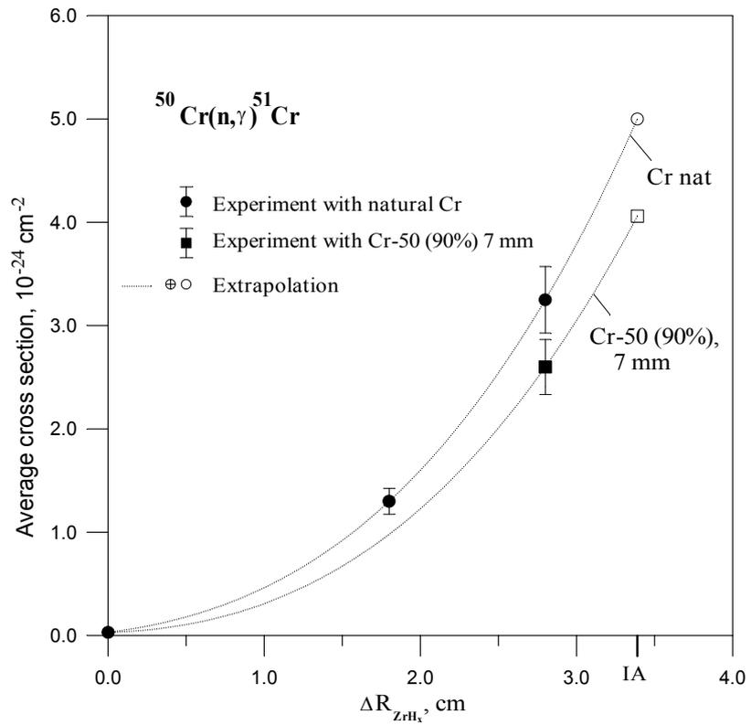
Fig.4. Cr-50 average capture cross section dependence on  $\text{ZrH}_x$  thickness.
