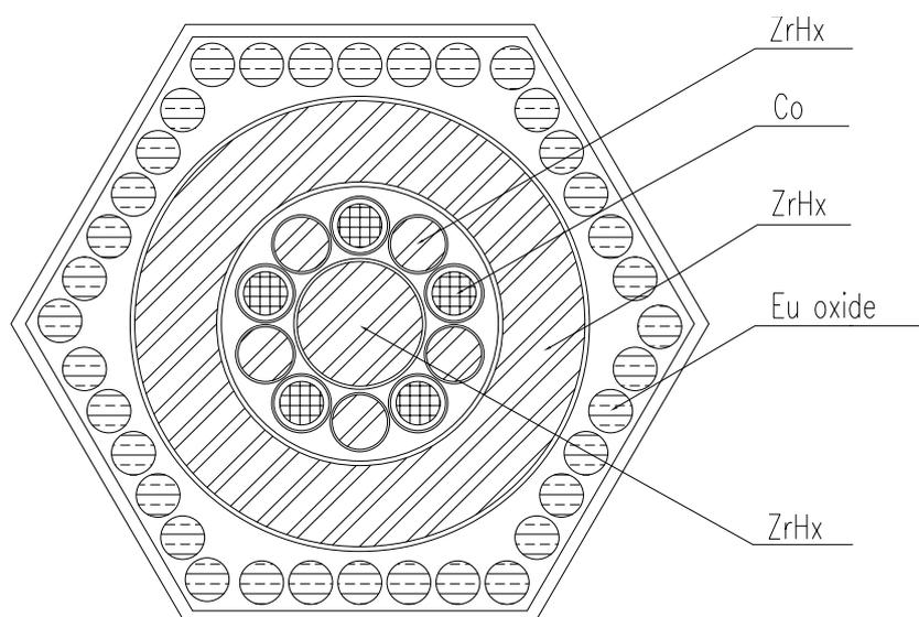
Fig.3. Experimental irradiating assembly for Co-60 production in BN-600 reactor.
