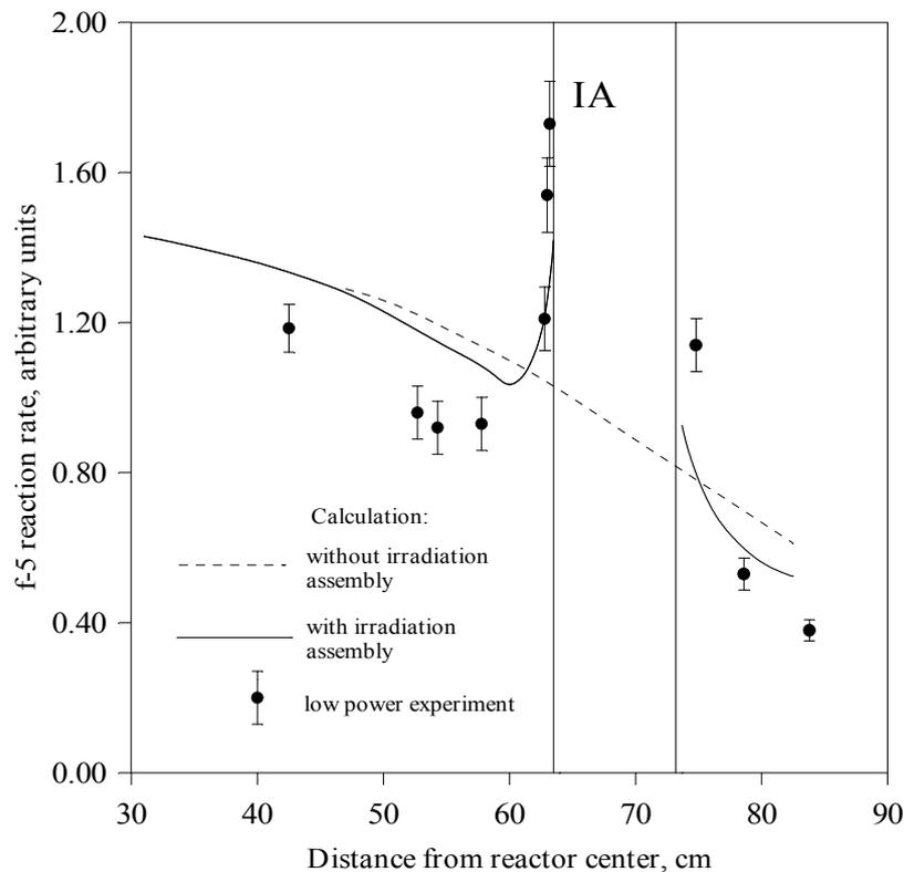
Fig.6. F-5 rate distribution in Cr-51 irradiation assembly area.
