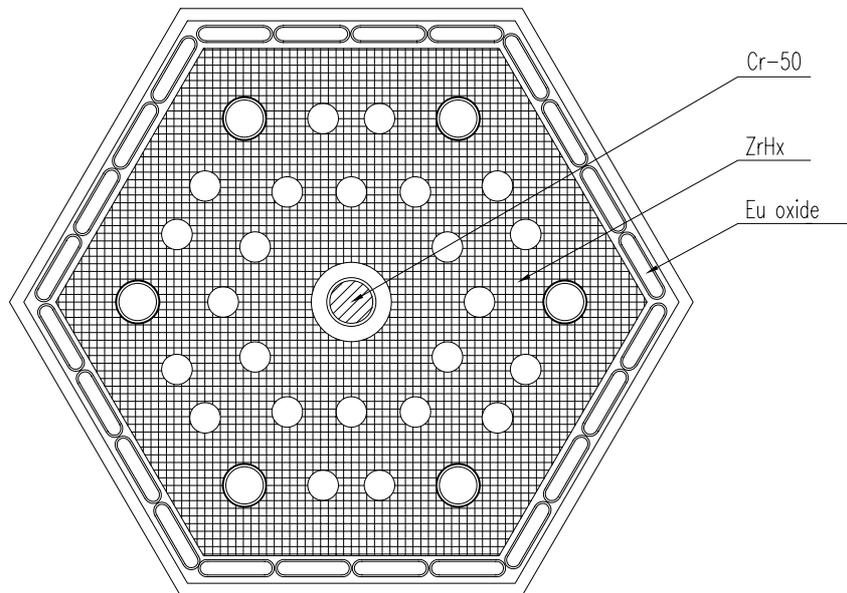
Fig.5. Irradiation assembly for Cr-51 production.
