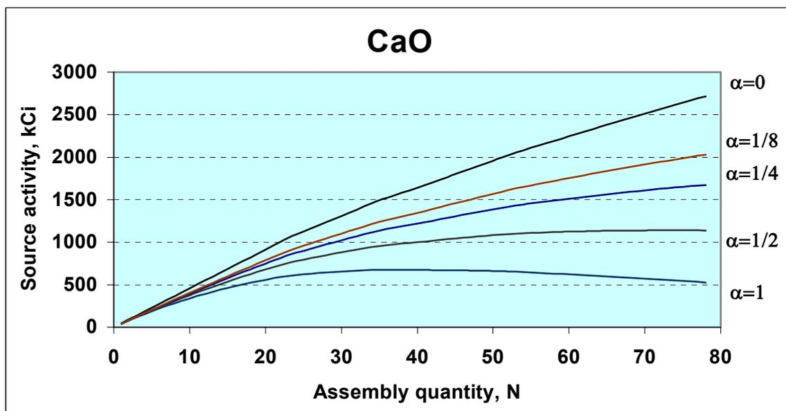
Fig.8. The expected activity of Ar-37 depending on IA amount and handling rate  $\alpha$  (day/assembly).
