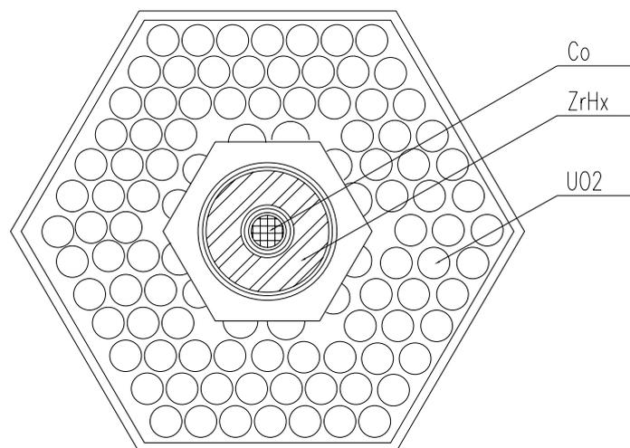
Fig.1. Diagram of experimental IA, tested in BN-350 reactor.
