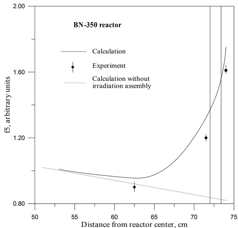
Fig.2. Distribution of U-235 fission rate near irradiating assembly.
