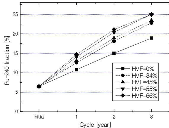
Figure 6. The fraction of  $^{240}\text{Pu}$  in each cycle
