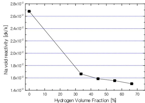
Figure 8. The sodium void reactivity
