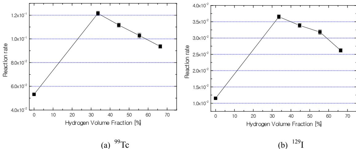
Figure 4. Capture reaction rate of LLFPs
