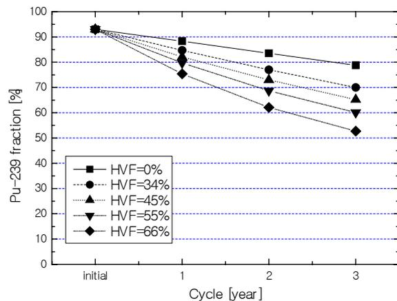
Figure 5. The fraction of  $^{239}\text{Pu}$  in each cycle
