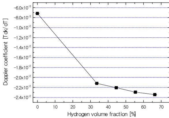
Figure 7. The Doppler reactivity coefficients
