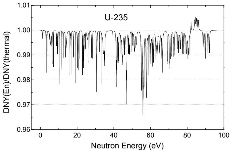
Fig.5 DNY ratio relative to thermal fission value for resonances of U-235.
