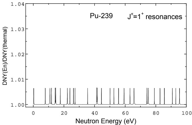
Fig.6 DNY ratio relative to thermal fission value for  $1^+$ -resonances of Pu-239
