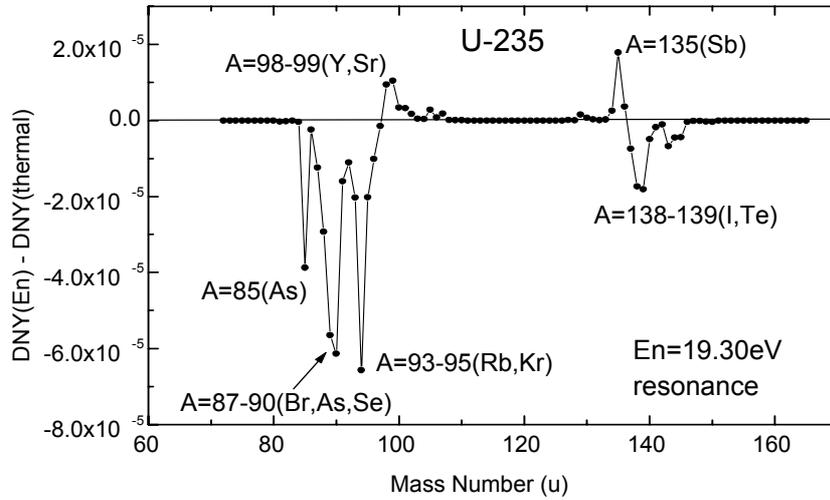
Fig.3. DNY at 19.30eV-resonance relative to thermal fission value of U-235
