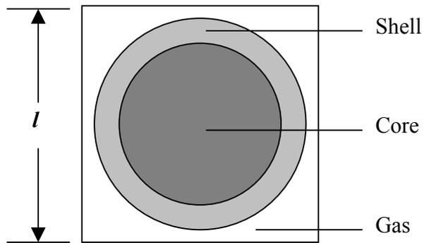
Figure 4. Cross-sectional view of single pebble cell.
