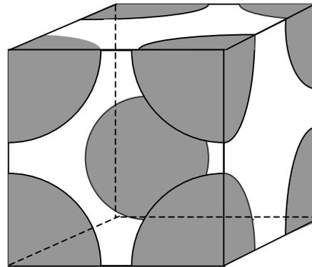
Figure 2. Body centered cubic cell.
