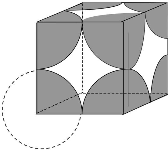
Figure 1. Simple cubic cell.
