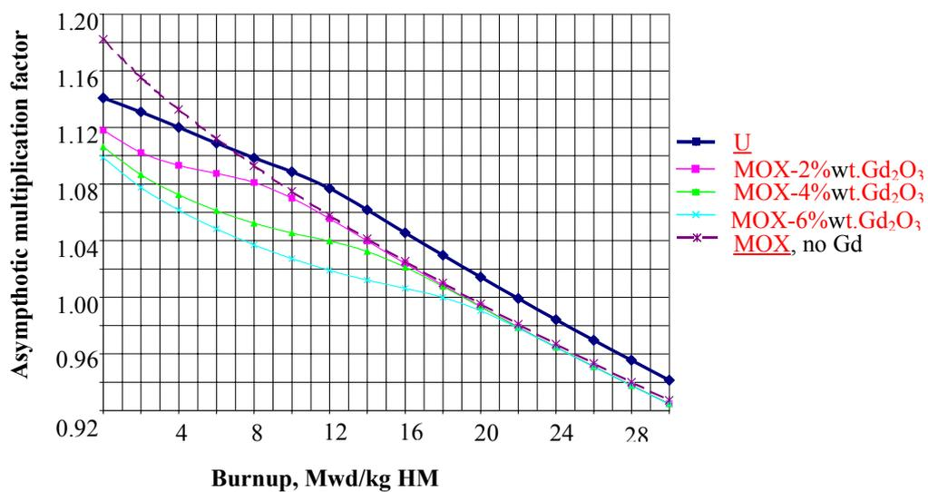
Fig.2.4 Multiplication factor of Uranium and MOX assemblies during irradiation for different gadolinium content in tvegs. Cb=1400 ppm
