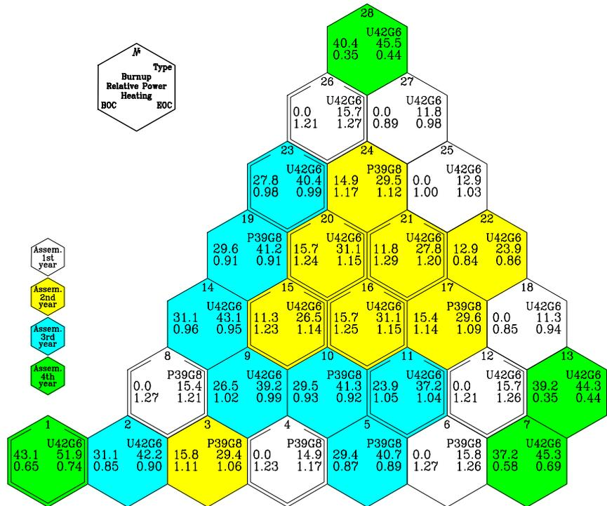
Fig.3.1 Assembly-by-assembly Power and Burnup Distributions and Reloading Scheme. Equilibrium cycle with 30% MOX fuel
