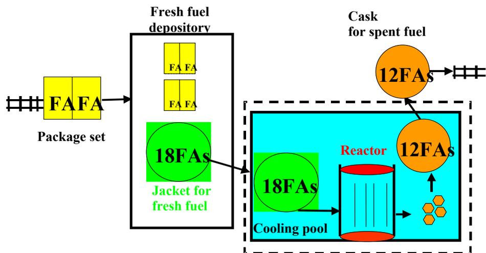
Fig. 4.1 Transportation scheme at VVER-1000 NPP
