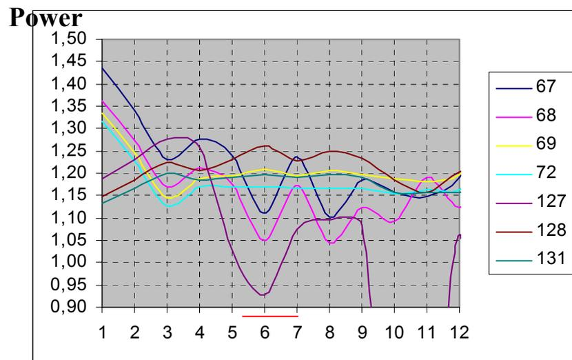
Fig. 2.6 Relative power distribution in registered fuel pins
