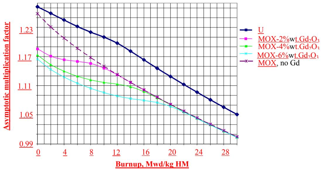
Fig.2.3 Multiplication factor of Uranium and MOX assemblies during irradiation for different gadolinium content in tvegs. Cb=0
