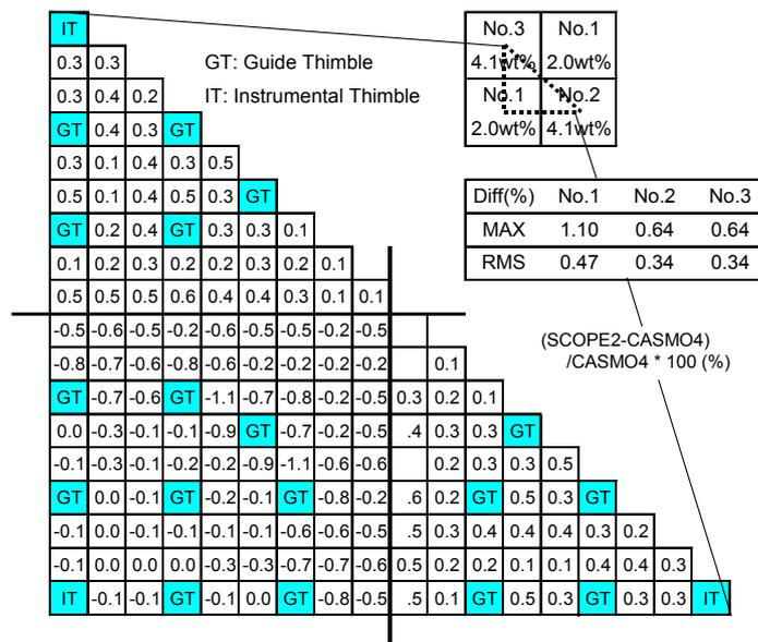
Figure 3. Pin power distribution predicted by SCOPE2 agreed well with that by CASMO-4 in the central zone of 2x2 assembly geometry of 2.0wt% and 4.1wt%  $UO_2$  fuel assemblies.
