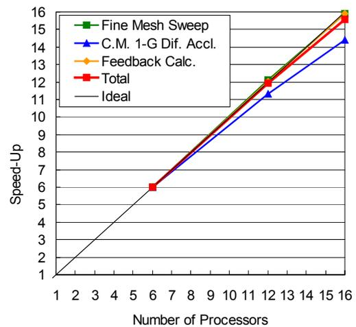
Figure 5. Speed-up curve in 3-D full-core geometry of PWR (340x340x26 meshes)
