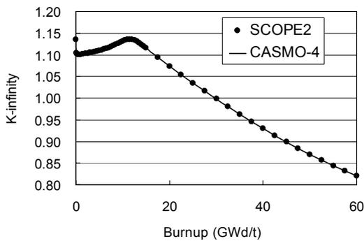
Figure 1. Reactivity change in single assembly geometry predicted by SCOPE2 agreed with the results by CASMO-4 in heterogeneous model used in preparation of cross section library for SCOPE2.
