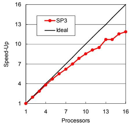
Figure 5. Speed-up curve for 3-D 1/4 core of PWR (170x170x18 meshes)
