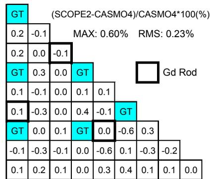
Figure 2. Error of predicted power distribution by SCOPE2 in 4.1wt%  $^{235}U$ -enriched 6wt% Gd fuel assembly at 45GWd/t.
