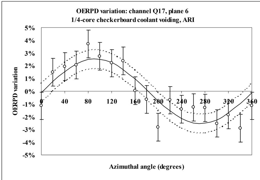
Figure 6. Azimuthal variations in OERPD, channel Q17, plane 6, 1/4-core checkerboard coolant voiding, ARI.
