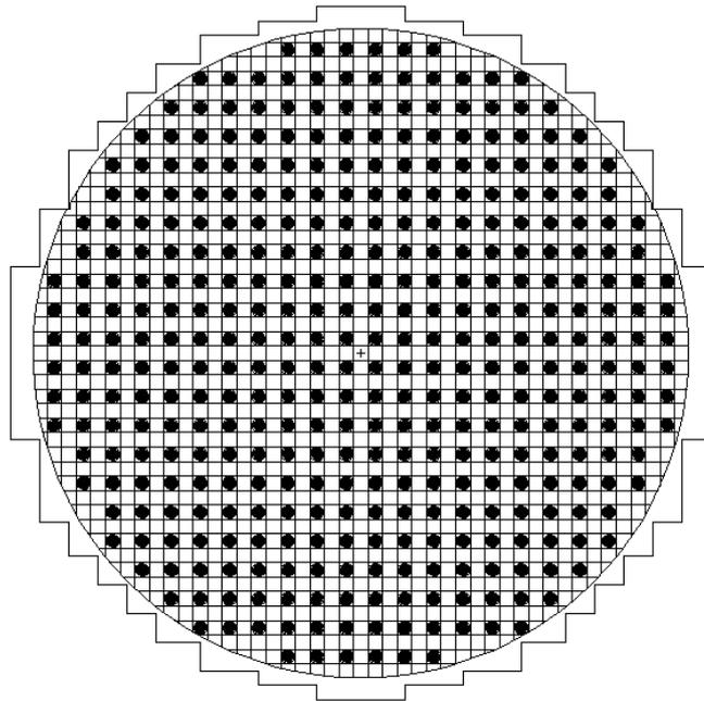
Figure 1. Cross-section of the CANDU 6 MCNP model (near the end face).
