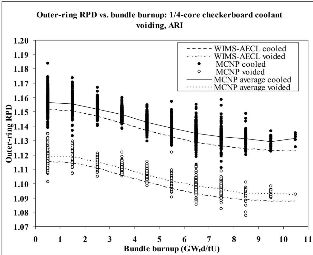
Figure 5. Outer-ring RPD as a function of bundle burn-up, 1/4-core checkerboard coolant voiding, ARI.
