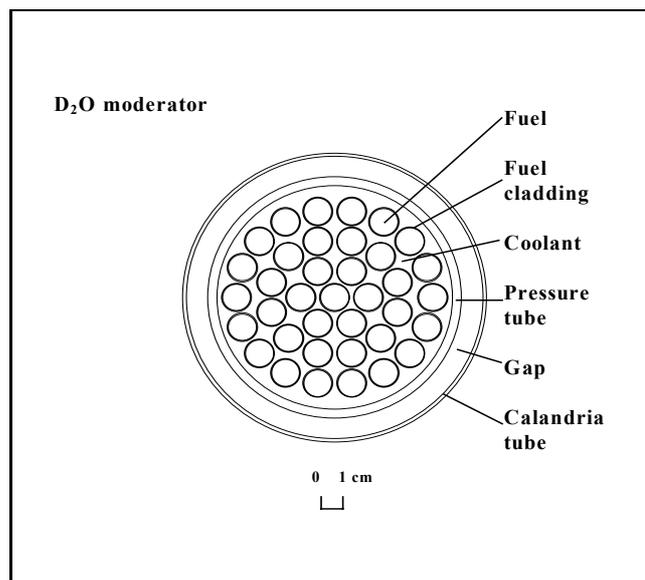
Figure 3. Cross-Section of a 37-Element CANDU Fuel Bundle
