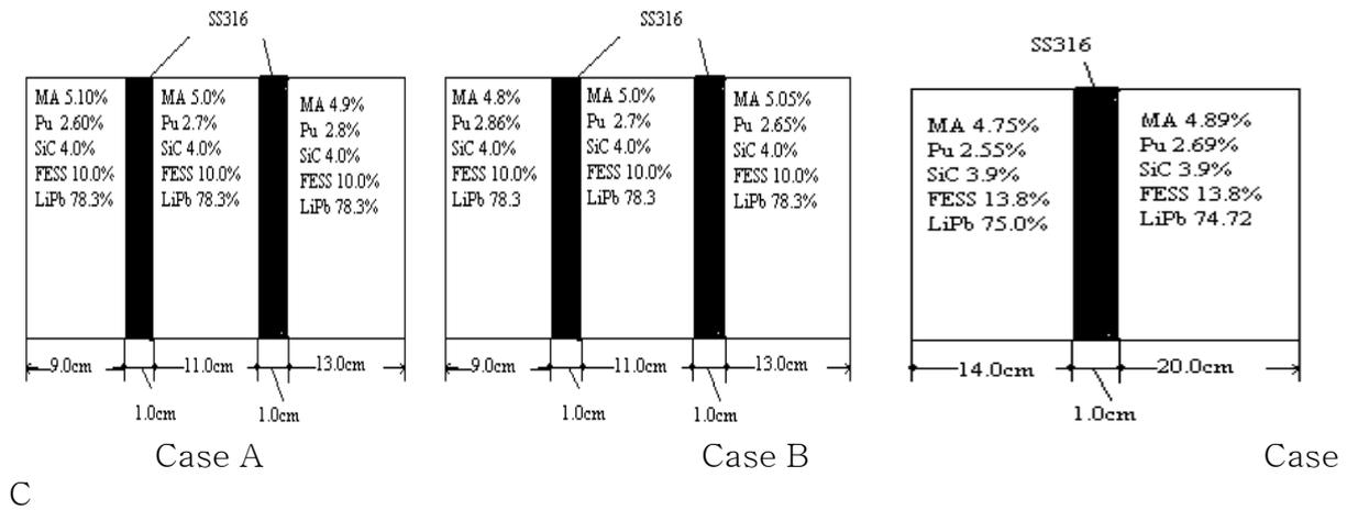
Fig.7 the heterogeneous loading pattern of each case
