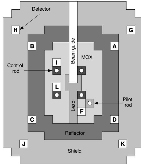
Figure 1. Schematic view of the MUSE-4 core
