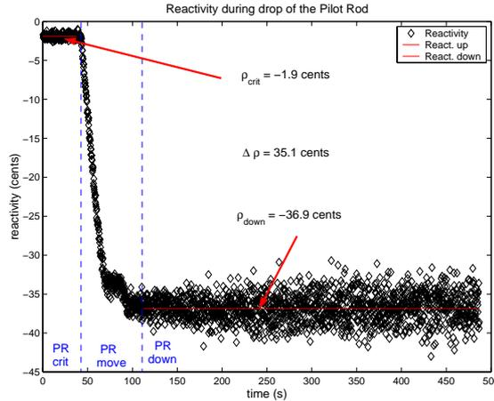
Figure 2. Rod-drop of pilot rod from near critical state to down
