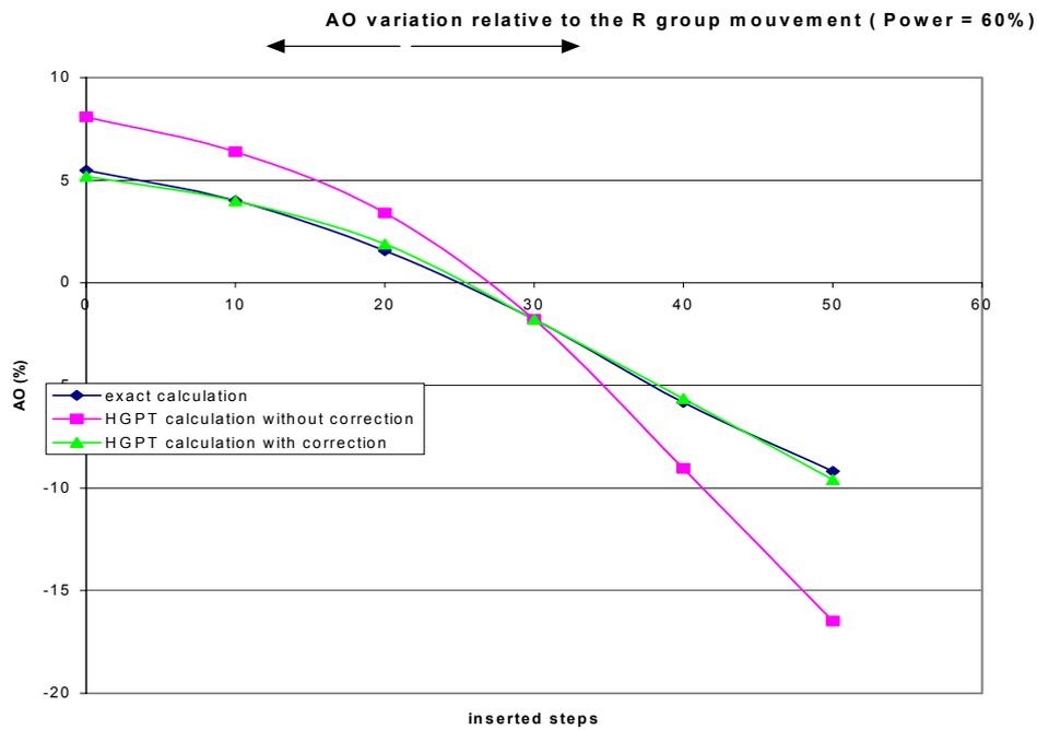
Fig. 9 GPT Axial-Offset reconstruction via HGPT: movement of group R at 60% power
