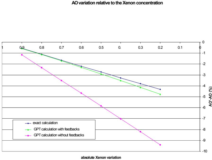
Fig. 5 GPT reconstruction of the Axial-Offset after a change of Xe concentration: effect of  $\delta H$ .
