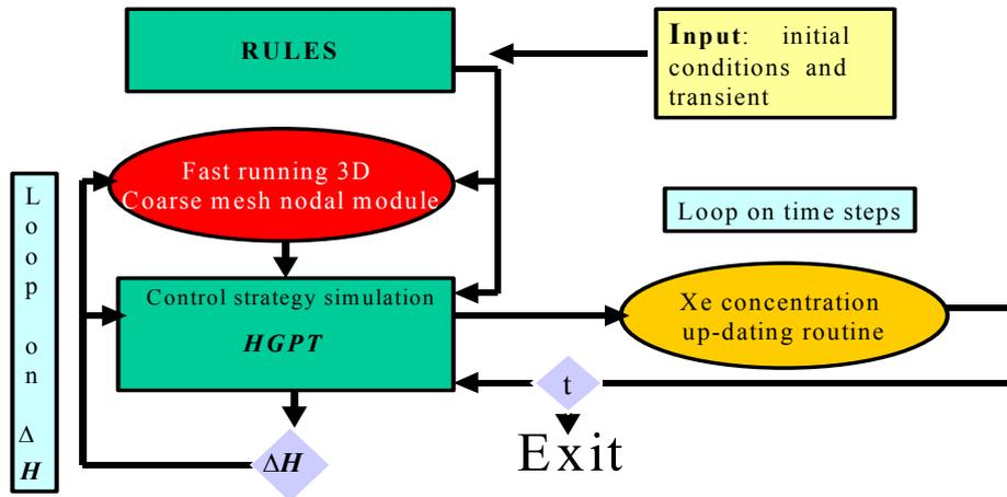
Fig. 3. Simplified scheme of an Operator-Aid System industrial version.
