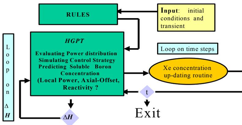
Fig. 2 Operator-Aid System conceptual scheme
