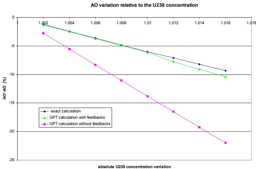
Fig. 4. GPT reconstruction of the Axial-Offset after a local variation of U238 concentration: effect of  $\delta H$ .
