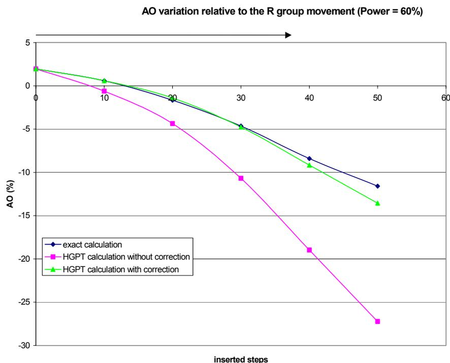
Fig. 8 GPT Axial-Offset reconstruction via HGPT: movement of group R at 30% power
