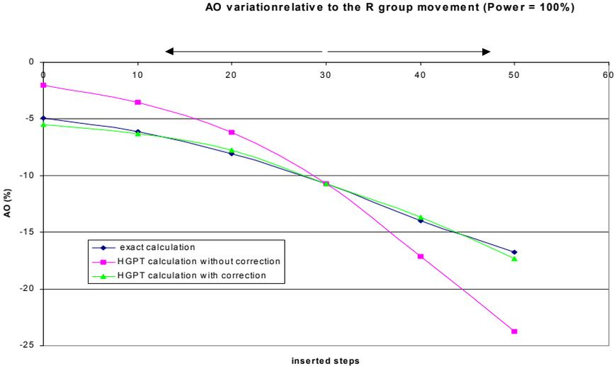
Fig. 7 GPT Axial-Offset reconstruction via HGPT: efficiency of the corrections at full power
