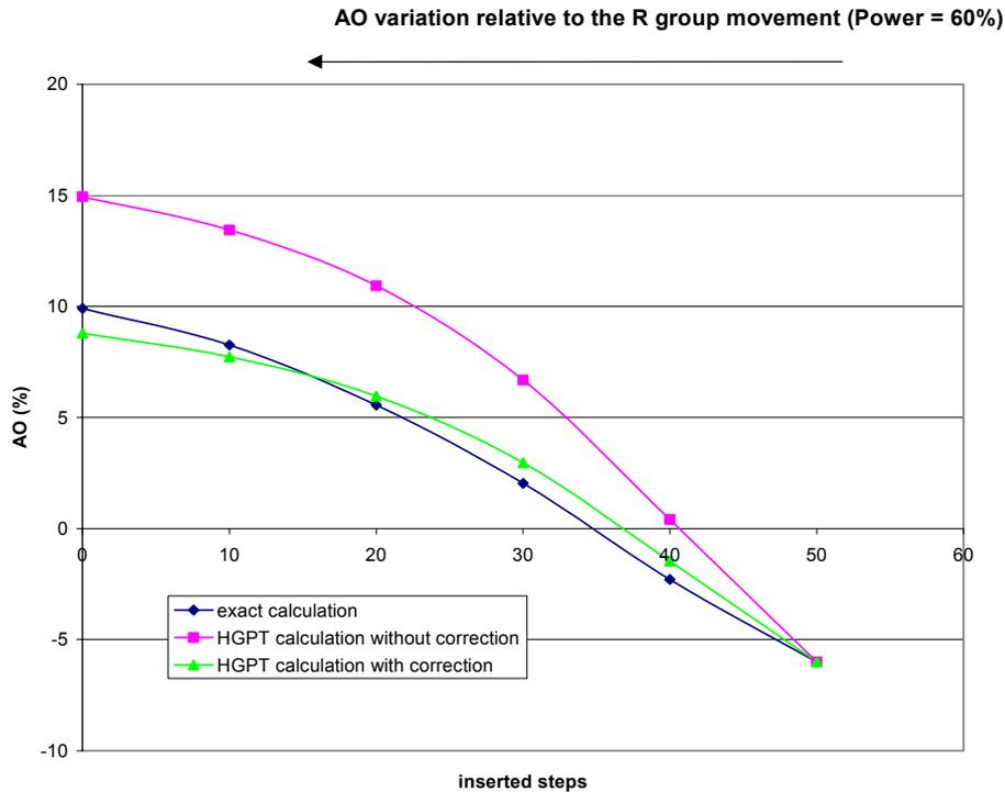
Fig. 11 GPT Axial-Offset reconstruction via HGPT: movement of group R at 60% power
