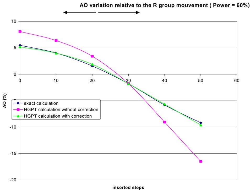
Fig. 10 GPT Axial-Offset reconstruction via HGPT: movement of group R at 60% power
