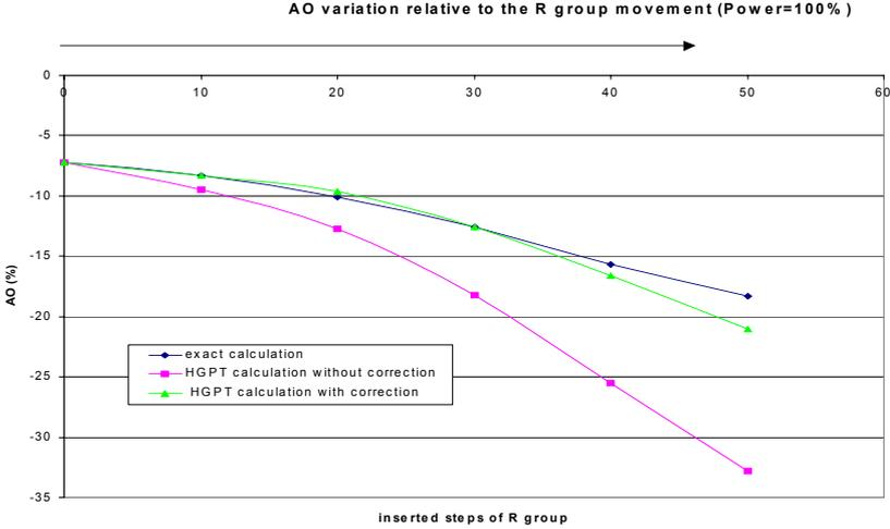
Fig. 6 GPT Axial-Offset reconstruction via HGPT :efficiency of the corrections at full power
