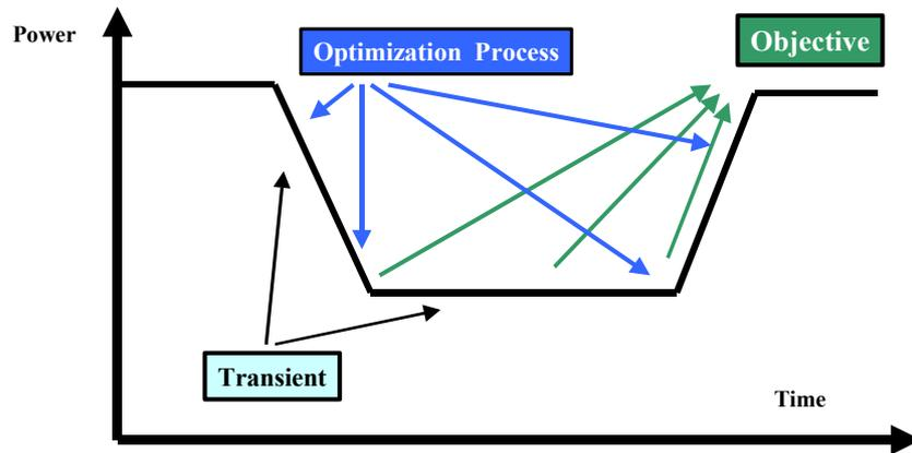
Fig. 1. Typical load-follow transient scheme
