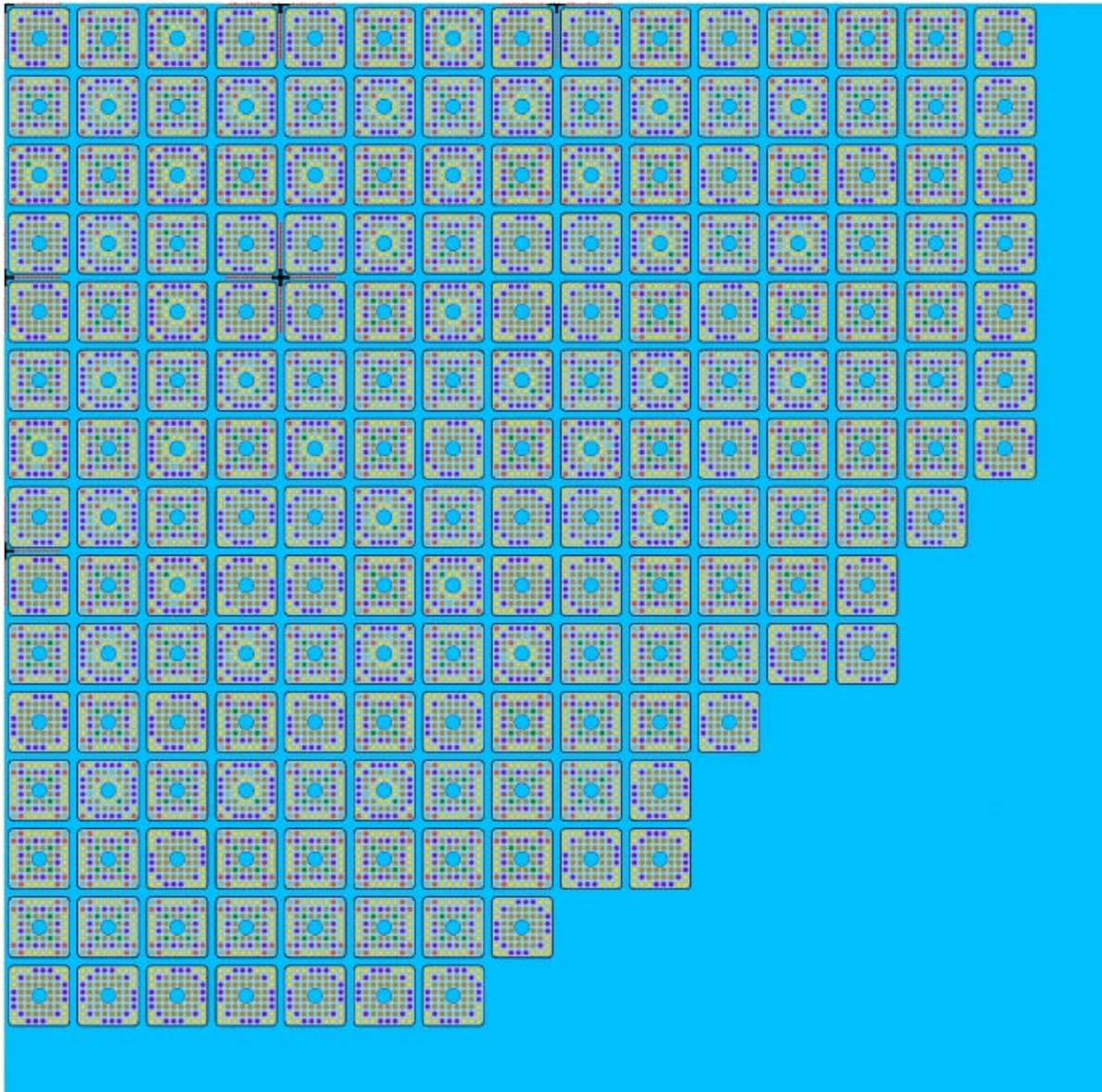
Fig. 8 Quarter-Core BWR Geometry
