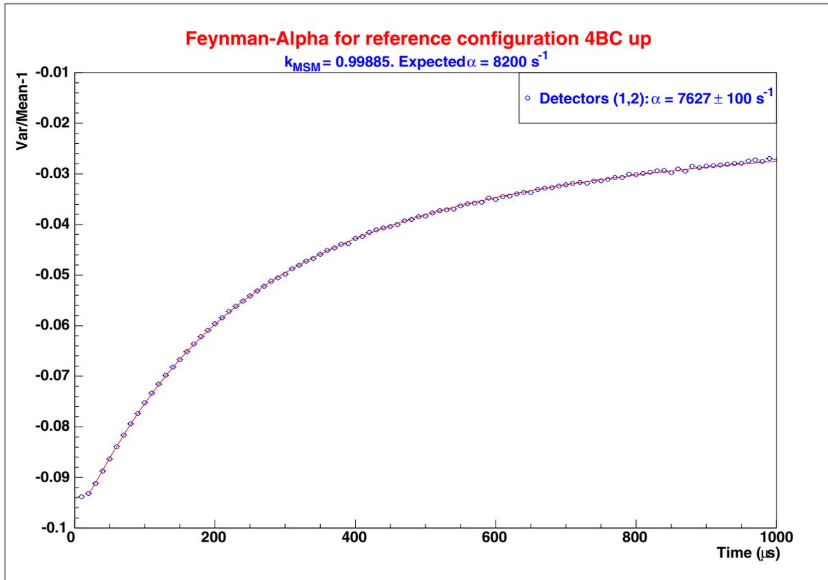
Figure 11. Feynman-Alpha distribution for a configuration close to criticality situation. The detector used is the same than in the Rossi-Alpha case.
