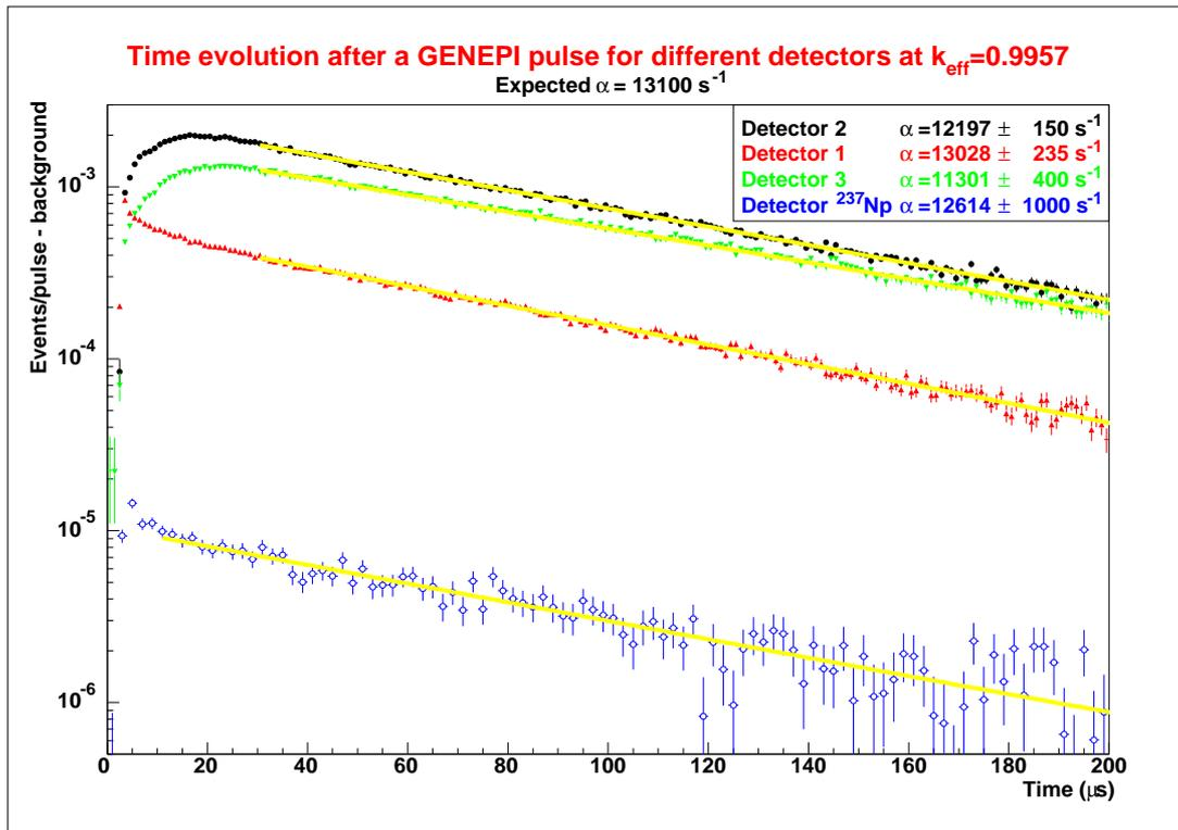
Figure 5. Prompt response of MASURCA after a  $1\mu\text{s}$  neutron burst for a same criticality level in different positions of the MASURCA reactor.
