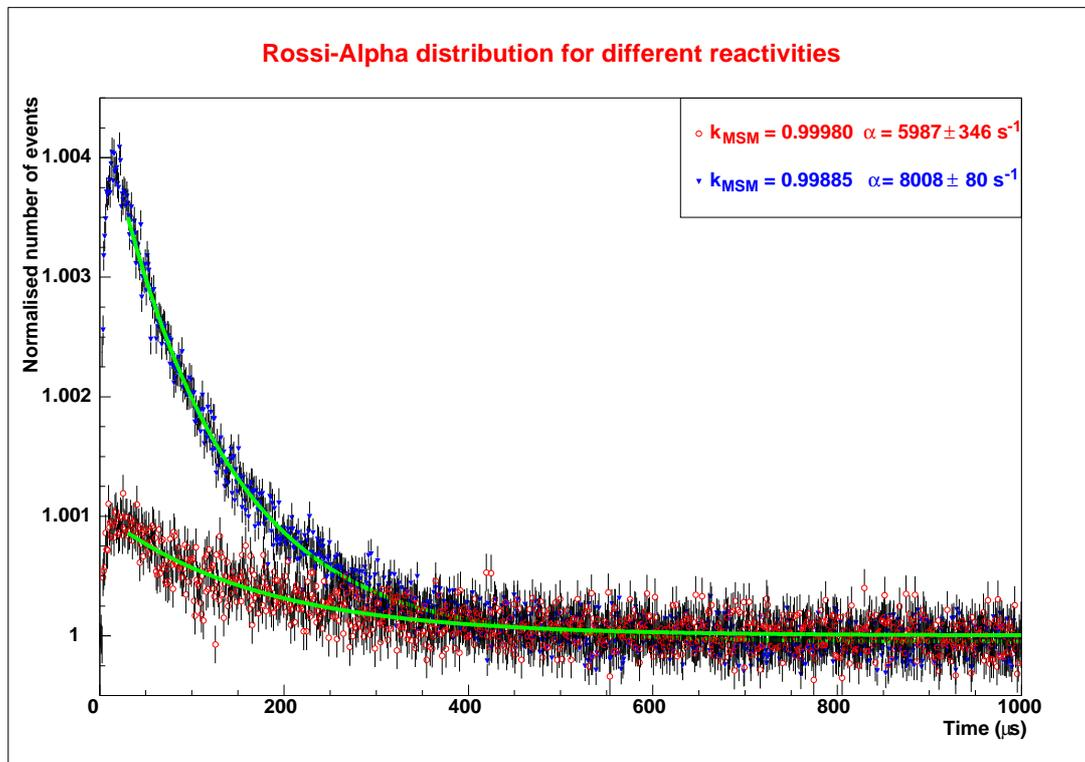
Figure 9. Rossi-Alpha distribution for a detector placed in the reflector region of the MASURCA reactor for two close to criticality configurations.
