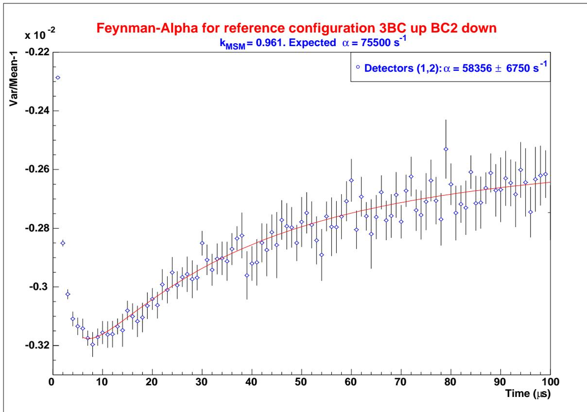
Figure 12. Feynman-Alpha distribution for a subcritical configuration. The detector used is the same than in the Rossi-Alpha case.
