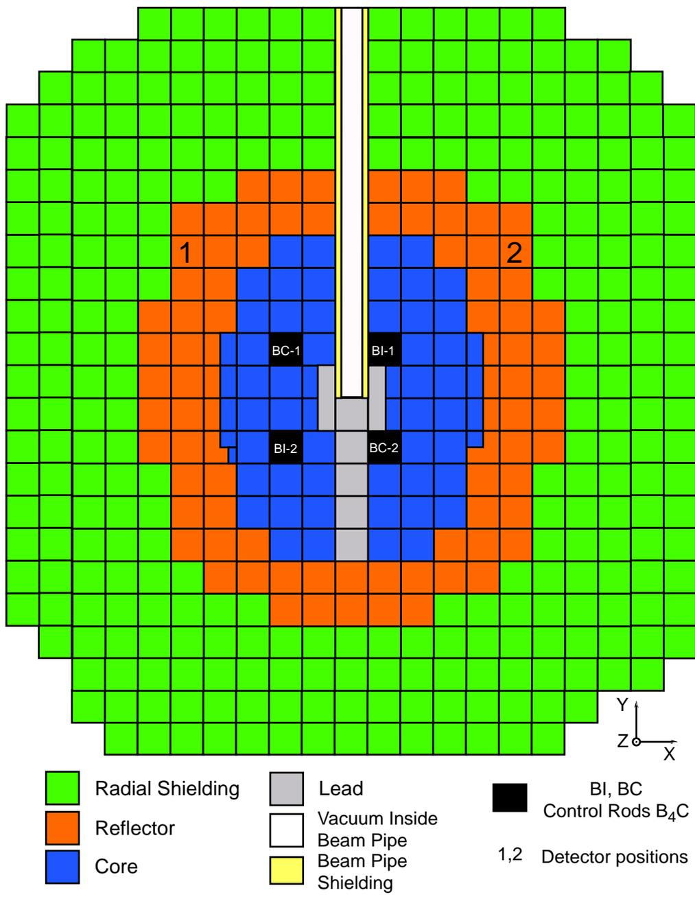
Figure 8. MASURCA loading for the close to criticality noise experiments of the MUSE-4 experiments.
