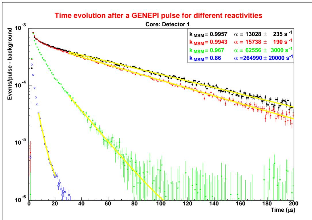
Figure 2. Prompt response of MASURCA after a  $1\mu\text{s}$  neutron burst in a detector placed in the core region for different reactivity levels.
