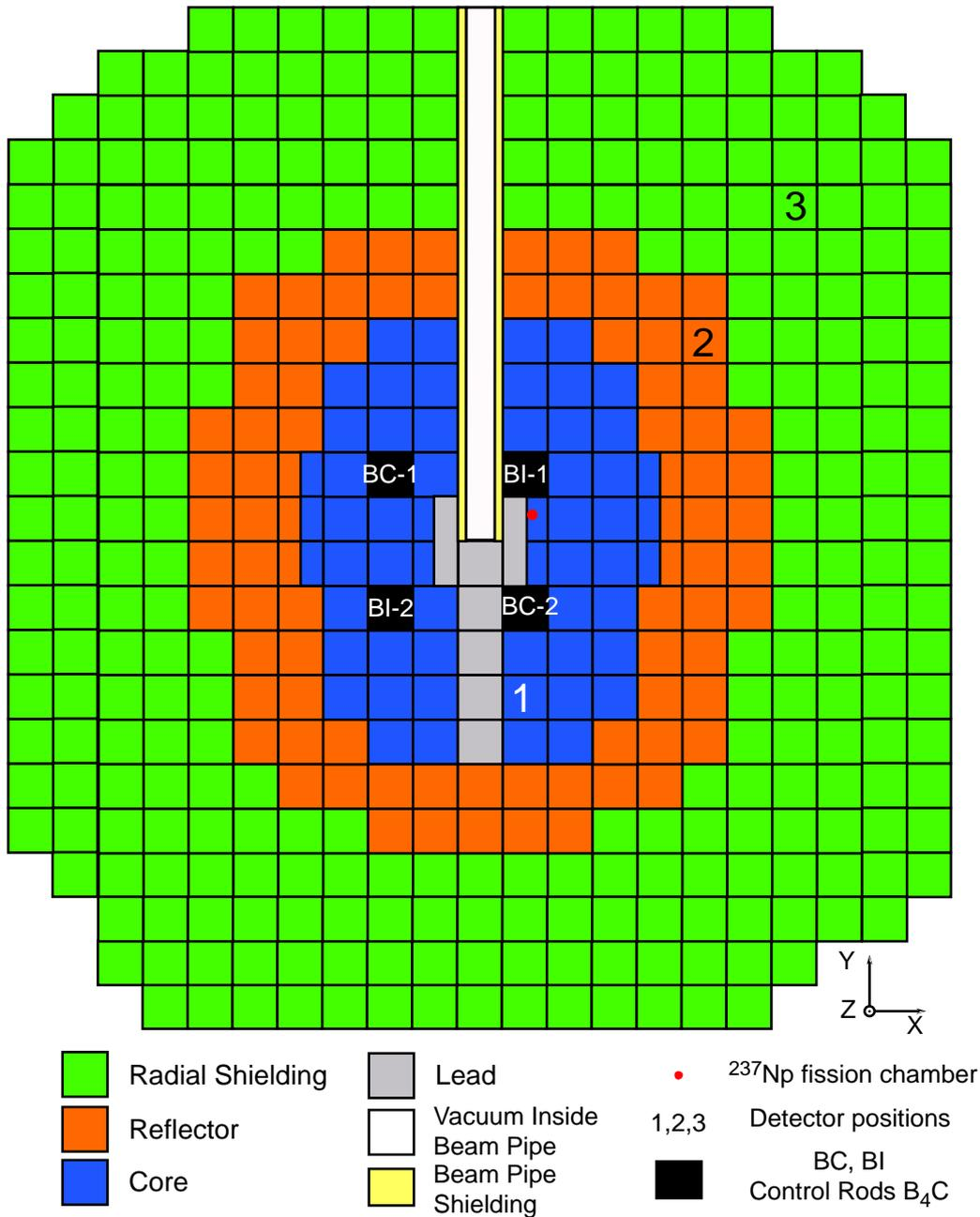
Figure 1. MASURCA loading for the first subcritical configuration of the MUSE-4 experiments.
