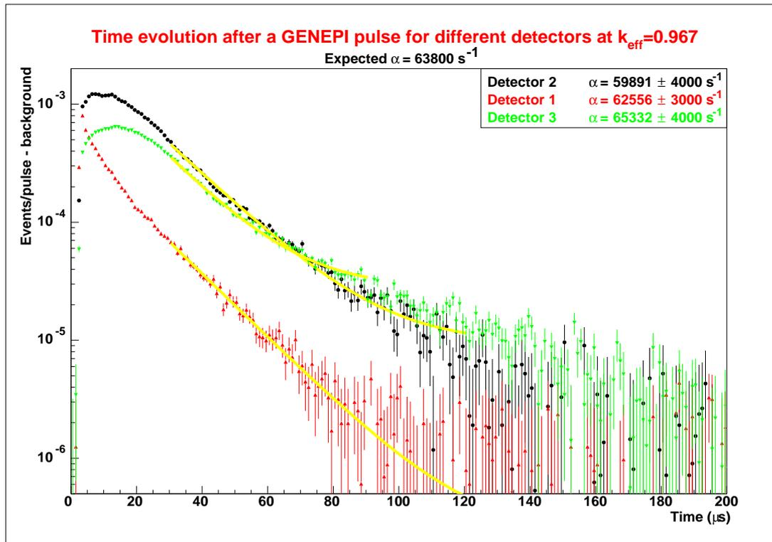
Figure 7. Prompt response of MASURCA after a 1 $\mu$ s neutron burst for a same criticality level in different positions of the MASURCA reactor.
