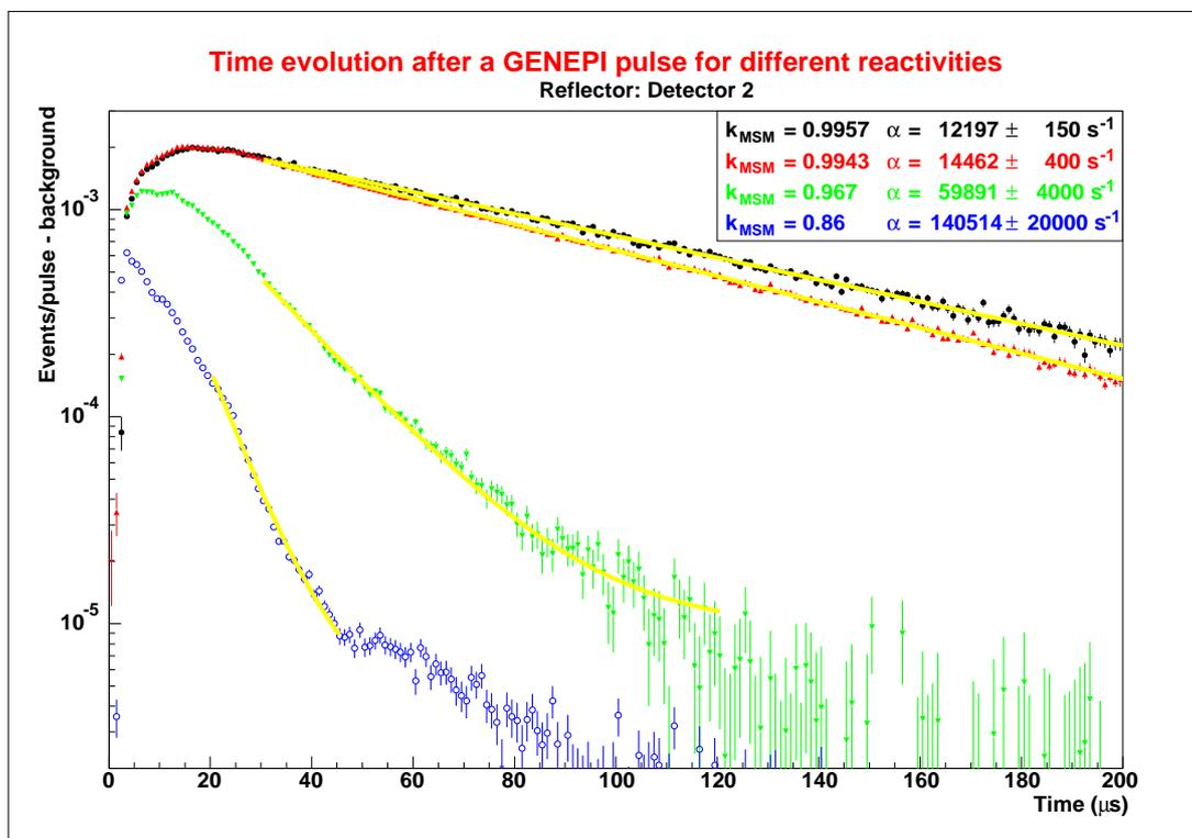
Figure 3. Prompt response of MASURCA after a  $1\mu\text{s}$  neutron burst in a detector placed in the reflector region for different reactivity levels.
