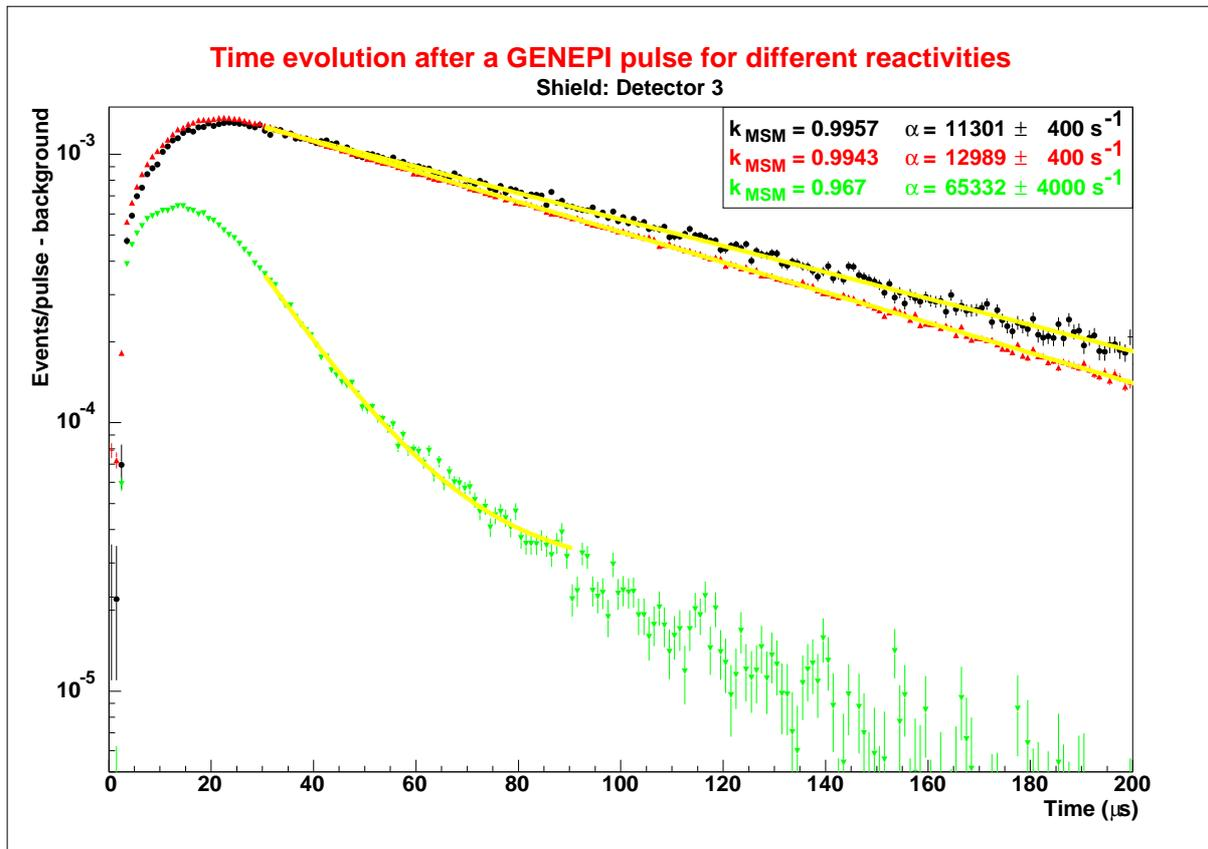
Figure 4. Prompt response of MASURCA after a 1μs neutron burst in a detector placed in the shielding region for different reactivity levels.
