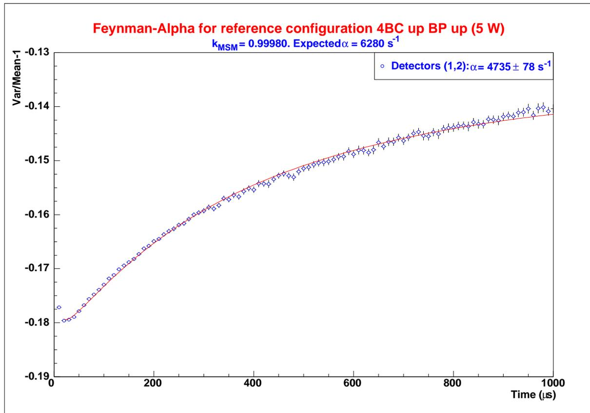
Figure 10. Feynman-Alpha distribution for a configuration close to criticality situation. The detector used is the same than in the Rossi-Alpha case.
