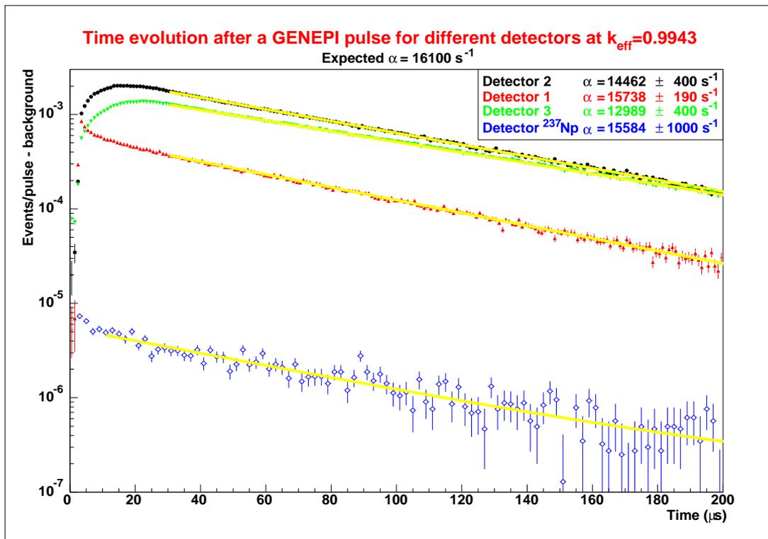
Figure 6. Prompt response of MASURCA after a  $1\mu\text{s}$  neutron burst for a same criticality level in different positions of the MASURCA reactor.
