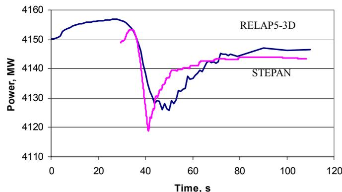
Figure 6. Total reactor core power versus time. Feedwater flow perturbation experiment
