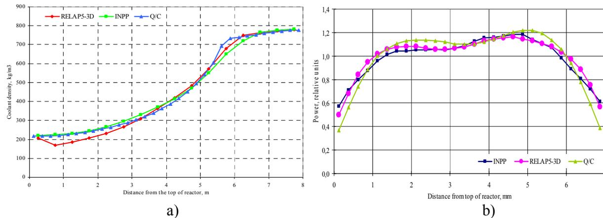
Figure 5. Comparison of the axial coolant density (a) and power (b) distribution profiles as calculated by RELAP5-3D and QUABOX/CUBBOX codes with the real plant data
