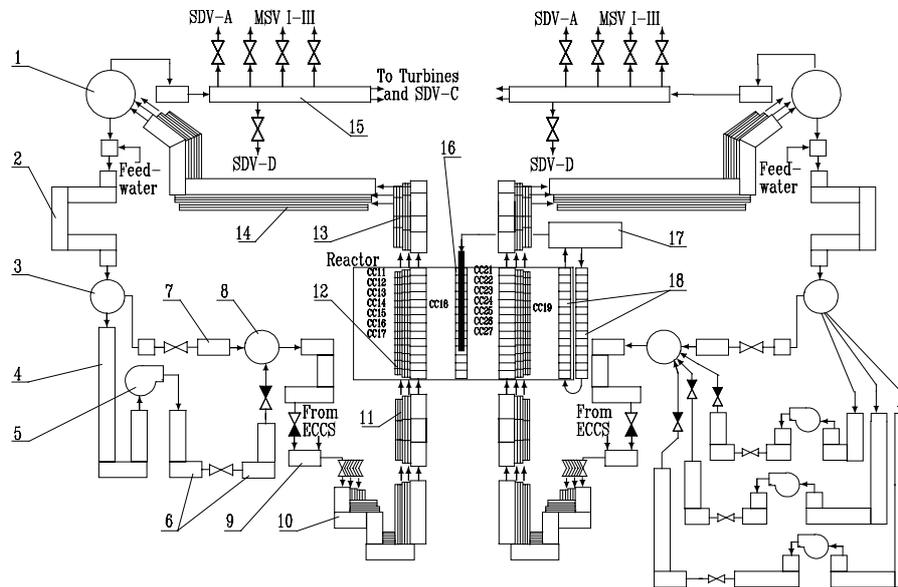
Figure 1. Ignalina NPP thermal-hydraulic model nodalization diagram:
