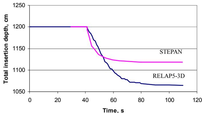
Figure 8. Total insertion depth of four automatic regulators. Feedwater flow perturbation experiment.
