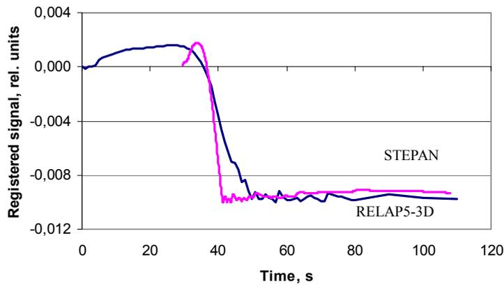
Figure 7. Summary signal of four lateral fission chambers. Feedwater flow perturbation experiment.
