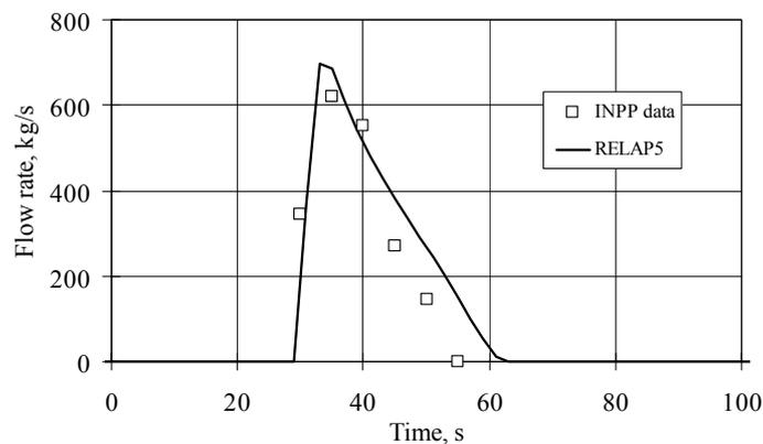
Figure 3. Inadvertent actuation of ECCS event. Mass flow from the ECCS accumulators
