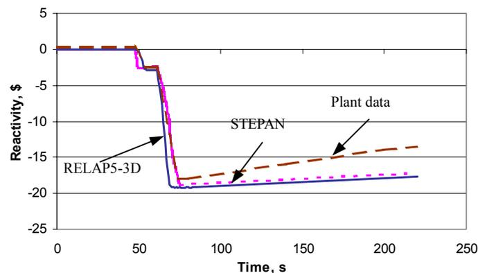
Figure 10. Calculation “counter” reactivity behavior during the reactor shutdown transient.
