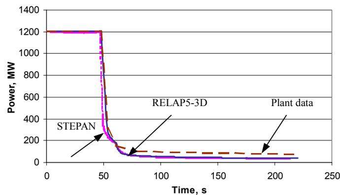
Figure 9. The total reactor core power behavior versus time during the reactor shutdown transient.
