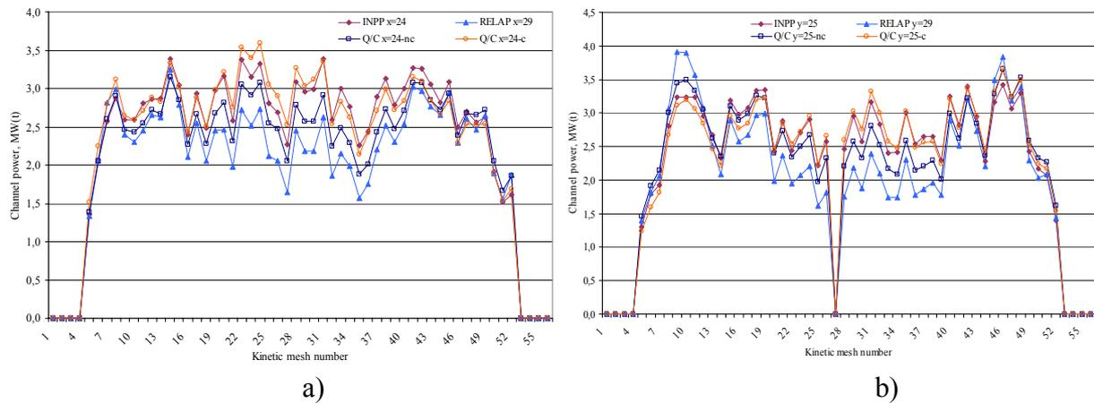
Figure 4. Comparison of the radial power distribution as calculated by codes RELAP5-3D and QUABOX/CUBBOX with the real plant data in X (a) and Y (b) directions in the center of the core
