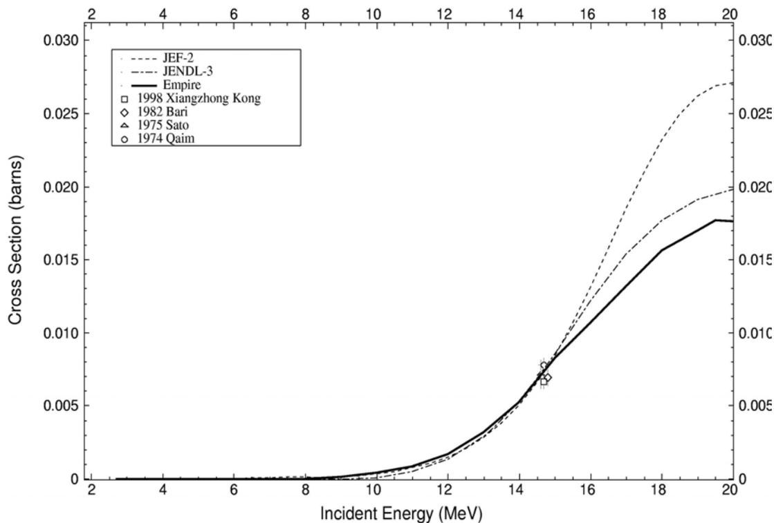
Fig. 3. (n, p) cross section for Sm-150.
