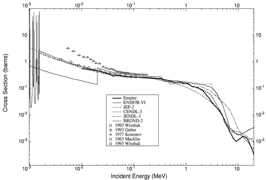
Fig. 2. Capture cross section for Sm-150.
