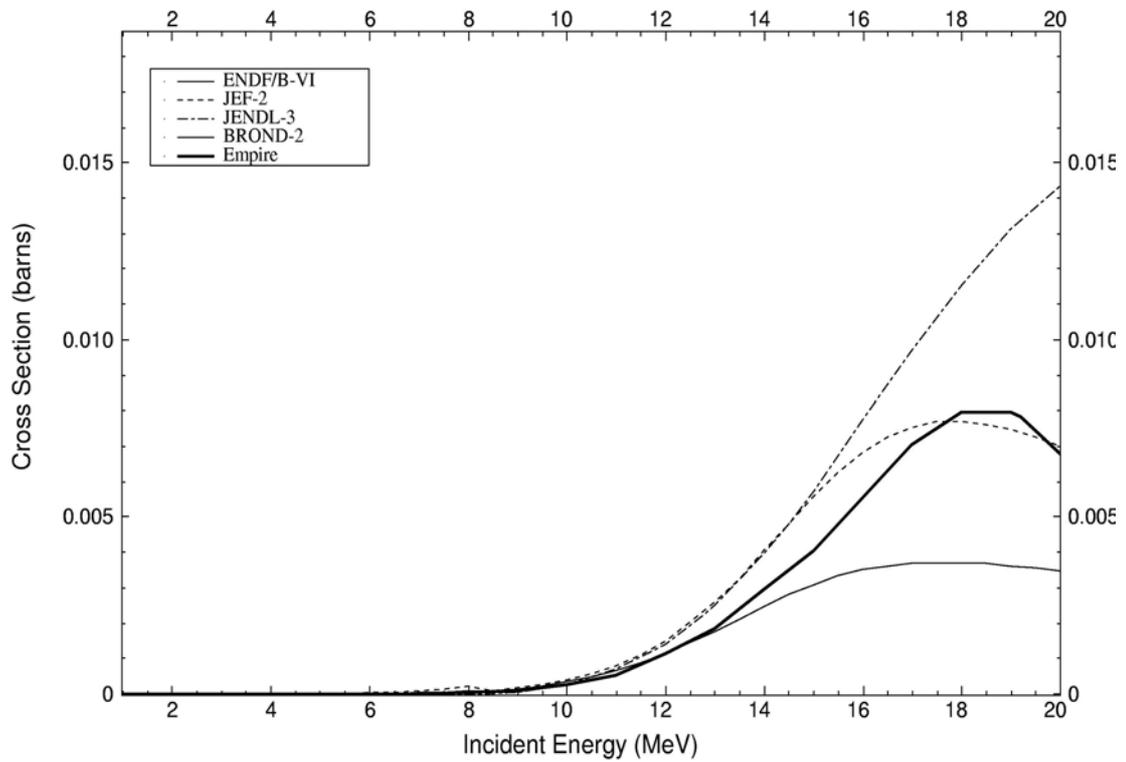
Fig. 6. (n, p) cross section for Sm-152.
