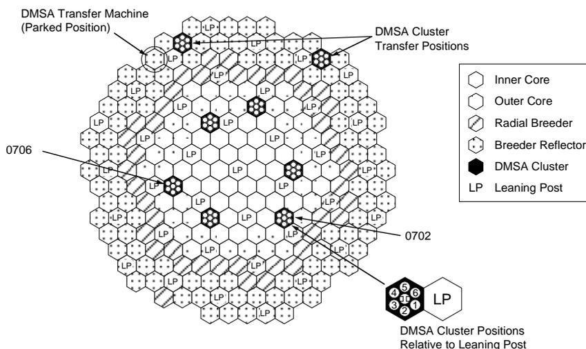
Figure 1. Core showing DMSA experimental positions
