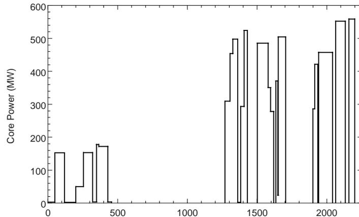
Figure 2 The power history simulation used in the calculations. Days are counted from July 1, 1982.
