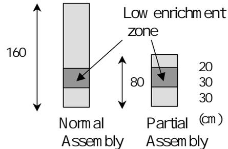
Fig. 6 Axial Pu Enrichment Distribution
