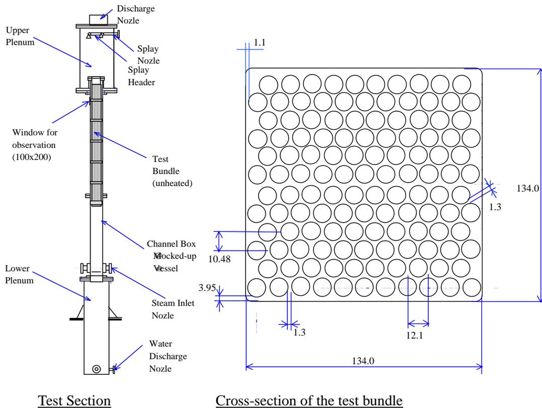
Fig. 11 CCFL test section and cross-sectional geometry of the test bundle
