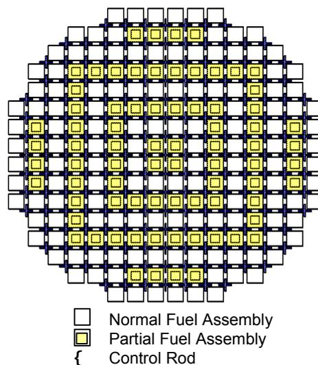
Fig. 3 BARS Core Layout
