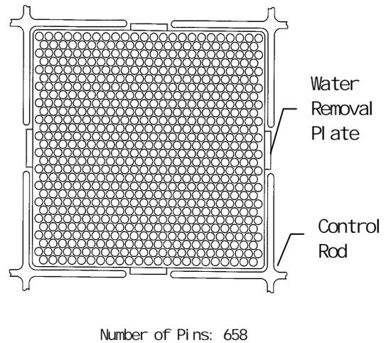
Fig. 4 Vertical View of Fuel Assemblies      Fig. 5 Horizontal Cross Section of Fuel Assembly
