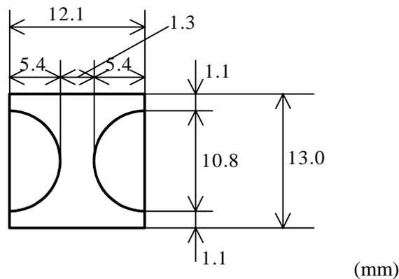
Fig. 8 Flow geometry of the test channel for Visualization test
