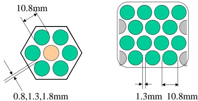
Fig. 9 Cross-sectional Views of the test bundle for the high-pressure thermal-hydraulic test
