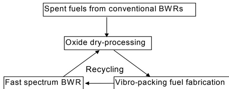
Fig. 1 Concept of BARS (BWR with Advanced Recycle System)
