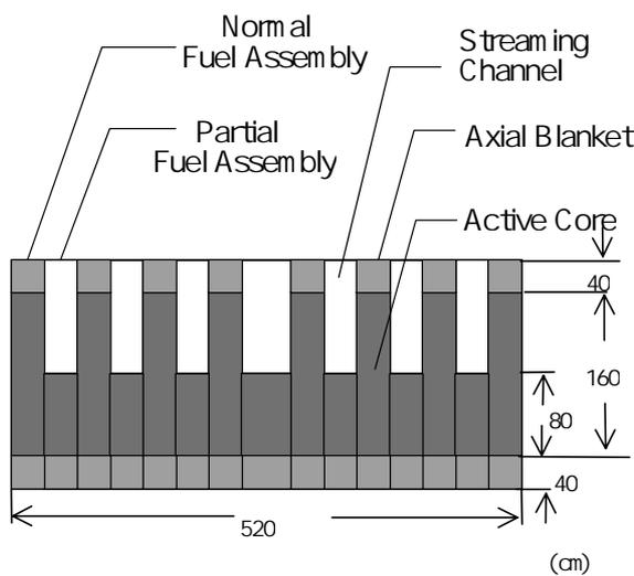
Fig. 2 Vertical View of BARS Core
