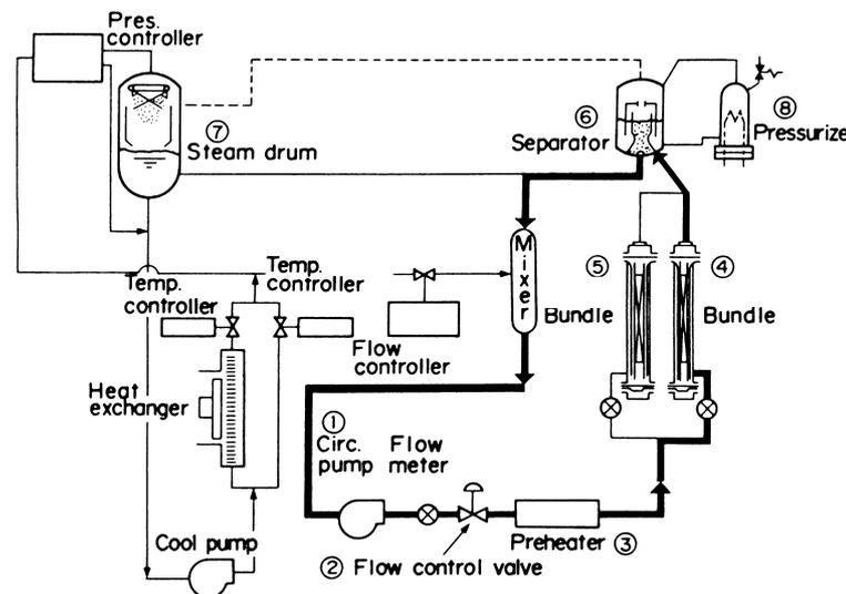
Fig. 10 Flow Diagram of Test Facility (BEST)
