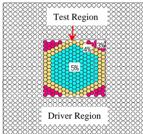
Fig. 7 One of the fuel rod arrangements of test core
