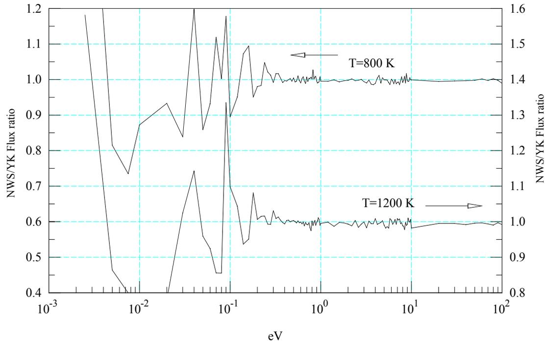
**Figure 2: Ratio of the neutron flux spectra inside fuel kernels computed with the NWS  $S(\alpha, \beta, T)$  and the YK  $S(\alpha, \beta, T)$  at the temperatures of 800 and 1200K.**
