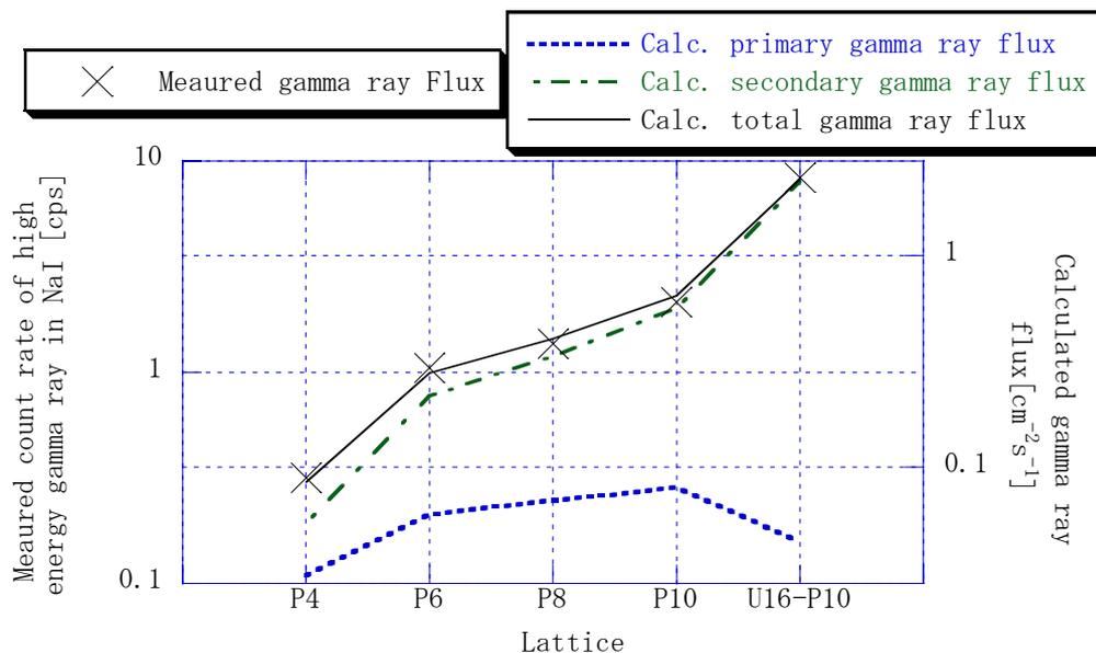
Figure 4. Comparison of the calculated high energy gamma ray flux to the measured count rate on the NaI(Tl) counter.
