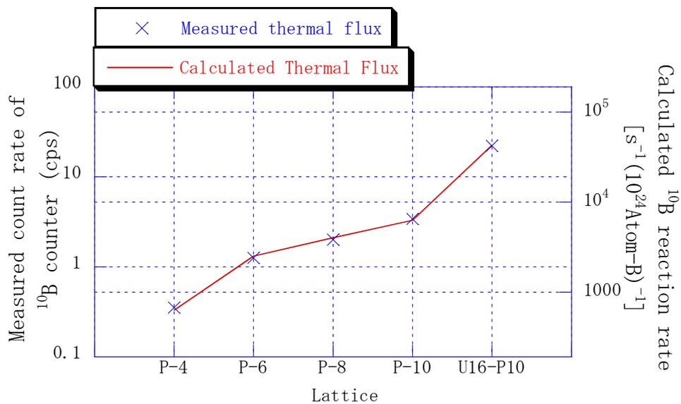
Figure 2. Comparison of calculated  $^{10}\text{B}(n,\alpha)$  reaction rate in surrounding water region with the count rate of  $^{10}\text{B}$  proportional counter.
