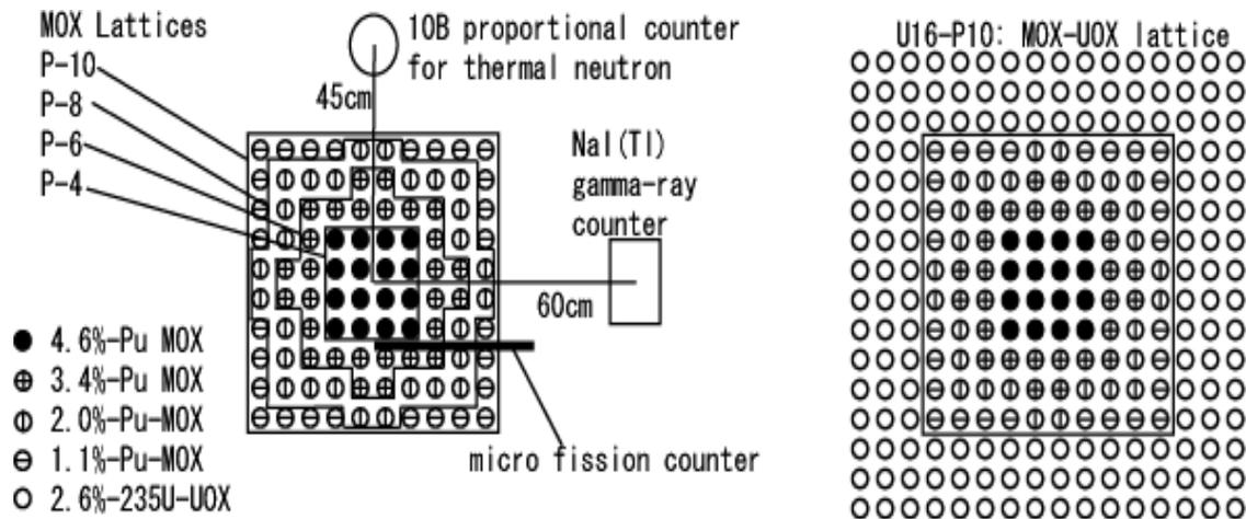
Figure 1. Horizontal schematic view of 5 types of subcritical MOX lattices and counters.
