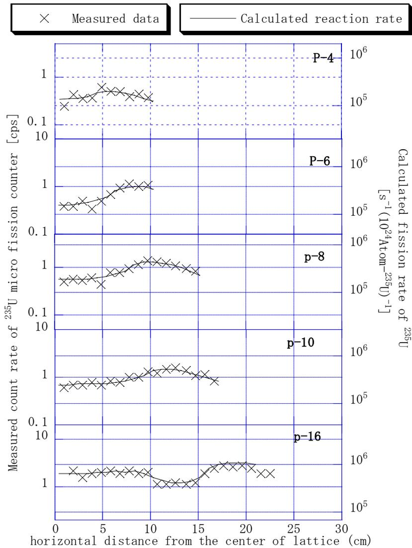
Figure 3. Comparison of calculated thermal flux distribution with the measured count rate of micro fission counter containing  $^{235}\text{U}$ .
