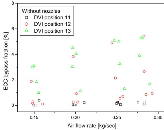
Figure 15. ECC water bypass by ECC water mixing according to DVI position
