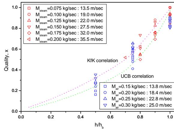
Figure 13. Amount of ECC water bypass by sweep-out from the present experiment with UCB and KfK correlations
