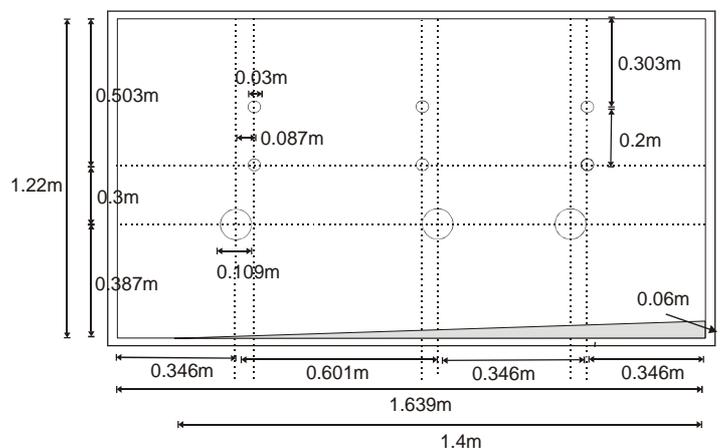
Figure 1. Schematic of test section
