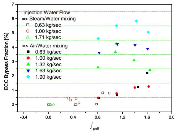
Figure 19. ECC water bypass fraction with air and steam injection
