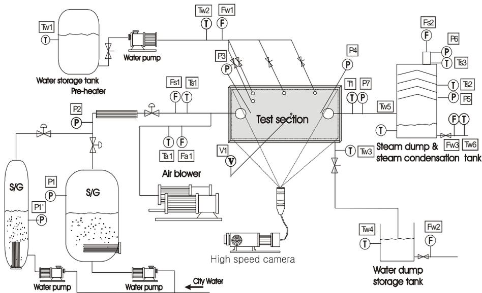
Figure 3. Schematic of experimental facility
