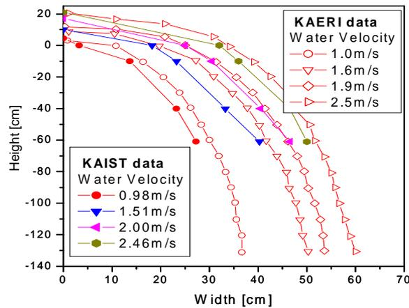
Figure 6. Comparison with results from KAERI experiment with the 1/7 scaled annulus downcomer
