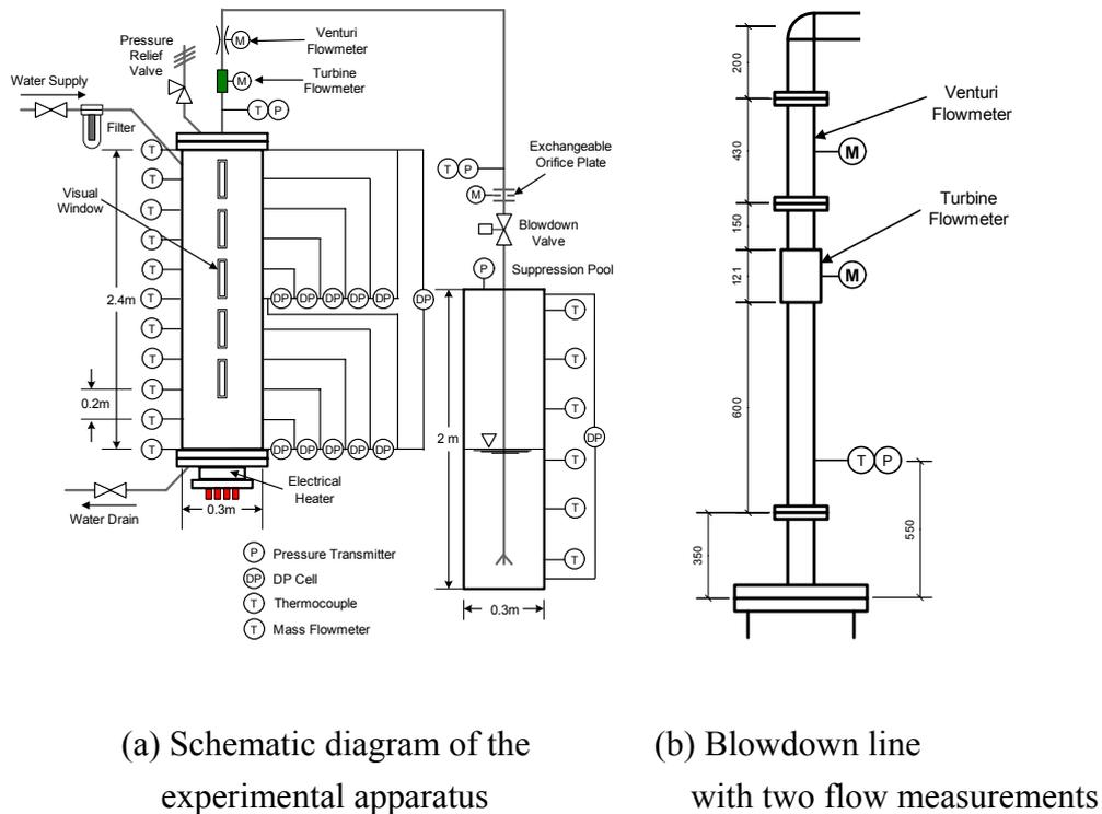
Figure 1. Depressurization and level-swell experimental apparatus.
