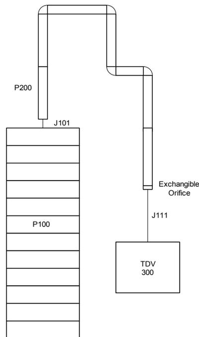
Figure 2. Nodalization of the present experimental apparatus.
