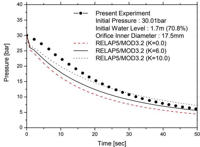
Figure 5. Pressure transient in the test vessel for case II.
