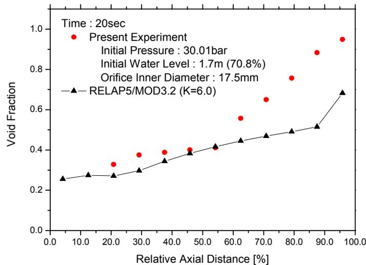
Figure 7. Axial void fraction distribution at the time of 20sec after the initiation of depressurization.
