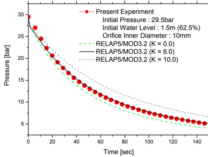
(a) Pressure transient in the test vessel
