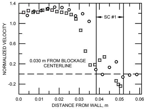
Figure 7. Axial velocity at 0.03 m downstream of blockage centerline.
