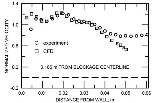
Figure 10. Axial velocity at 0.185 m downstream of blockage centerline.
