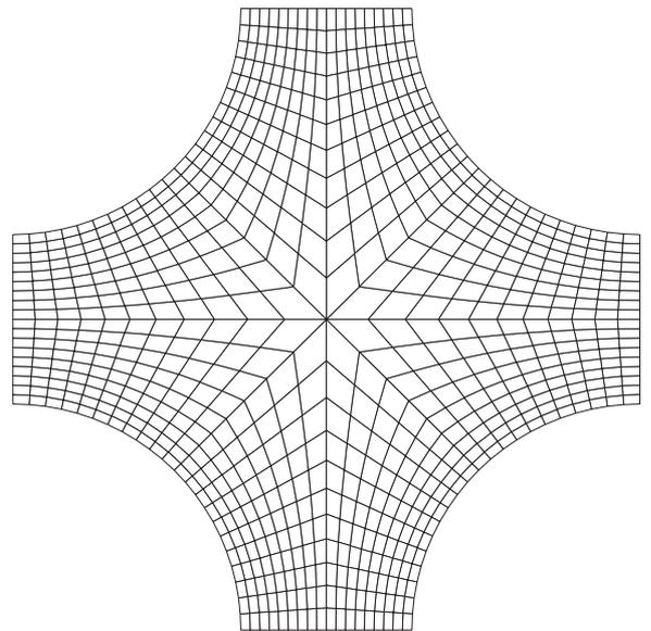
Figure 13. Flow-channel cross section (RNG grid)
