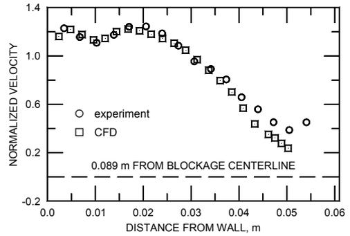
Figure 9. Axial velocity at 0.089 m downstream of blockage centerline.
