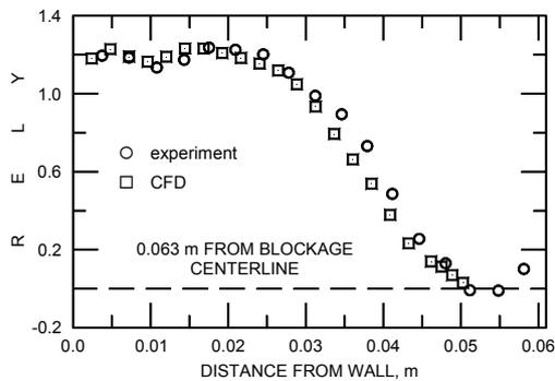
Figure 8. Axial velocity at 0.063 m downstream of blockage centerline.
