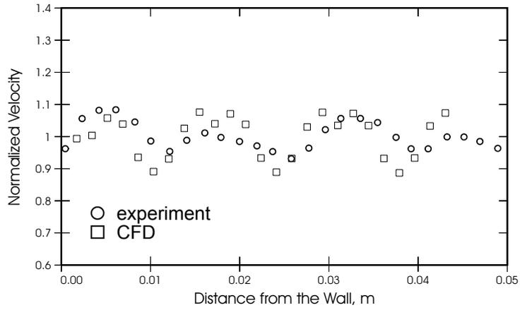
Figure 3. Axial velocity at 0.309 m downstream of spacer
