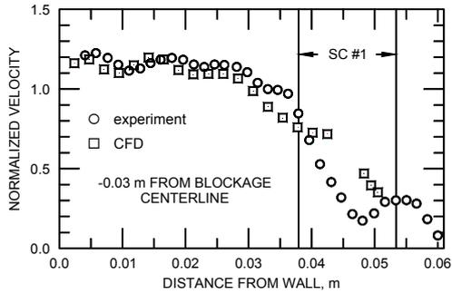
Figure 6. Axial velocity at 0.03 m upstream of blockage centerline.
