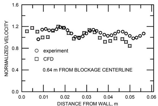
Figure 11. Axial velocity at 0.64 m downstream of blockage centerline.
