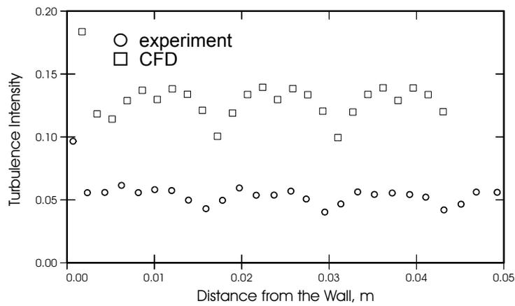
Figure 5. Axial turbulence intensity at 0.309 m downstream of spacer
