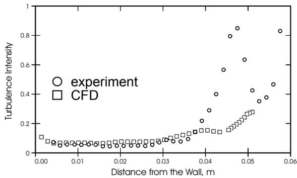
Figure 12. Axial turbulence intensity at 0.03 m upstream of blockage centerline
