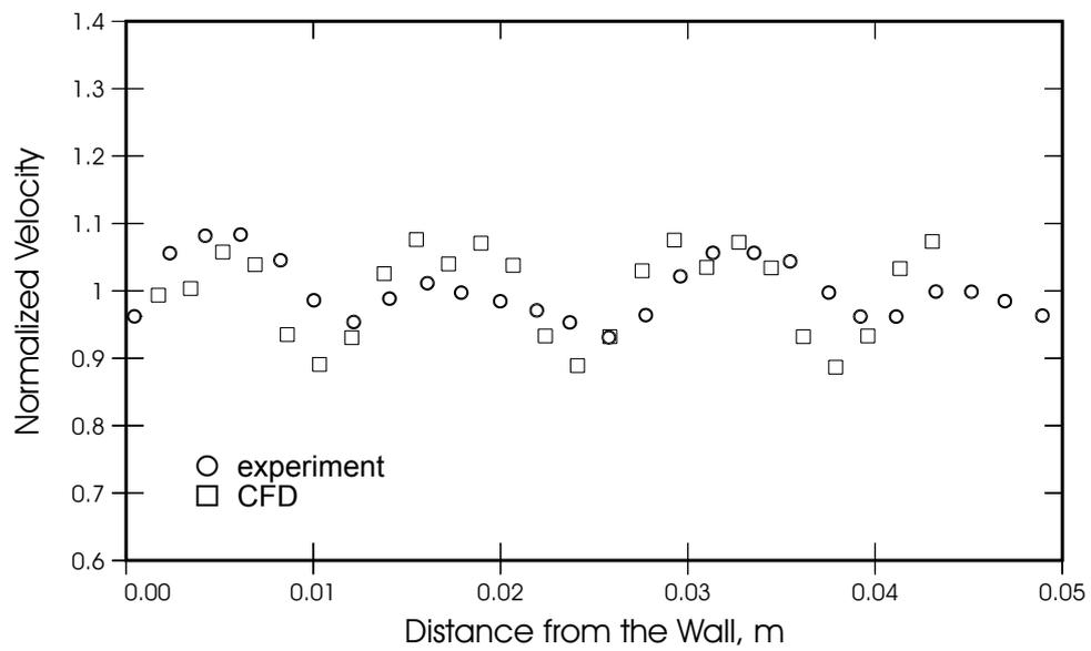
Figure 2. Axial velocity at 0.017 m downstream of spacer
