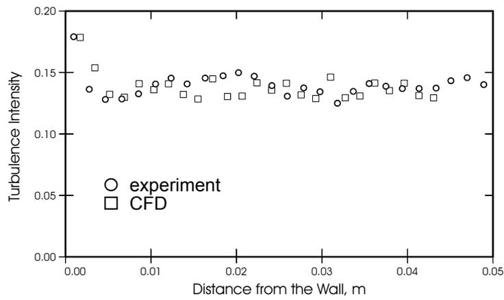
Figure 4. Axial turbulence intensity at 0.017 m downstream of spacer
