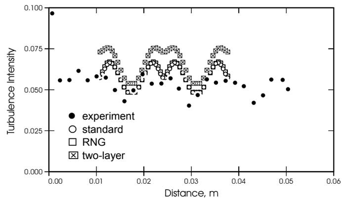
Figure 15. Axial turbulence intensity (k- $\epsilon$  models vs experiment)
