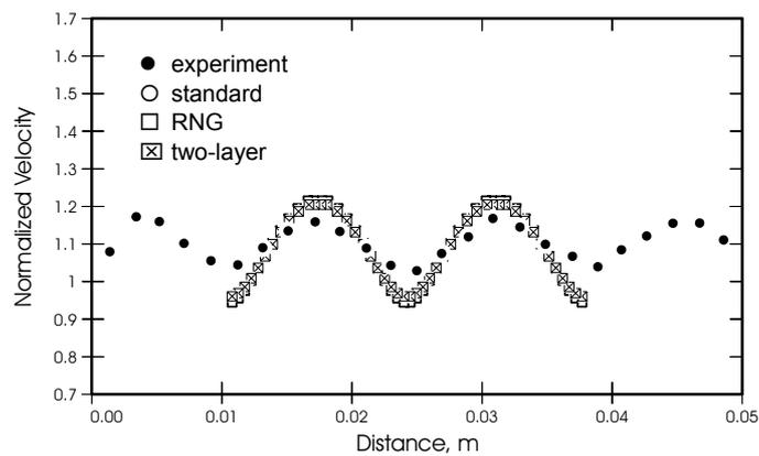
Figure 14. Axial velocity (k- $\epsilon$  models vs experiment)
