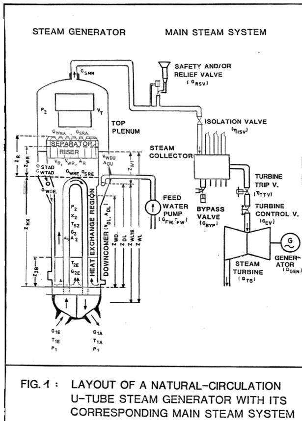
valves), all the lines ending in a steam collector (SC) with steam lines to the bypass and steam turbine system (bypass, turbine-trip and turbine control valves).
