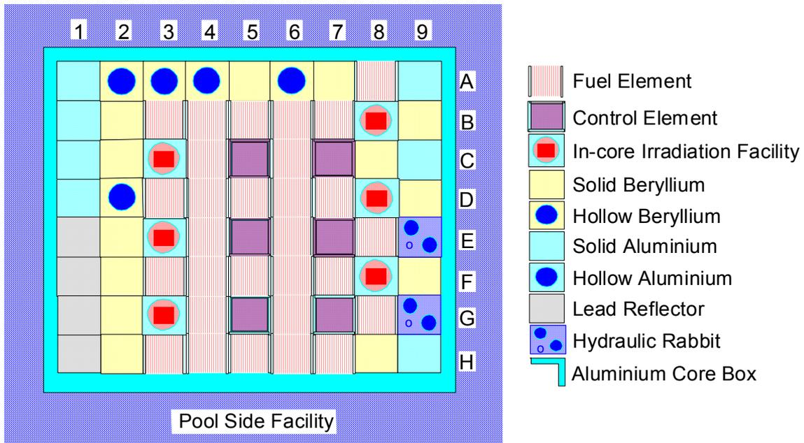
Figure 1. SAFARI-1 core layout for cycle 9907/1.
