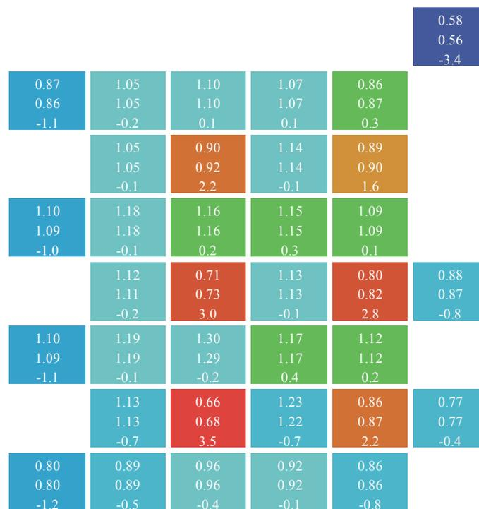
Figure 2. Relative power distribution and differences with re-homogenization applied EOC 9907/1.
