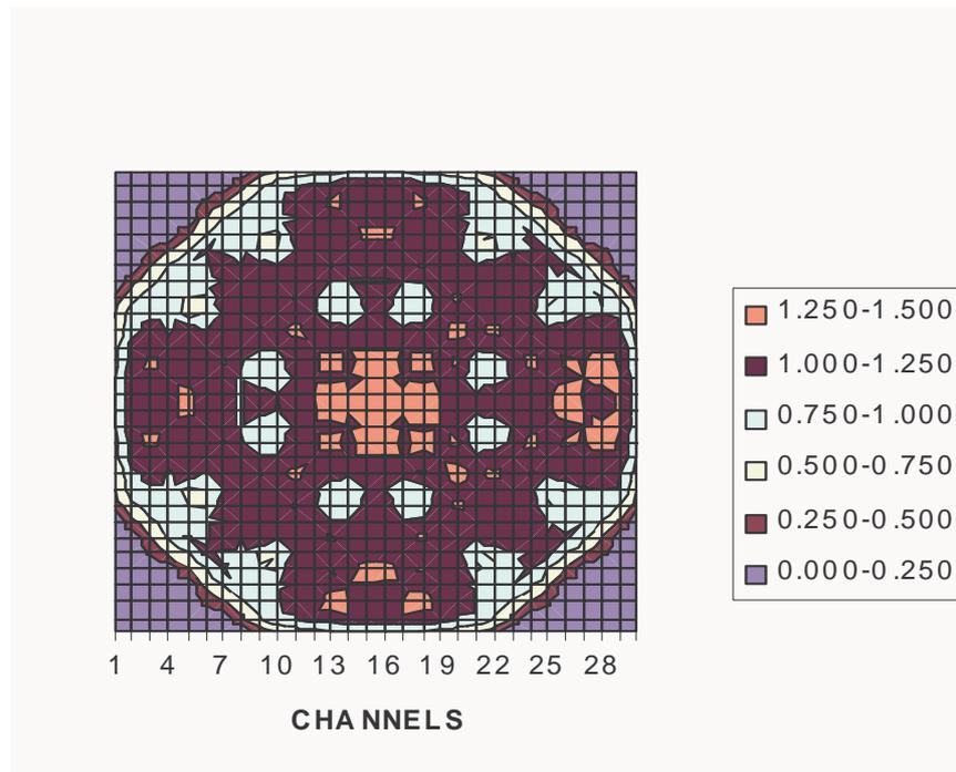
Figure 7. Two-dimensional normalized power distribution for initial steady state
