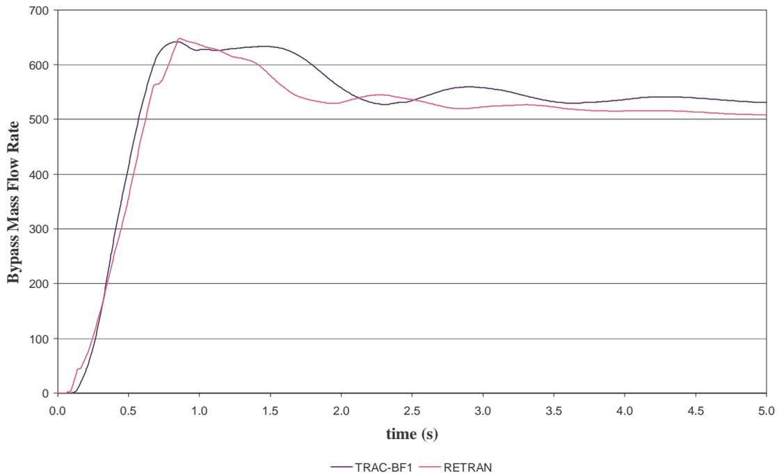
Figure 3. Bypass Mass Flow Rate Predictions for First Benchmark Exercise
