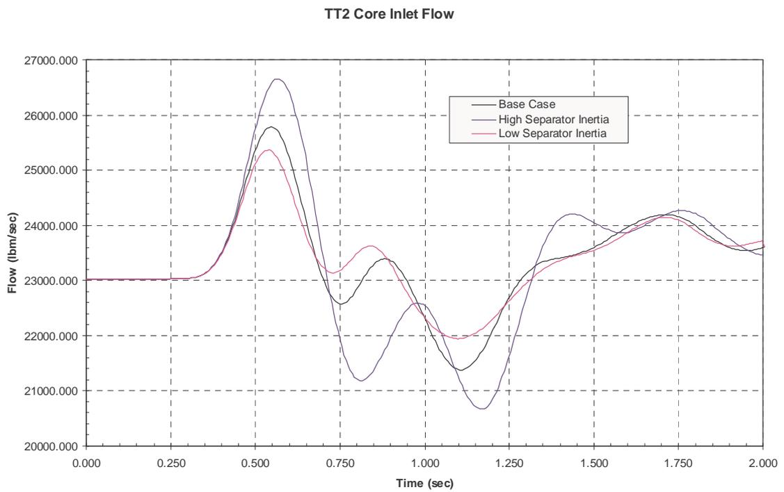
Figure 10. Time Evolution of Core Inlet Flow Response for Different Cases
