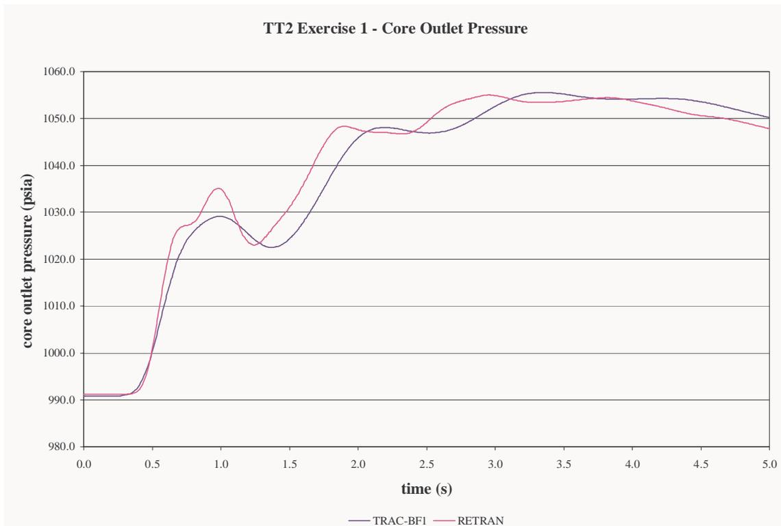
Figure 4. Core Exit Pressure Predictions for the First Benchmark Exercise
