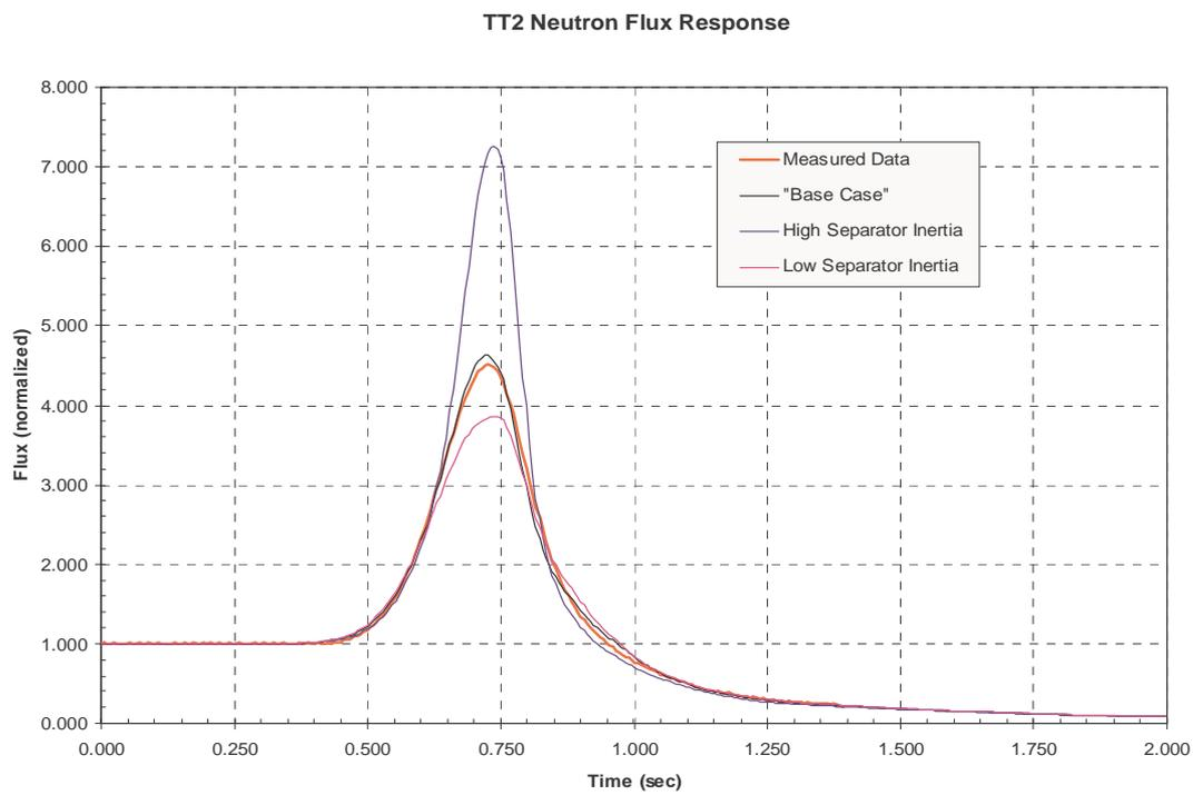
Figure 12. Time Evolution of Neutron Flux Response for Different Cases
