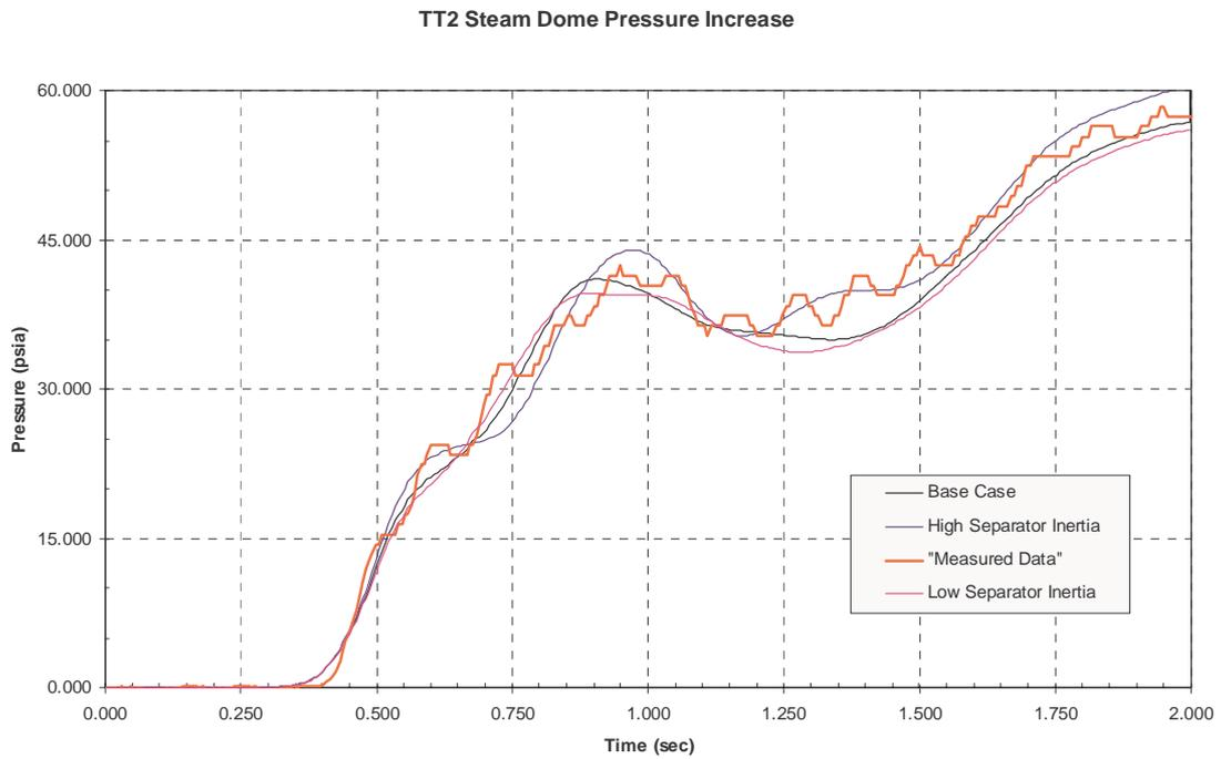
Figure 9. Time Evolution of Steam Dome Pressure Response for Different Cases
