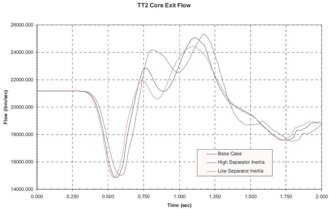
Figure 11. Time Evolution of Core Exit Flow Response for Different Cases
