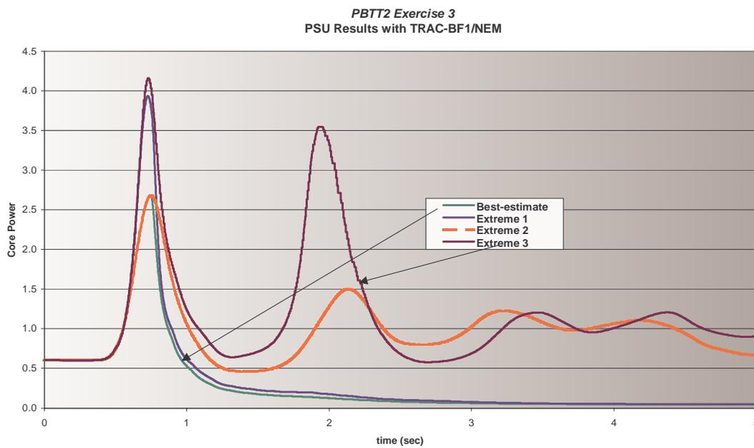
Figure 8. Relative core power response time evolution for different benchmark scenarios
