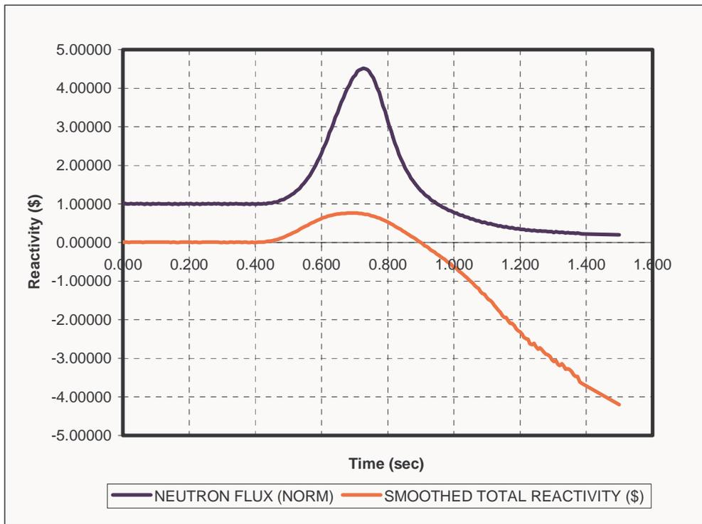
Figure 1. Neutron Flux and Reactivity Time Evolution for PB2 TT2
