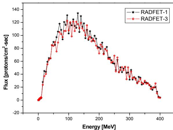
Figure 8. Calculated fluxes at two locations by MCNP-X detailed model
