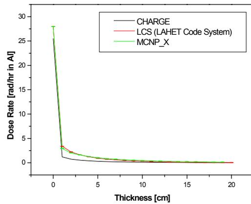
Fig 6. Proton spectrum of KITSAT-1 orbit at SAA location Fig 7. Dose-depth curves for aluminum from SAA spectrum environment
