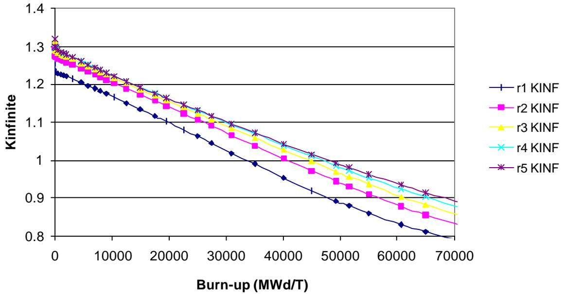
Figure 6. K-infinite vs burn-up for different seed rod dimensions. (r1=0.33cm, r2=0.4cm, r3=0.45cm, r4=0.5cm, r5=0.55cm)
