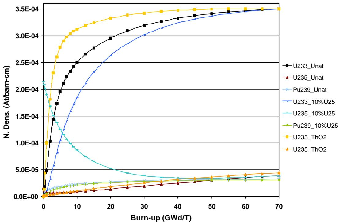
Figure 4. Main fissile isotopes evolution in the blanket sub-lattice
