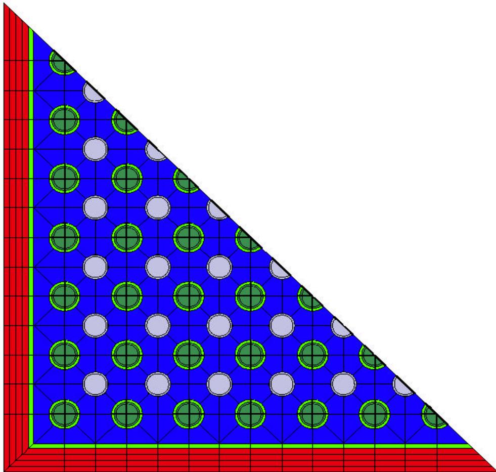
Figure 3. Blanket-seed lattice (diagonal symmetry).
