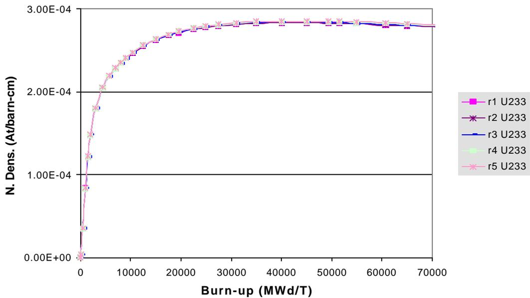
Figure 5. U-233 build-up for different dummy rod dimensions.
