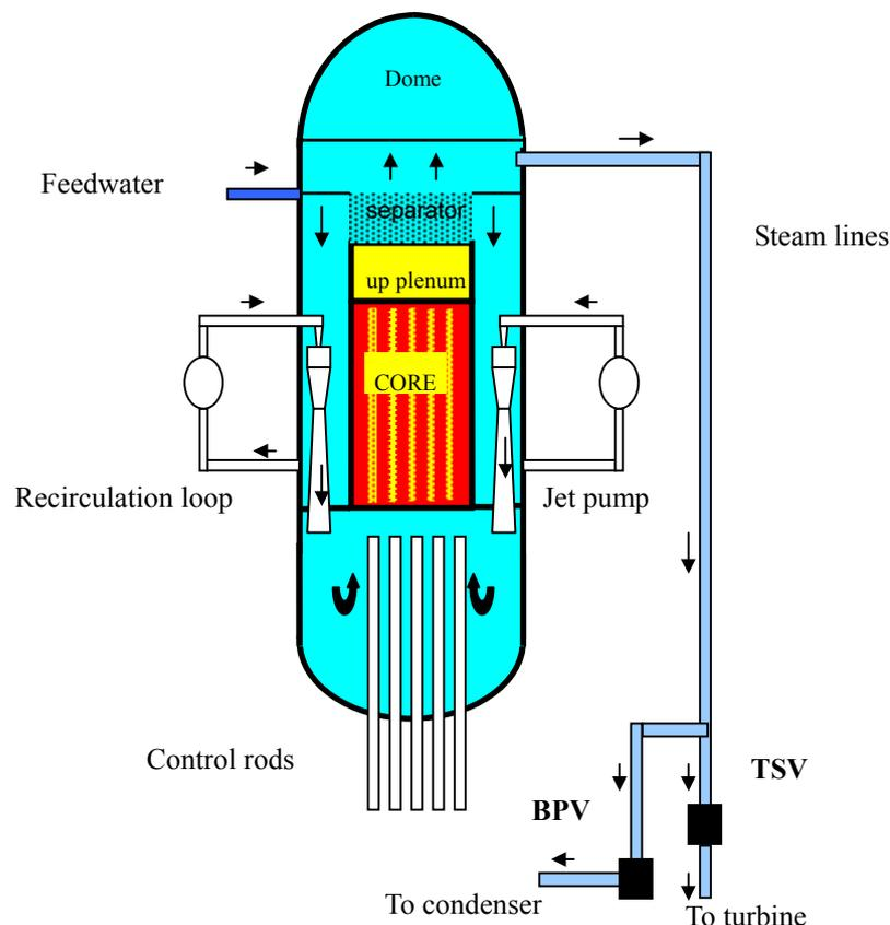
Figure 1. Peach Bottom reactor model
