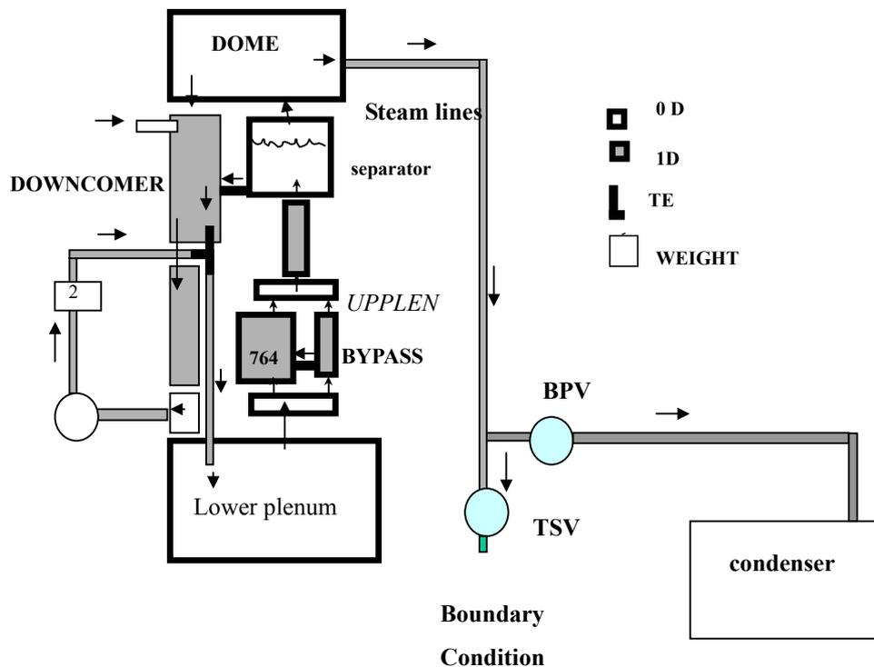
Figure 2. CATHARE modeling of the PB2 reactor
