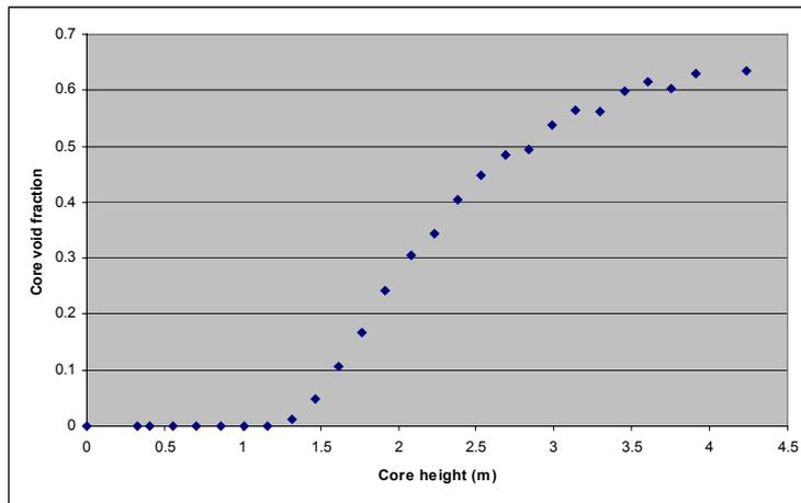
Figure 3. Axial distribution of core void fraction
