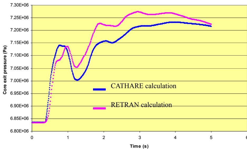
Figure 6. Core exit pressure evolution
