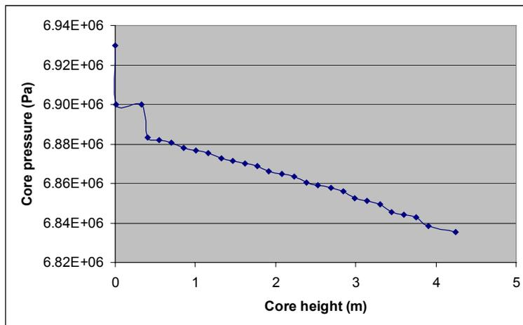
Figure 4. Core pressure drop
