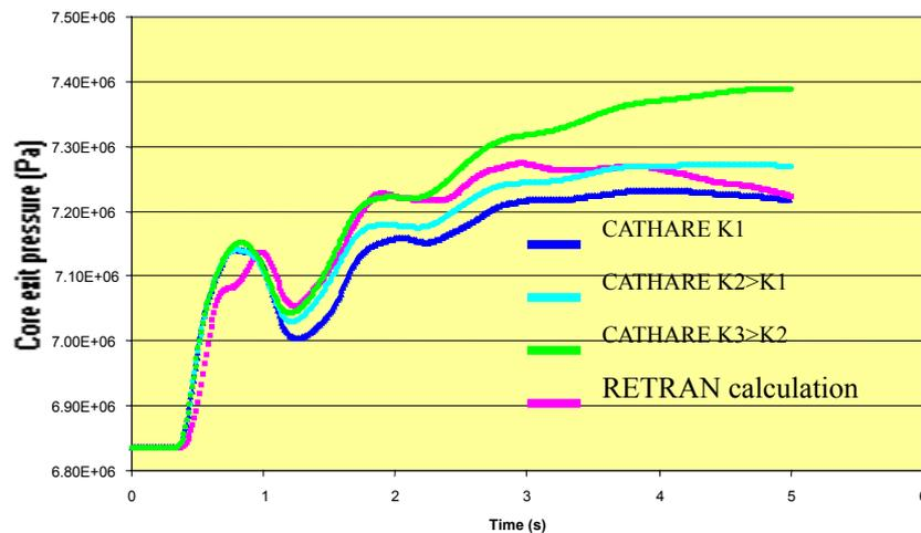
Figure 8. Core exit pressure. Sensitivity to the BPV coefficient
