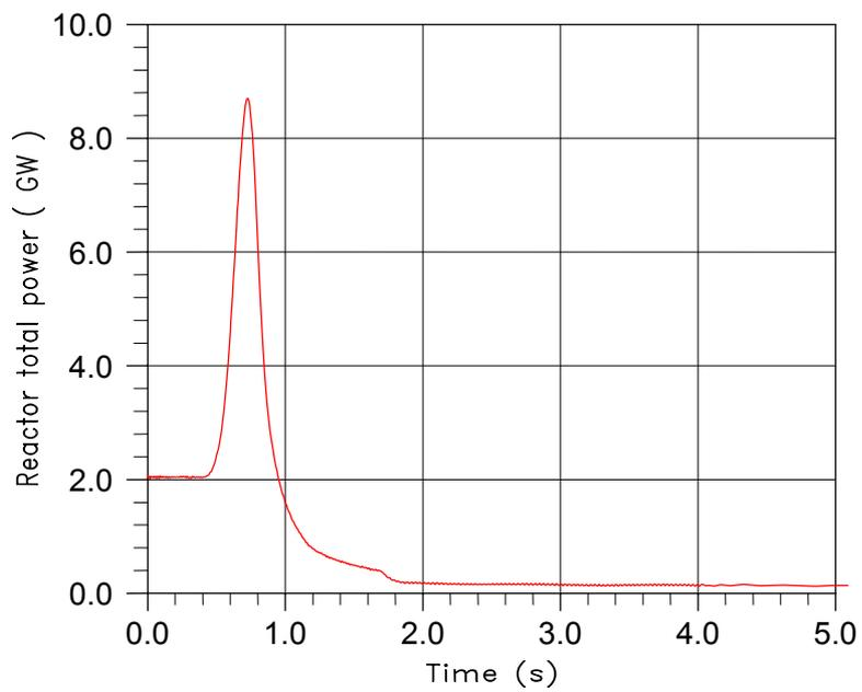
**Figure 3.** Total reactor power specified in the Benchmark for Exercise 1
