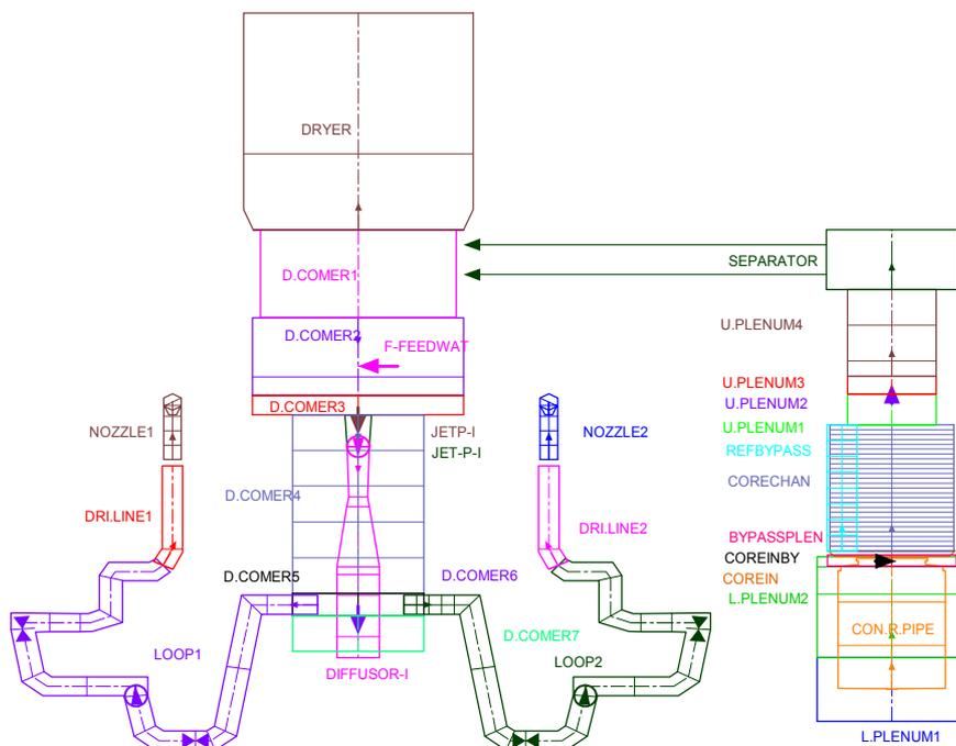
**Figure 1.** ATHLET nodalization of the reactor vessel and the recirculation loops
