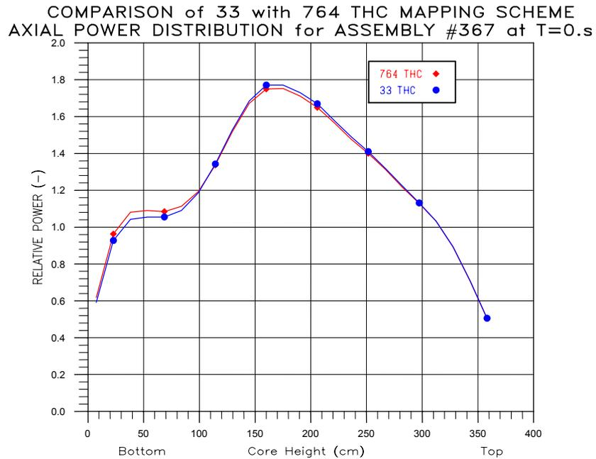
**Figure 11.** Comparison of axial power distributions in the initial steady state for fuel assembly #367 using 33 THC and 764 THC in the ATHLET-QUABOX/CUBBOX calculations
