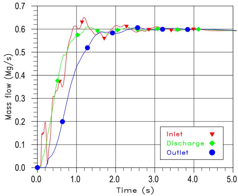
**Figure 8.** Mass flow rate in the bypass line at the inlet from the steam line, at the outlet and the discharge flow
