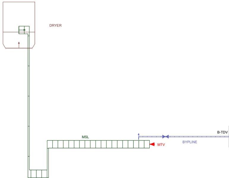
**Figure 2.** ATHLET nodalization of the steam line and the bypass line
