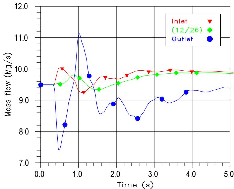
**Figure 5.** Mass flow rate in the reactor core at inlet, at outlet and at an intermediate location
