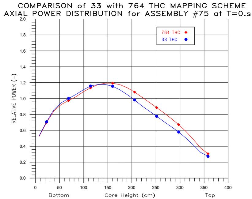
**Figure 10.** Comparison of axial power distributions in the initial steady state for fuel assembly #75 using 33 THC and 764 THC in the ATHLET-QUABOX/CUBBOX calculations
