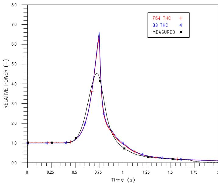
**Figure 9.** Relative power histories for Exercise 2 calculated by ATHLET-QUABOX/CUBBOX using 33 THC and 764 THC compared to measured data
