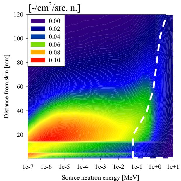
Figure 5. Recoil protons produced by hydrogen (dashed line explained in the text).
