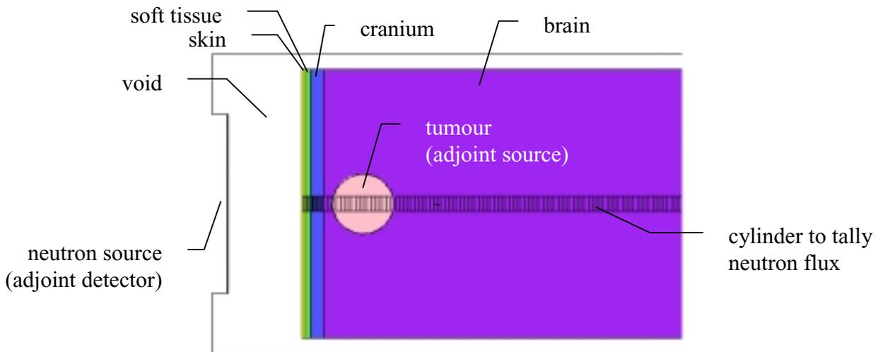
Figure 1. Cross-section of MCNP slab geometry.
