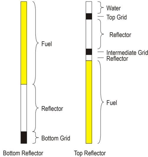
Figure 2. Schematic of the axial reflector configuration.
