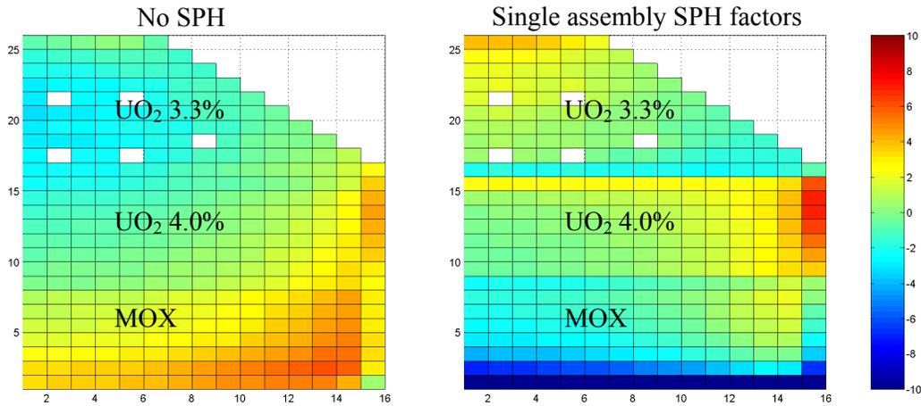
Figure 5. Pin power relative percent error for 8 group, SP<sub>3</sub> solution.
