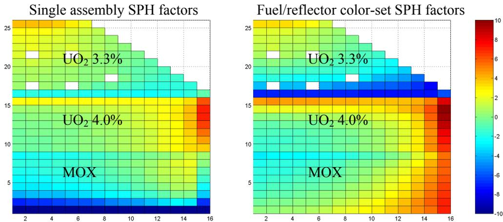
Figure 6. Pin power relative percent error for 8 group, SP<sub>3</sub> solution.
