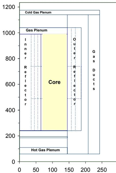
Fig 1. Sketch of the ACACIA model with annular core.
