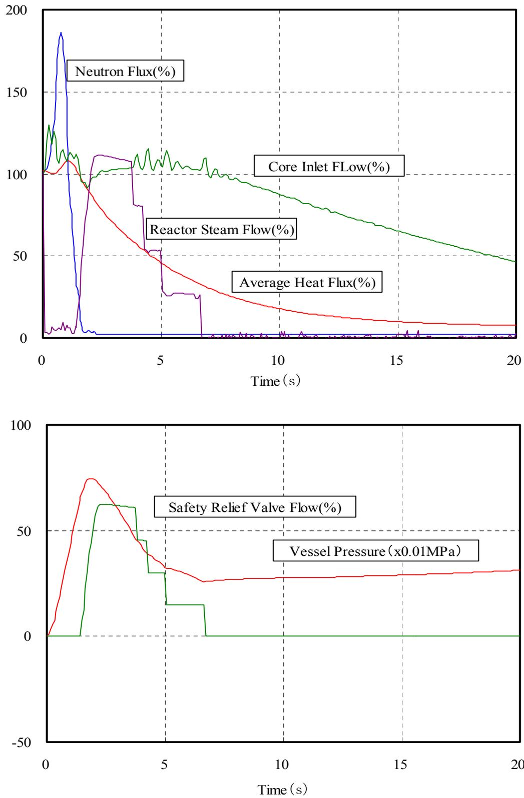
Figure 11. Generator Load Rejection with turbine bypass valve failure
