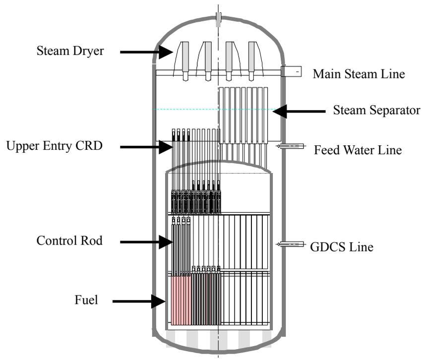
Figure 1. Schematic vertical view of reactor vessel
