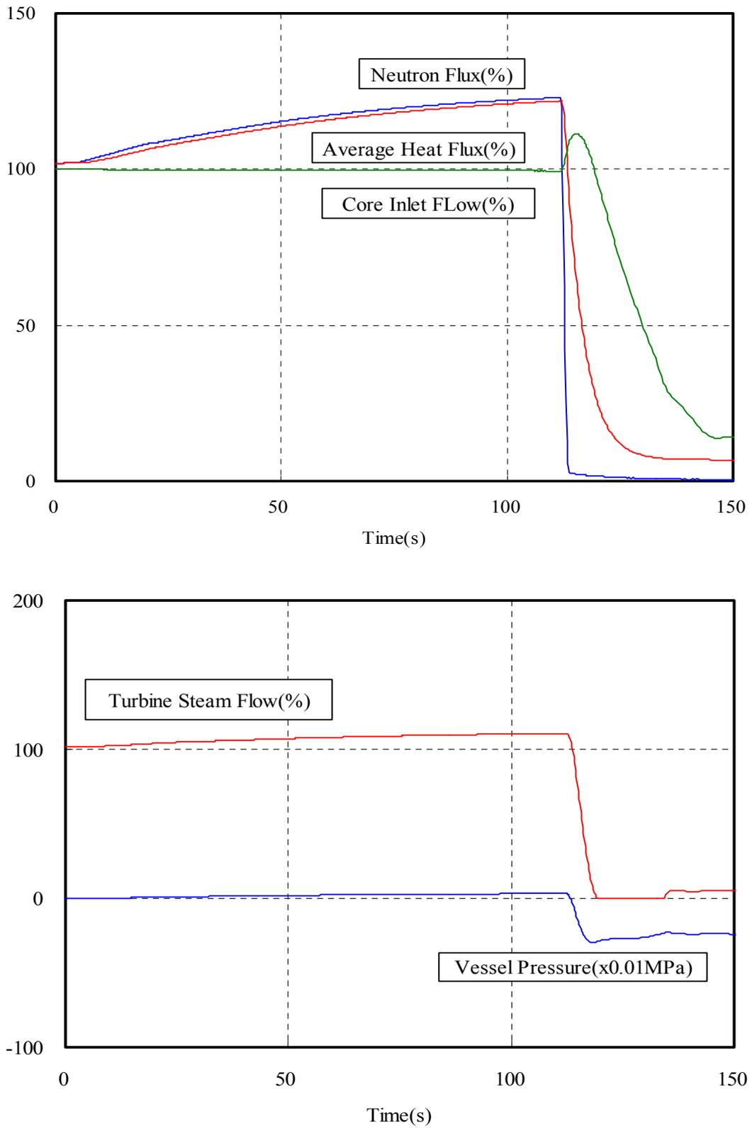
Figure 10. Loss of feedwater heating
