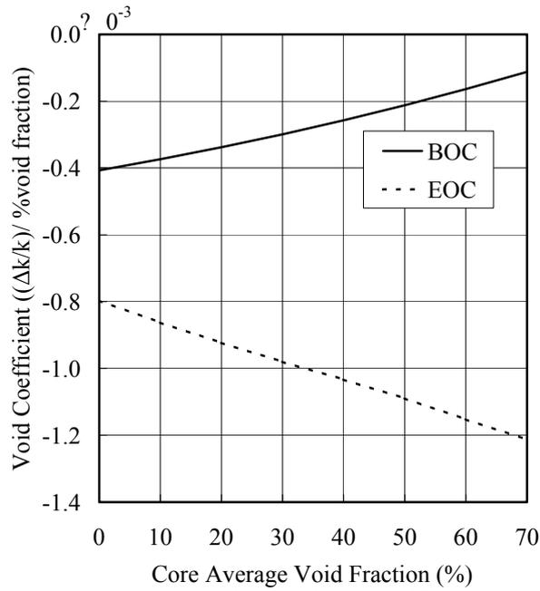
Figure 8. Void reactivity coefficient
