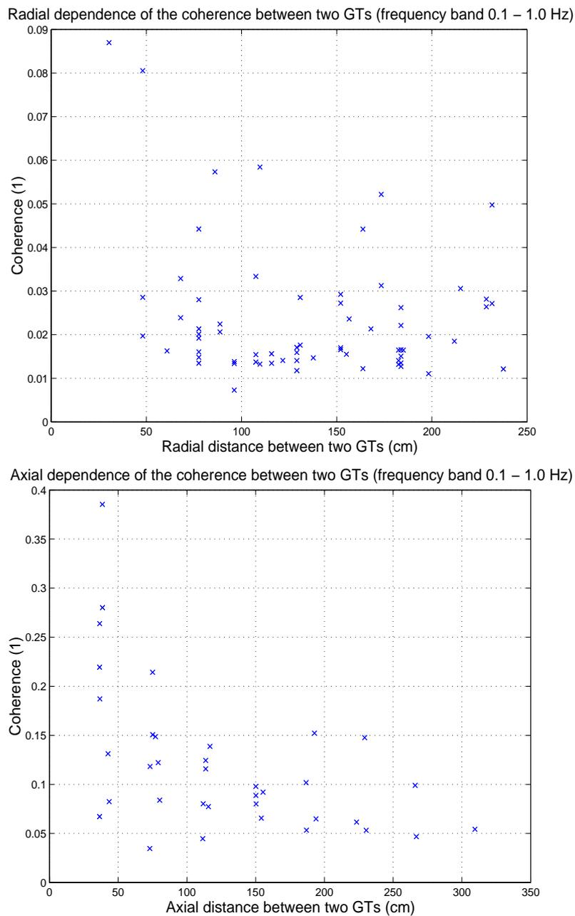
Figure 5. Dependence of the coherence between two GTs with their separation distance in the frequency band 0.1 - 1.0 Hz
