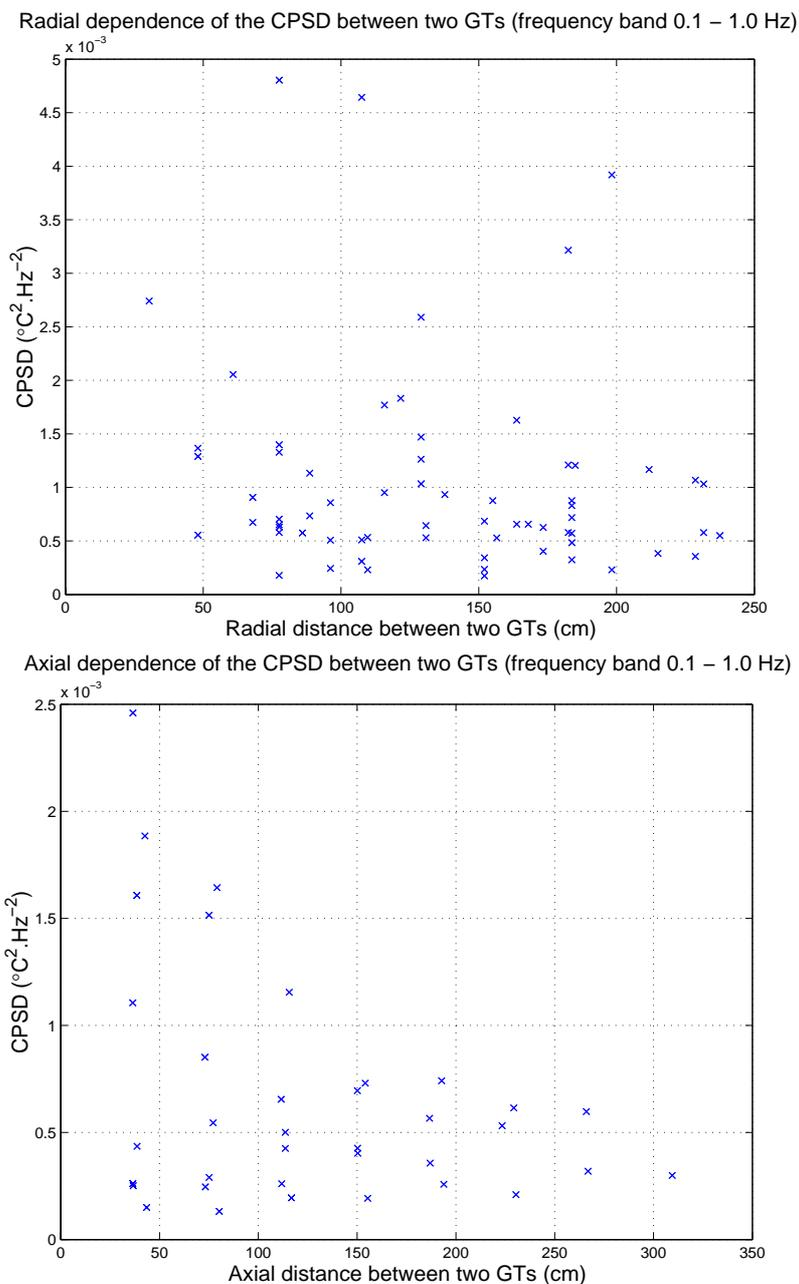
Figure 6. Dependence of the CPSD between two GTs with their separation distance in the frequency band 0.1 - 1.0 Hz
