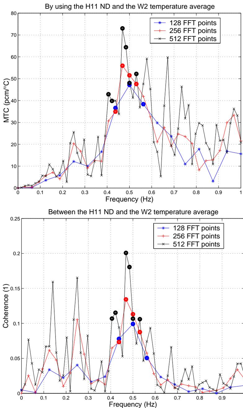
Figure 7. Frequency dependence of the MTC noise estimation with respect to the number of FFT points used (neutron noise measured in the H11 assembly and temperature noise evaluated by using W2)
