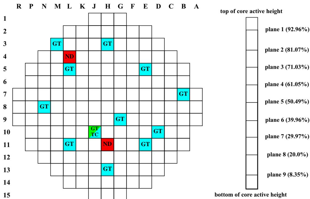
Figure 3. Position of the detectors for the noise measurement in Ringhals-2 on January 16<sup>th</sup>, 2002 (on the left hand side the radial position on the seventh axial plane; on the right hand side the axial position in the J10 fuel assembly))
