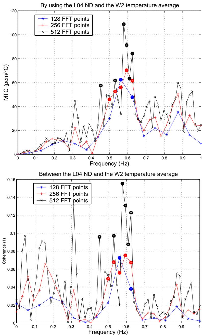
Figure 8. Frequency dependence of the MTC noise estimation with respect to the number of FFT points used (neutron noise measured in the L04 assembly and temperature noise evaluated by using W2)
