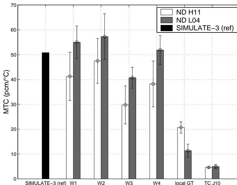
Figure 10. Comparison between the different MTC noise estimators (estimations carried out with 256 FFT points)
