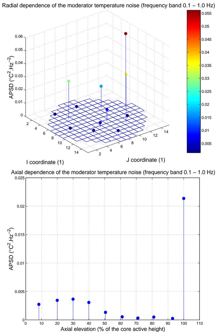
Figure 4. Spatial dependence of the APSD of the moderator temperature noise in the frequency band 0.1 - 1.0 Hz
