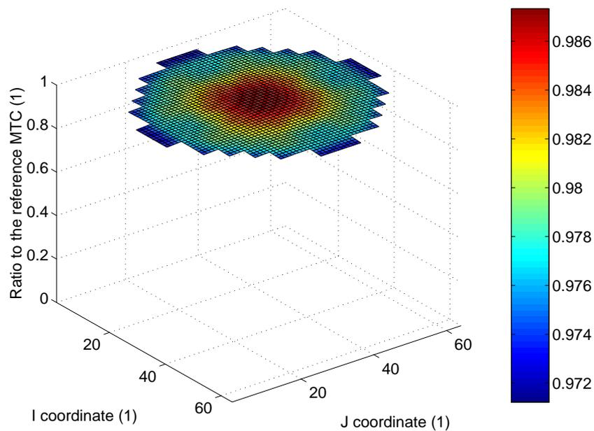
Figure 2. Ratio between the  $\tilde{H}_1^{biased}$  MTC noise estimator (i.e. the recently suggested one) and the actual value of the MTC
