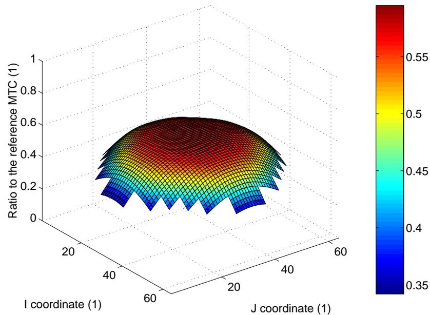
Figure 1. Ratio between the  $H_1^{biased}$  MTC noise estimator (i.e. the traditionally used one) and the actual value of the MTC
