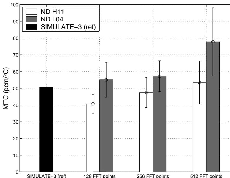
Figure 9. Comparison of the MTC noise evaluations with respect to the number of FFT points used (temperature noise evaluated by using W2)
