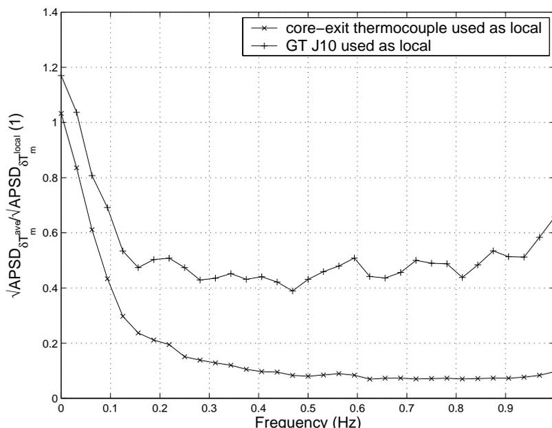
Figure 11. Comparison between the noise levels recorded by the core-exit thermocouple, a GT, and the planar average of all the GTs
