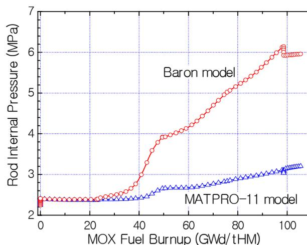
Figure 7 Rod internal pressure change with burn-up increase
