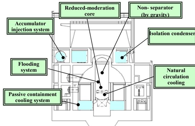
Figure 3 Plant system concept for hybrid design
