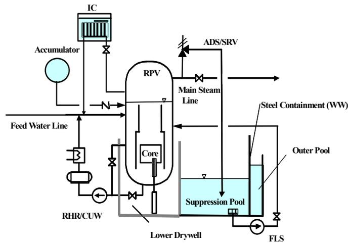
Figure 4 Concept of safety system
