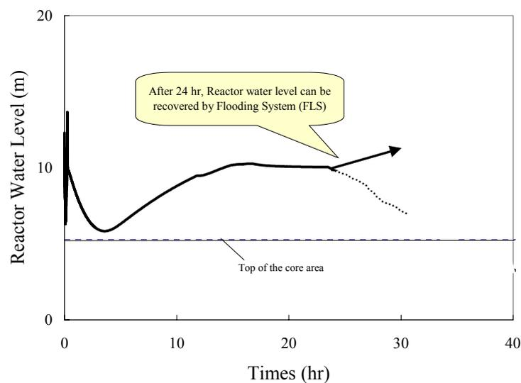
Figure 5 Analyzed water level during drain line break LOCA
