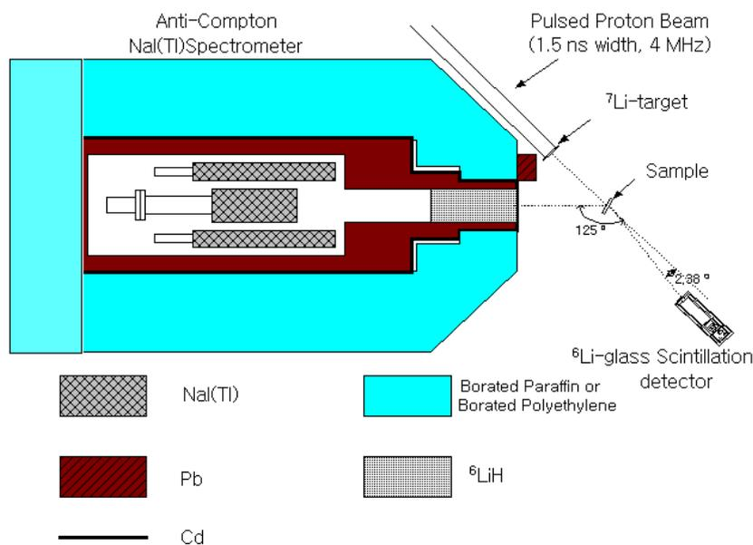
Figure 1. The experimental arrangement for cross section measurement
