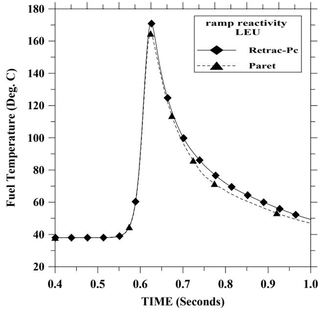
Figure 4 : Fuel Temperature transient
