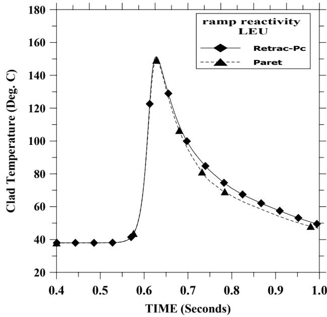
Figure 5: Clad Temperature transient
