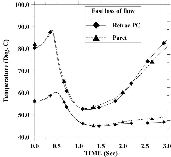
**Figure 8: Results of RETRAC-PC and PARET codes for fast loss of flow transient (LEU)**
