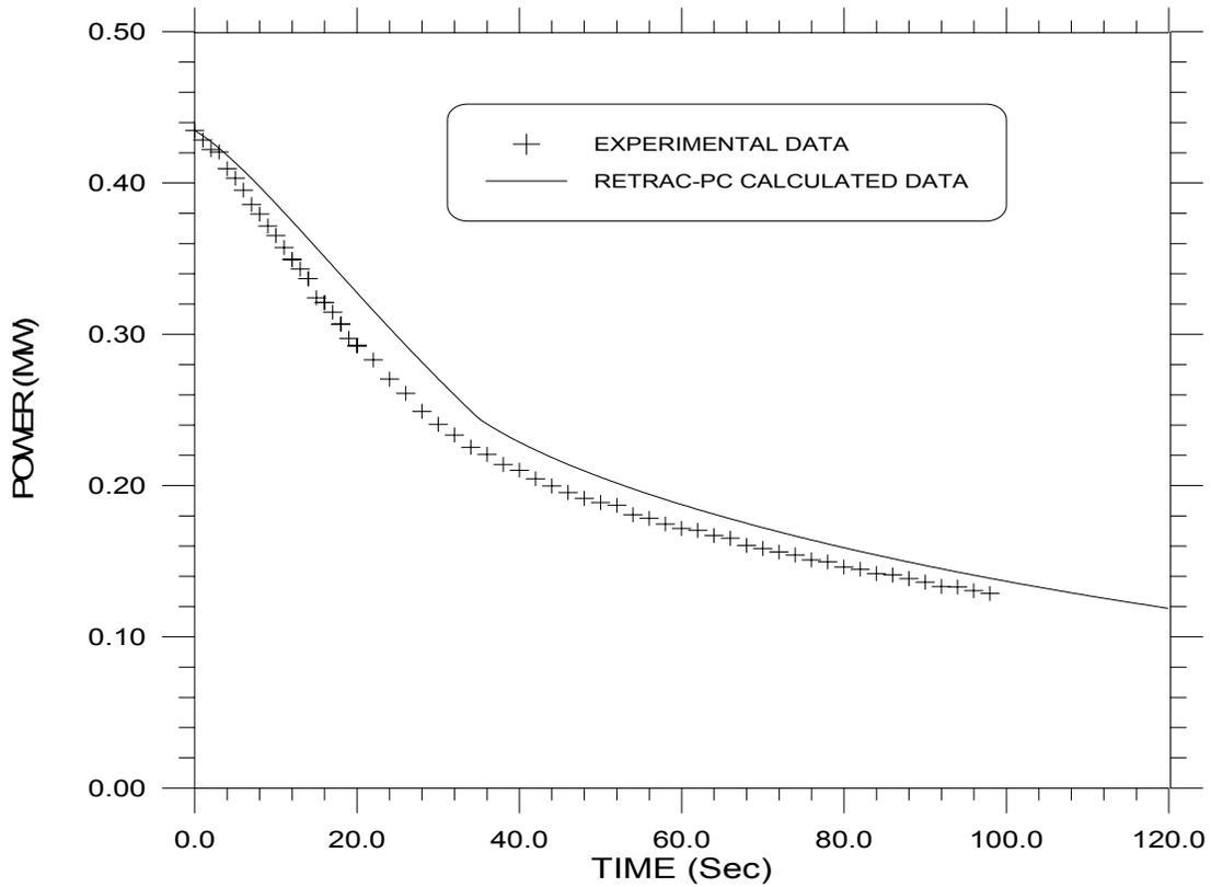
**Fig-2 Power Evolution during Control Rod Insertion Test**
