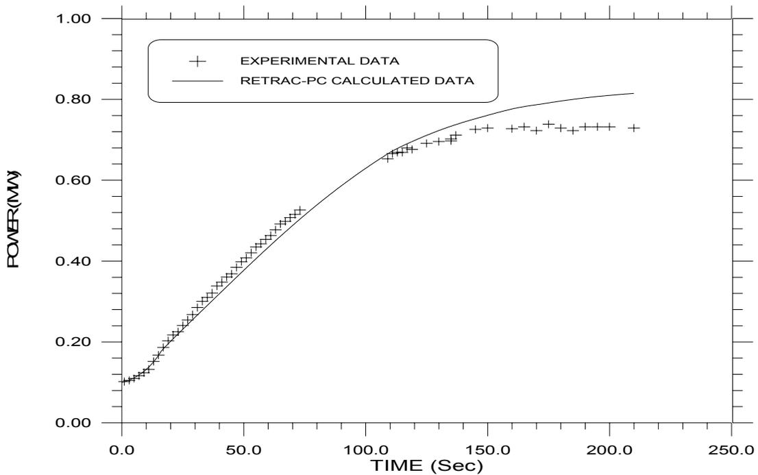
**Fig-1 Power Evolution during Control Rod Withdrawal Test**
