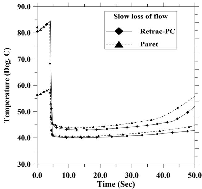
**Figure 7: Results of RETRAC-PC and PARET codes for slow loss of flow (LEU)**
