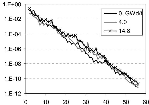
Figure 1. Convergence ratio: maximum nodal deviation versus iteration number (double precision), at the beginning, middle and end of the cycle.
