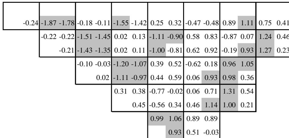
Figure. 2. Errors (%) in power distributions to 0. GWd/t, HFP, ARO, with both cross sections and interface flux discontinuity heterogeneity factors from assembly calculations.
