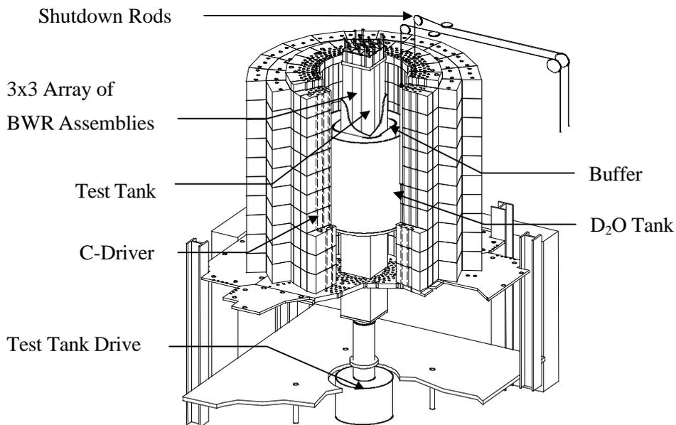
Figure 1. Cut-away view of the LWR-PROTEUS facility with indication of the main zones and components.
