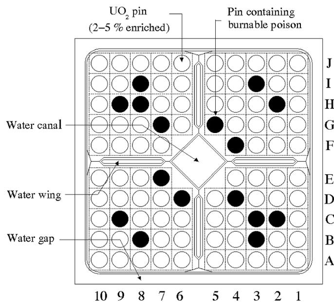
Figure 2. Westinghouse SVEA-96+ fuel assembly. Shaded areas correspond to the location of Gd-containing fuel pins in the upper assembly region.
