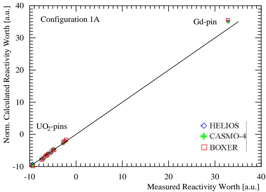
Figure 4. Calculated and measured LWR-PROTEUS reactivity worths for selected pins in the lower SVEA-96+ region.
