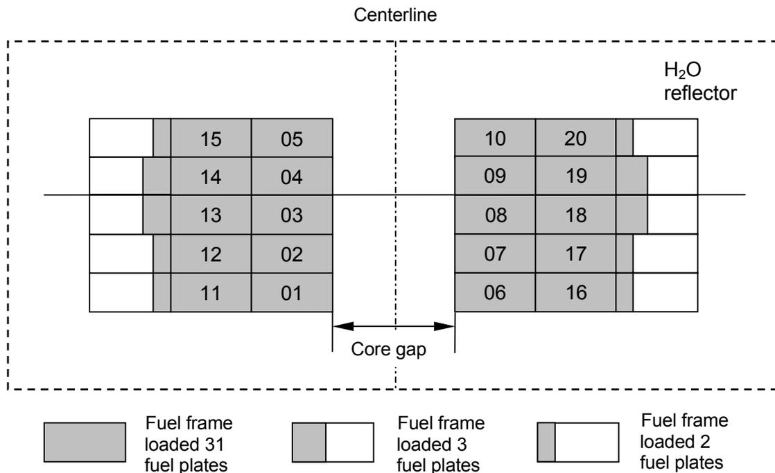
Fig. 1 Top view of investigated coupled-core configuration at the KUCA C-core.
