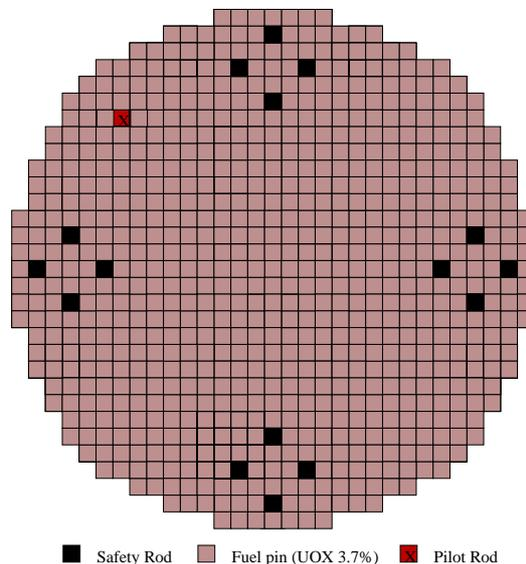
Figure 1. MISTRAL1 Homogeneous Core
