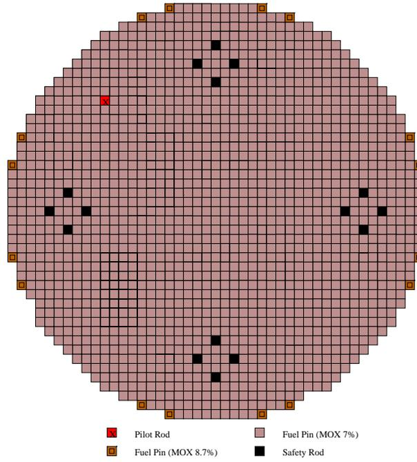
Figure 2. MISTRAL2 Homogeneous Core
