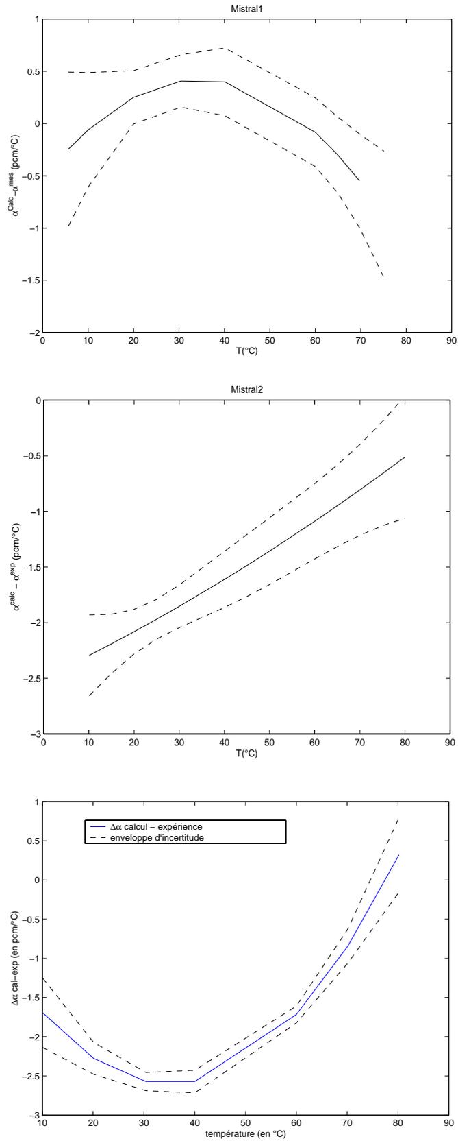
Figure 6. Calc-Exp Comparison of the RTC in MISTRAL1, 2 and 3 Experiments
