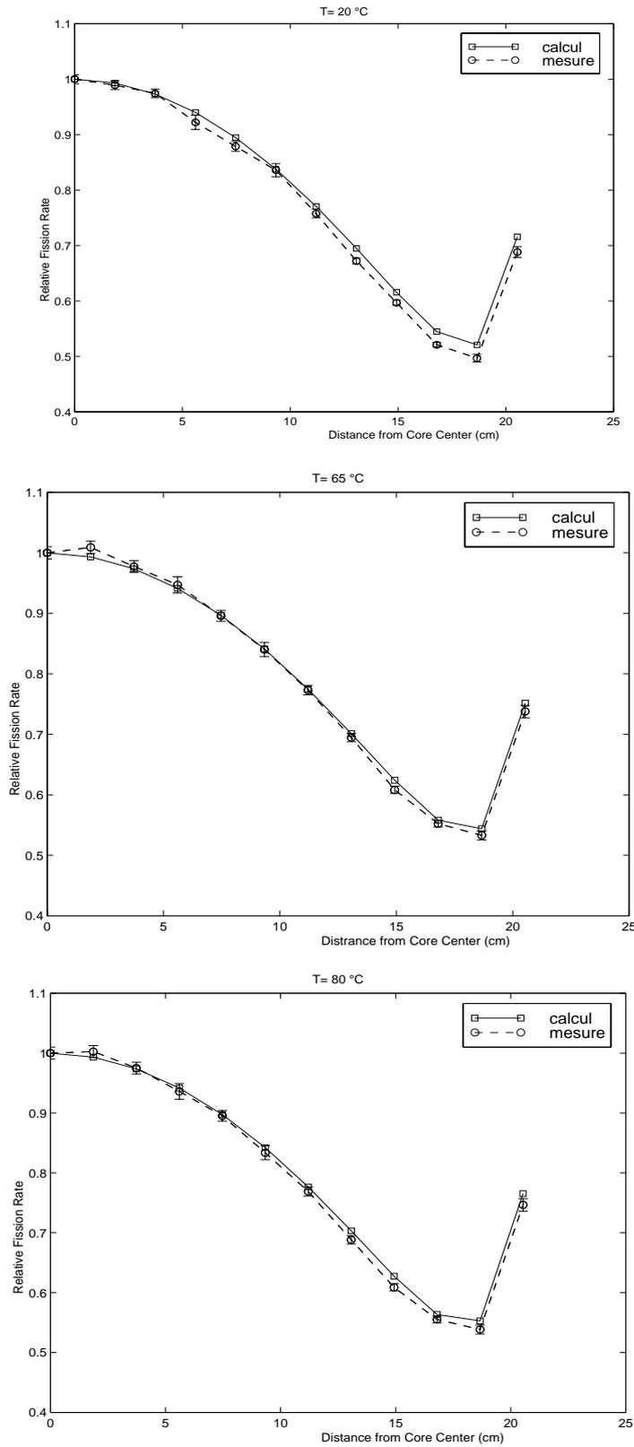
Figure 5. Radial Fission Rate in Mistral1 ( $T=20^\circ\text{C}$ ,  $T=65^\circ\text{C}$  and  $T=80^\circ\text{C}$ )
