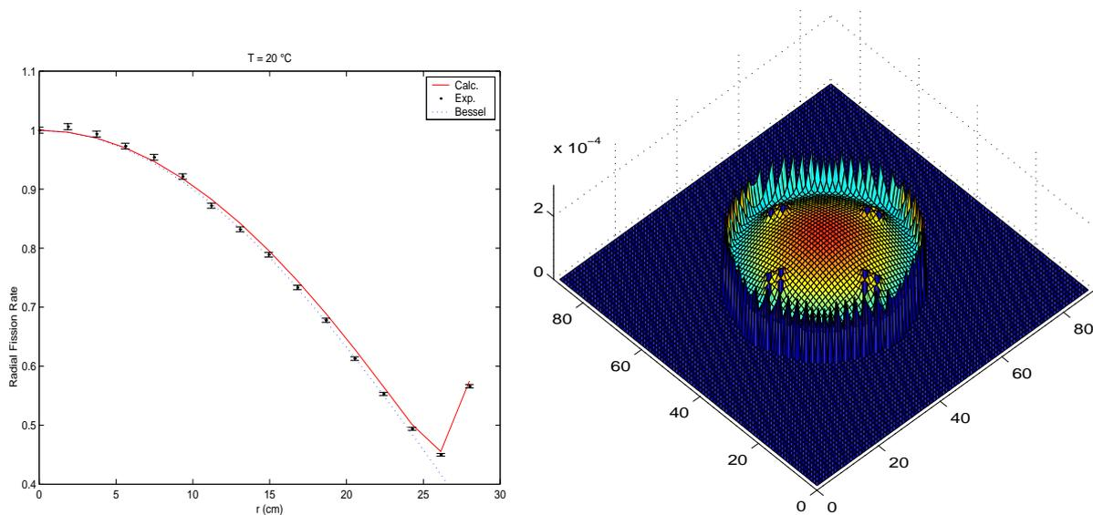
Figure 4. Radial Fission Rate in Mistral2
