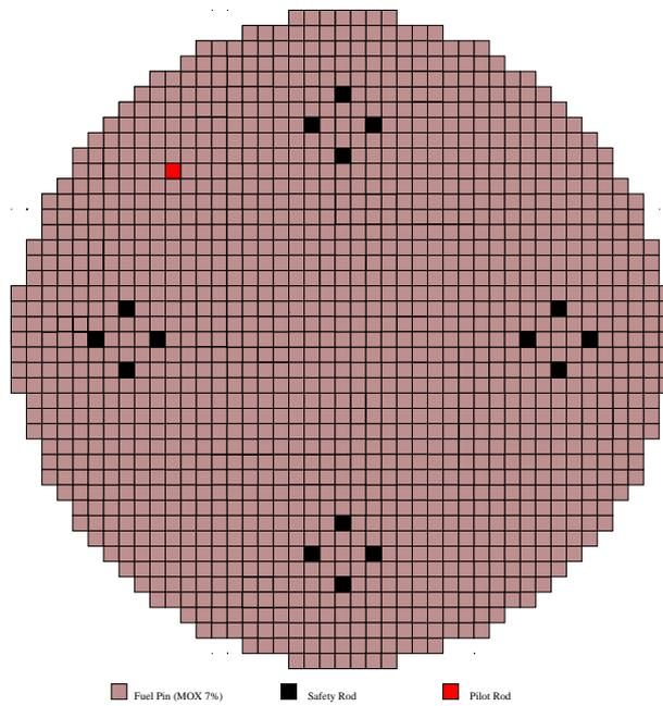
Figure 3. MISTRAL3 Homogeneous Core
