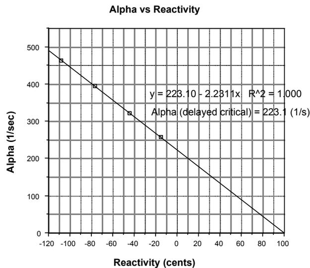
Figure 6. Rossi- $\alpha$  as a function of reactivity for  $^{235}\text{U}-\text{SiO}_2$ -polyethylene experiment.
