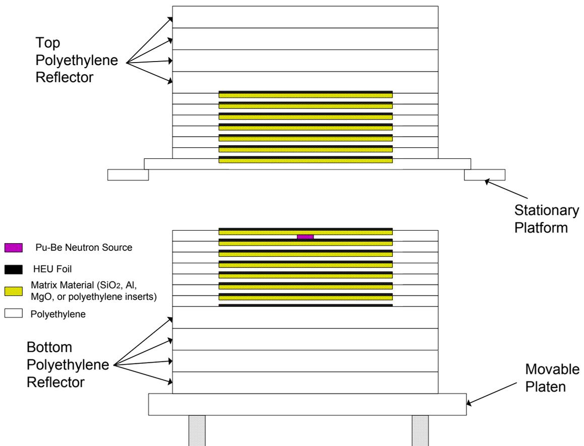
Figure 2. Approximate final configuration for the diluted HEU experiments.
