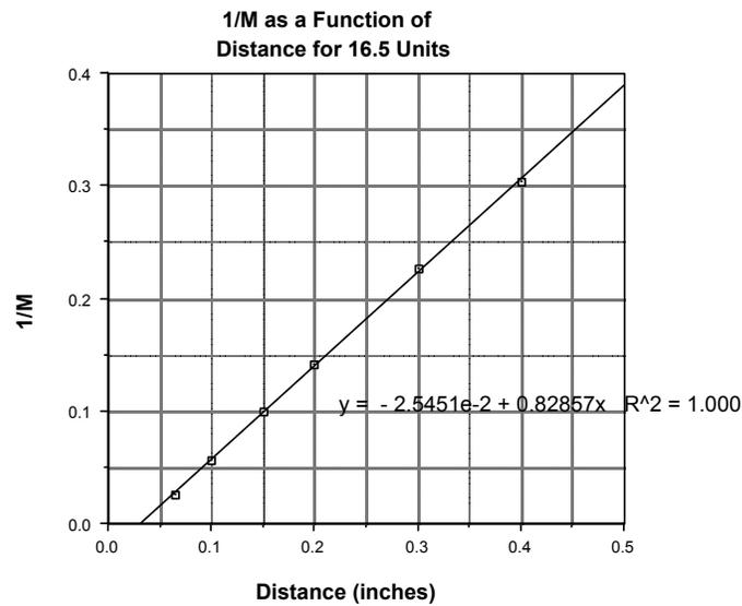
Figure 5. Normalized 1/M as a function of separation for  $^{235}\text{U}$ -SiO<sub>2</sub>-polyethylene experiment.
