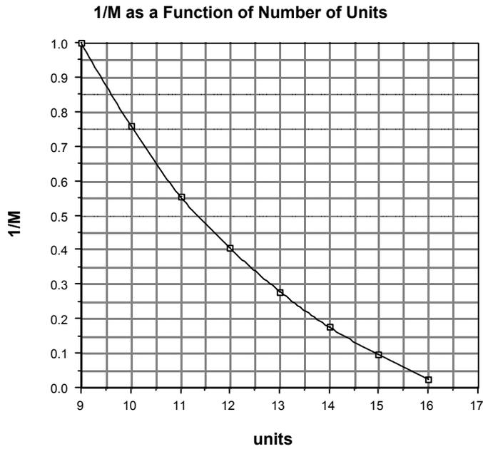
Figure 4. Normalized 1/M as a function of highly enriched HEU foils for  $^{235}\text{U}$ -SiO<sub>2</sub>-polyethylene experiment. Two HEU foils represent a unit.
