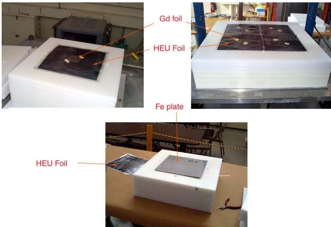
Figure 3. Gadolinium and iron critical--mass experiments.
