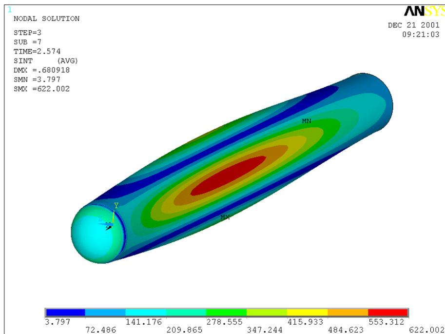
Figure 10. Total Stress Intensity (MPa) contour plot for external pressure of 5.74 MPa using irradiated HT-9 with 25 dpa
