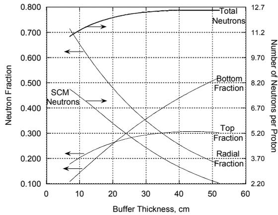
Figure 3. Neutron source yield as a function of the LBE buffer thickness
