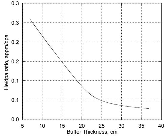
Figure 5. Helium/atomic displacement ratio as a function of the buffer thickness
