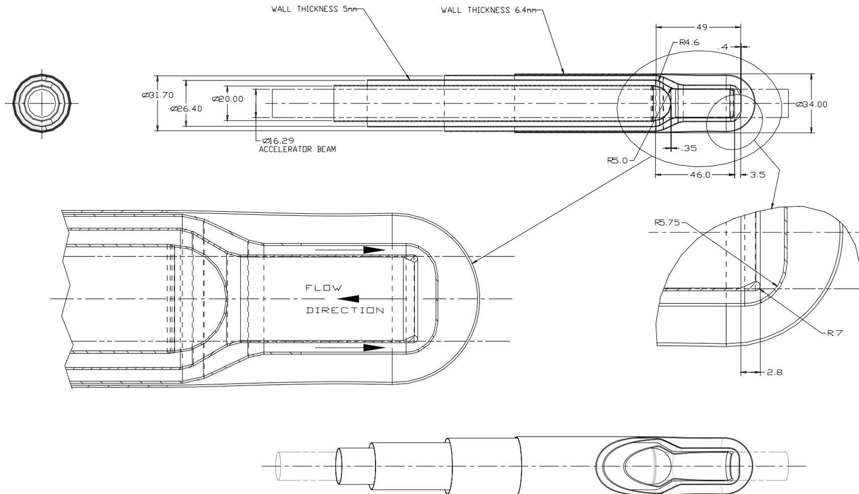
Figure 1. Lead-bismuth eutectic target design
