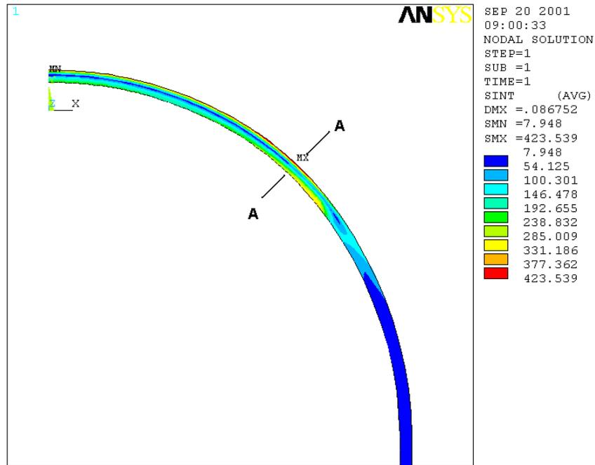
Figure 9. Stress intensity (Pa) in the 3.5-mm hemi-spherical beam window during the normal operating conditions
