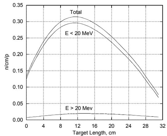
Figure 7. Neutron source distribution along the outer buffer surface
