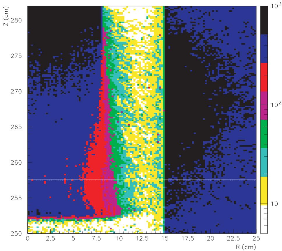
Figure 14. SCM-100 energy deposition distribution with the lead-bismuth target, W/cm<sup>3</sup>
