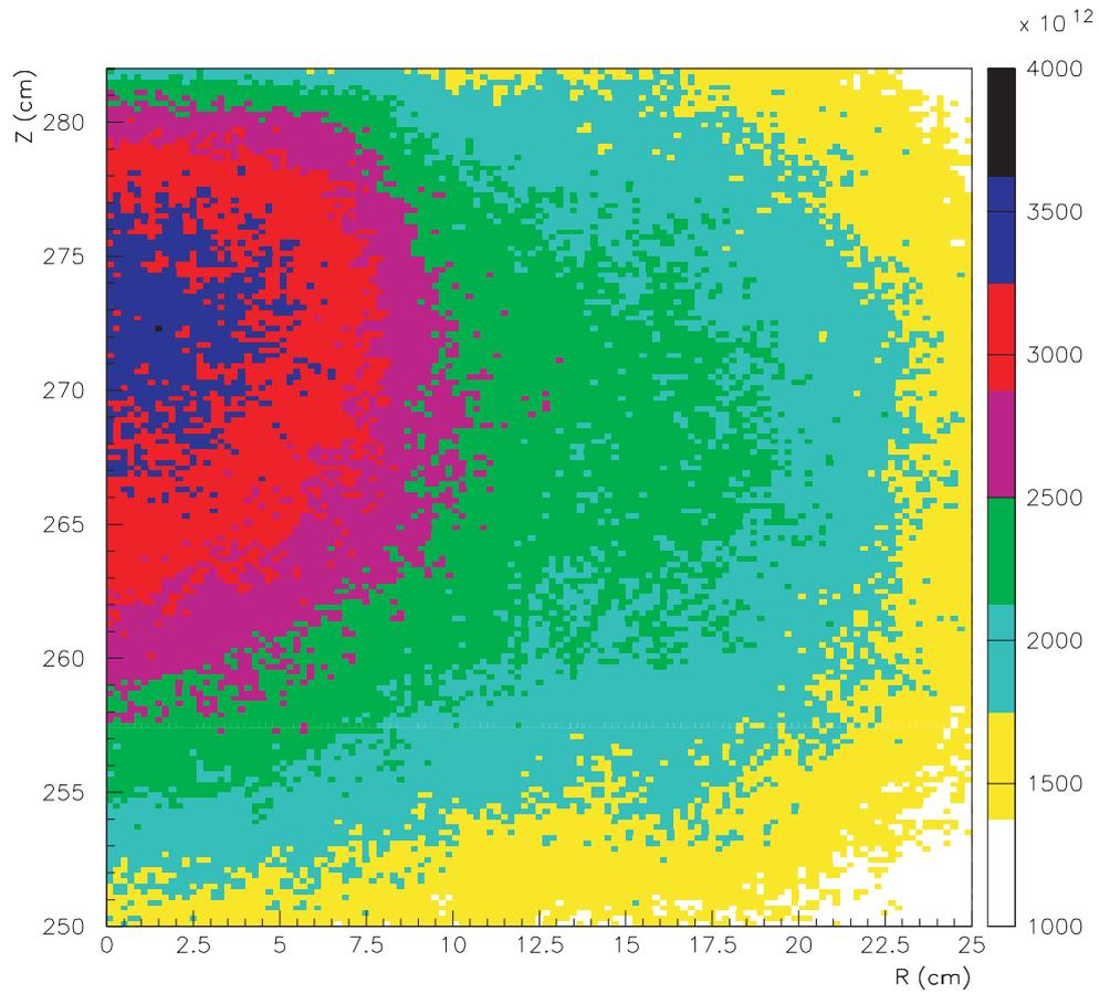
Figure 13. SCM-100 fast neutron flux (0.1 to 20 MeV)  $n/cm^2/s$  with the lead-bismuth target
