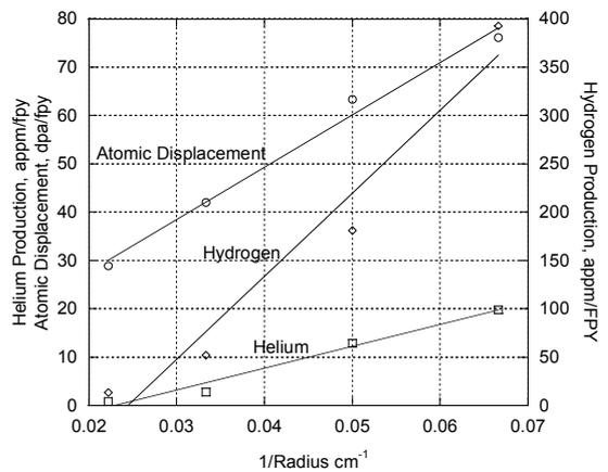
Figure 4. Midplane nuclear responses in the outer buffer structure as a function of the reciprocal of the LBE outer buffer radius
