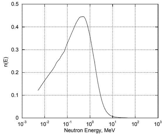
Figure 6. Neutron source spectrum
