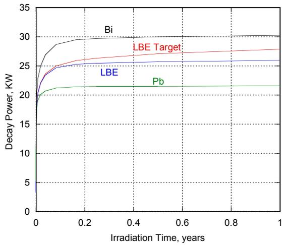
Figure 11. Buildup of decay power in a bismuth, lead, or LBE cylindrical geometry compared to LBE target material
