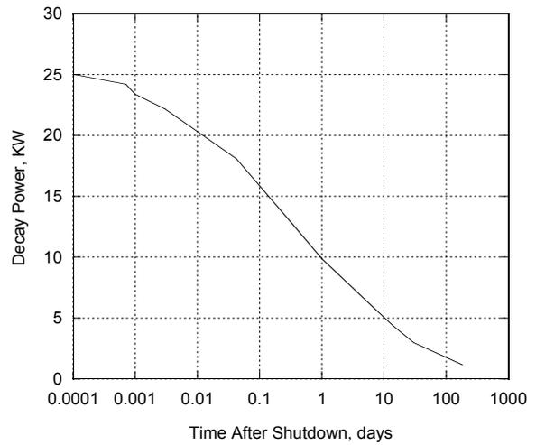
Figure 12. Decay power from the LBE target material as a function of time after shutdown
