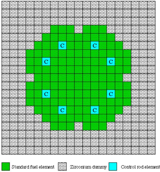
Figure 3. Minimal critical configuration of TREAT
