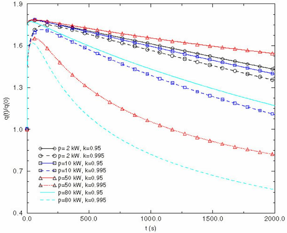
Figure 6. Source initiated power excursions in TREAT. At  $t=$ s the accelerator power is increased by the factor 1.8.
