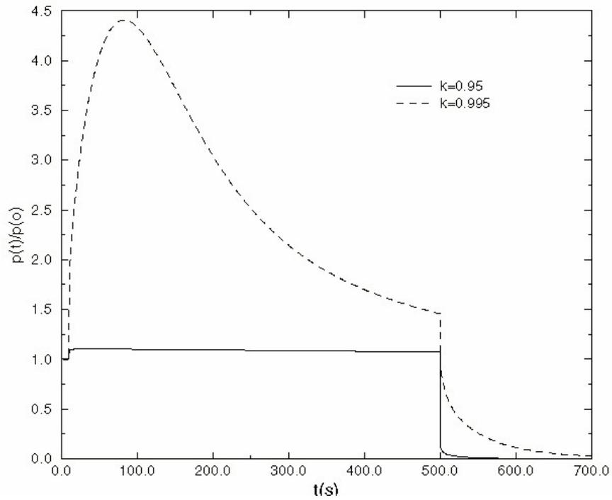
Figure 7. Control rods initiated power excursion in TREAT at 50 kW. Insertion of 500 pcm of reactivity at  $t=10$  s. At  $t=500$  s the accelerator is shut down.
