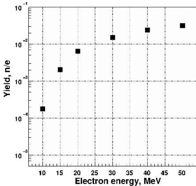
Figure 2 The photoneutron yield produced from a cylindrical as a function of the electron beam energy from a 3 cm thick target.
