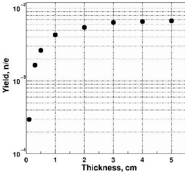
Figure 1. The photoneutron yield produced from a cylindrical U target for 20 MeV electrons incident on target of various thickness
