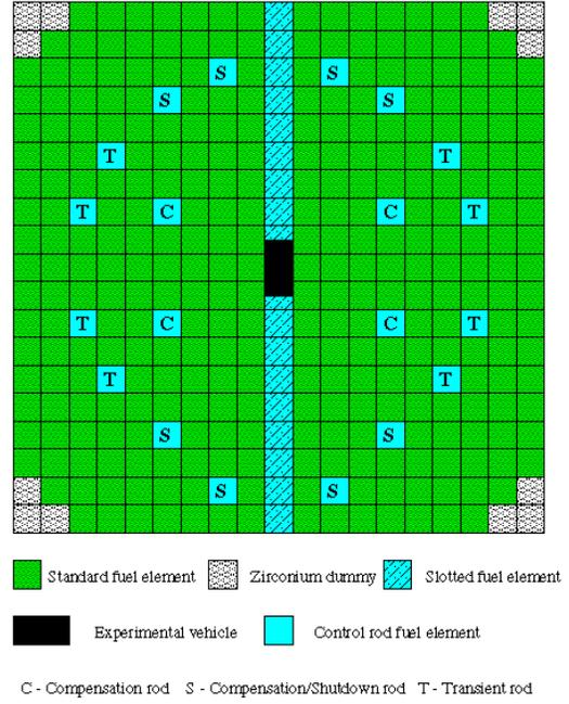
Figure 4 M8CAL critical configuration
