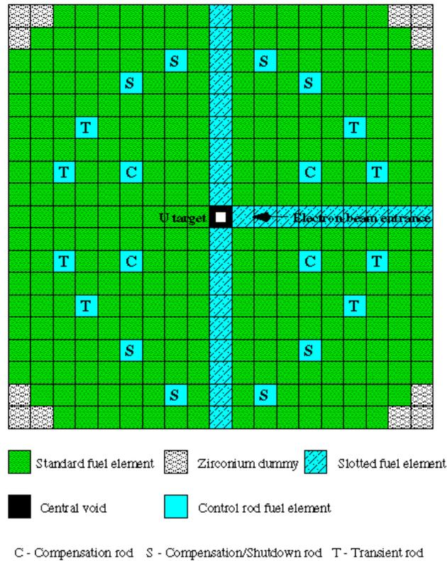
Figure 5. Proposed setup of the TREAT core for TREACS experiments
