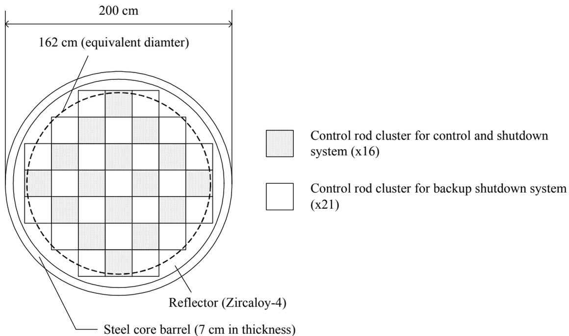
Figure 2. Cross sectional view of the PSRD-100 core.
