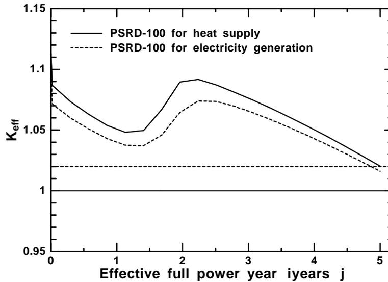
Figure 4. Burn-up characteristics of the PSRD-100 core.
