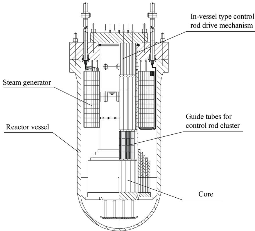
Figure 1. Conceptual drawing of the PSRD-100.
