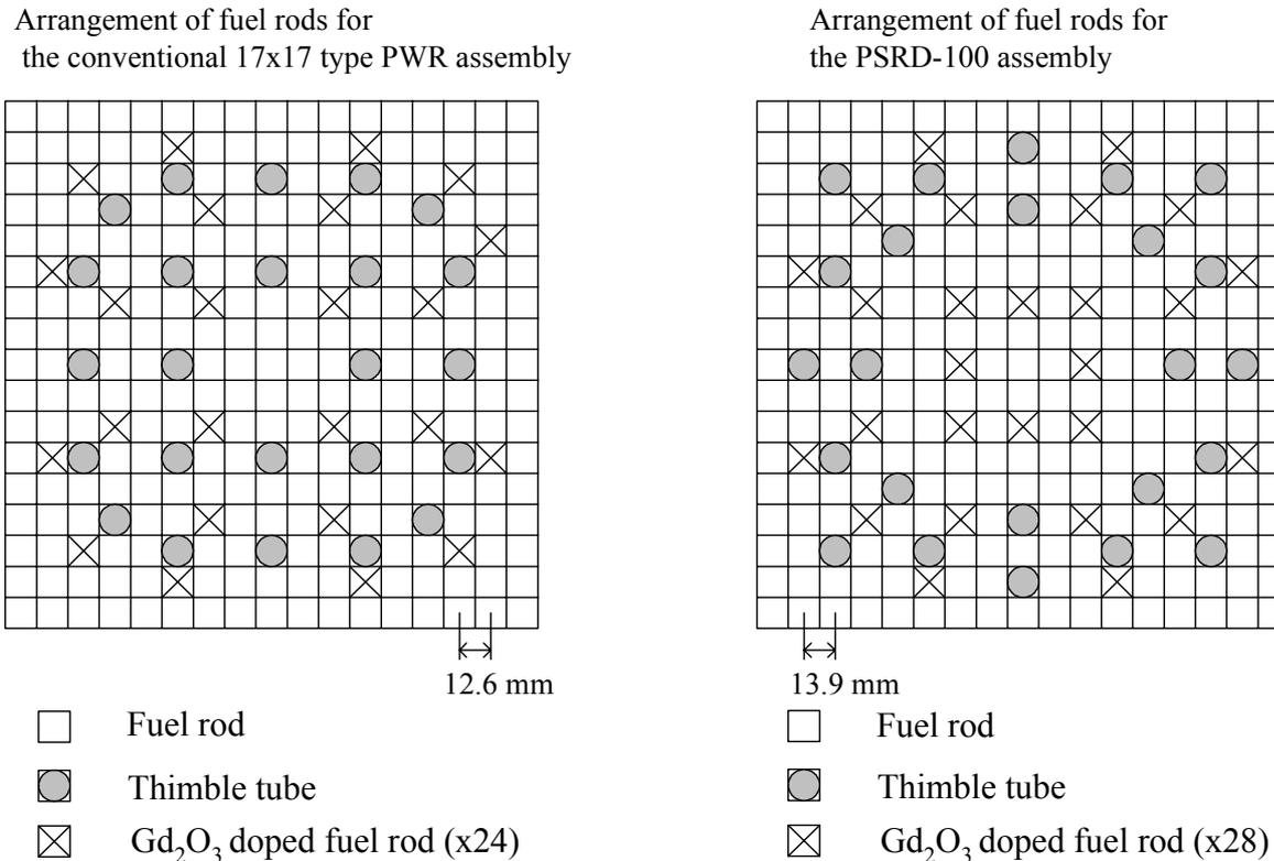
Figure 3. Arrangement of fuel rods in assembly.
