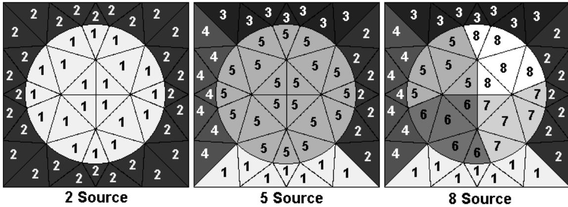
Figure 2. Two, Five, and Eight Lumped Source Representations of the Pin-cell Geometry
