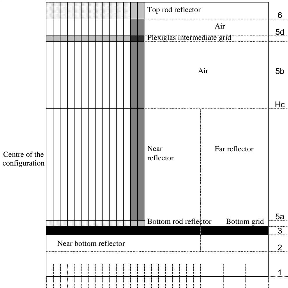
Figure 4. XZ view of the 3D model of the REBUS configuration #1 (reference case). The number of the axial layer is explained in the text. Layer 5 is subdivided into four regions in account of the interface flooded/non-flooded fuels and of the intermediate plexiglas grid.
