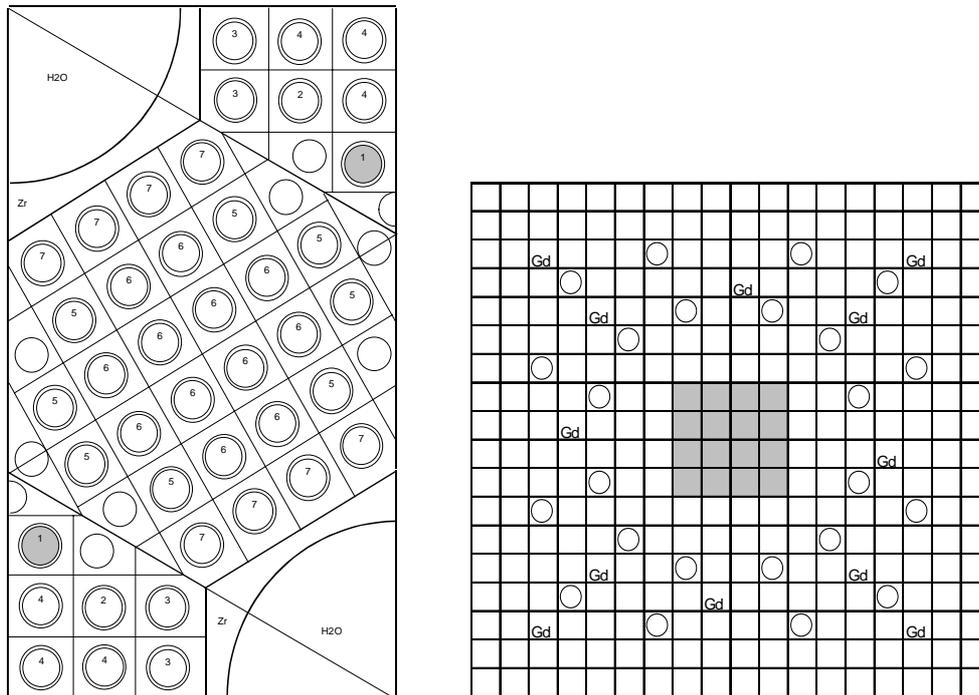
Figure 3. Geometrical model for the depletion calculation. On the left, a macro-assembly model for the representative MOX rod (indicated by the shaded cell) to be depleted up to 20.3 GWd/t<sub>M</sub>. On the right, a 18×18 assembly whose central 16 rods indicate the representative rod to be depleted up to 54.0 GWd/t<sub>M</sub>.
