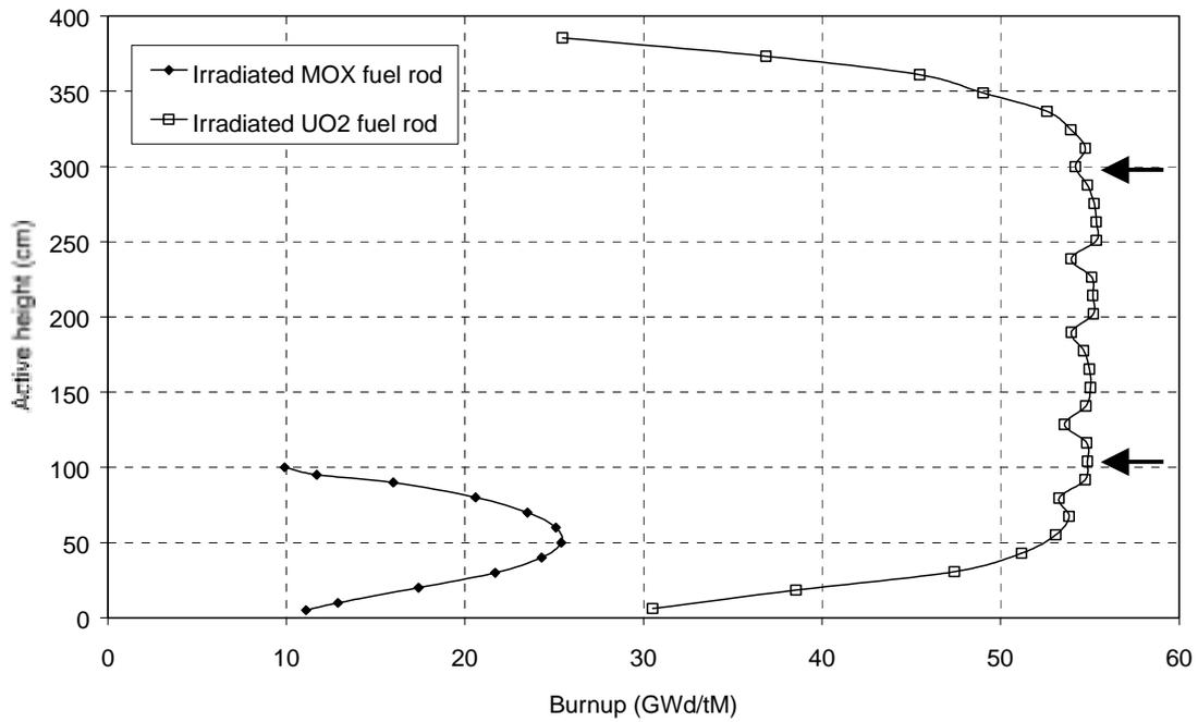
Figure 2. Axial burnup profile of one BR3 MOX and one GKN UO<sub>2</sub> fuel rods. Notice that only the central 2 meters section (see arrows) of UO<sub>2</sub> rods is to be used.
