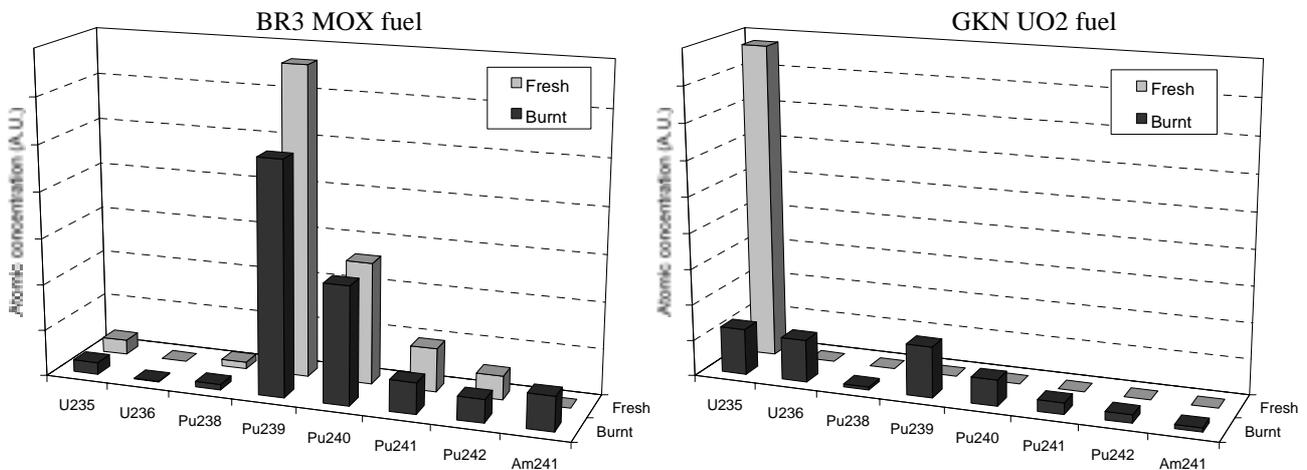
Figure 6. Comparison of the actinides vector of the couples fresh / irradiated fuels.
