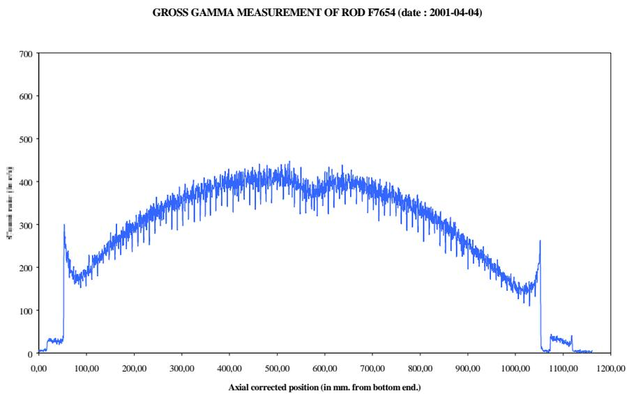
Figure 5. Example of a gross-gamma scan on an irradiated BR3 MOX fuel rod.
