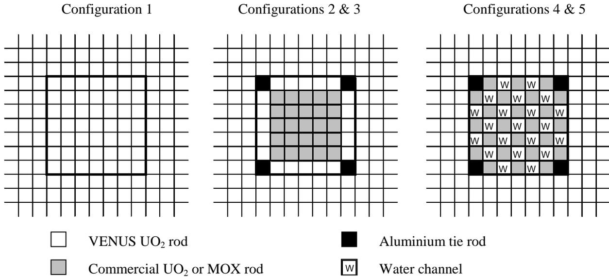
Figure 1. Centres of the critical configurations to be loaded in VENUS in the frame of REBUS-PWR
