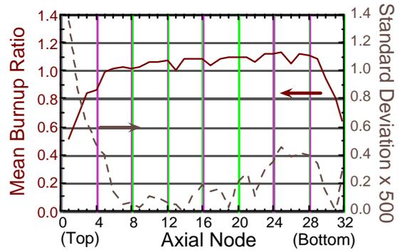
Figure 7. The mean and standard deviation of normalized axial burnup shapes in fuel assemblies received from the Nuclear Power Plant Neckarsheim II, as a function of the node number.
