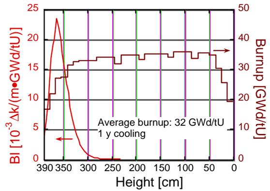
Figure 8. The burnup importance calculated for Phase II-C model in the mean burnup shape.
