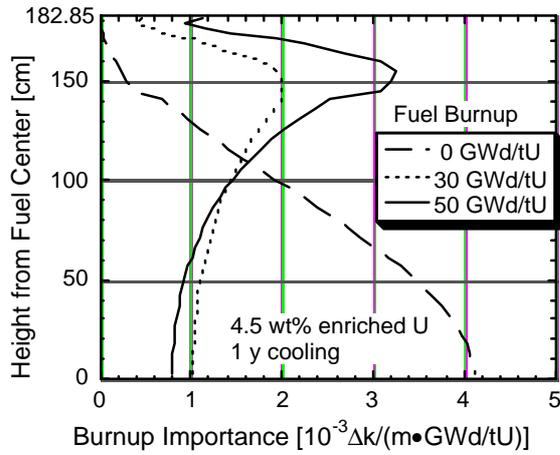
Figure 4. Burnup importance calculated for various burnups (1 y cooling).
