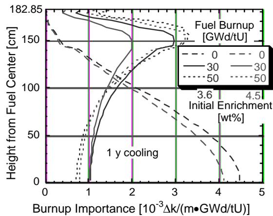
Figure 6. Burnup importance for the cases of the initial enrichment of 3.6 wt% compared with those of 4.5 wt%.
