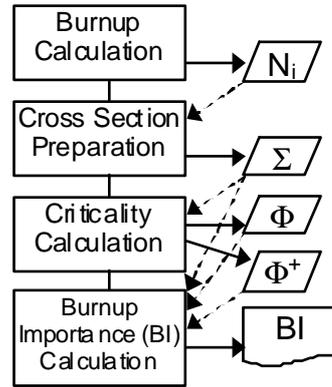
Figure 2. Calculation flow for burnup importance function.
