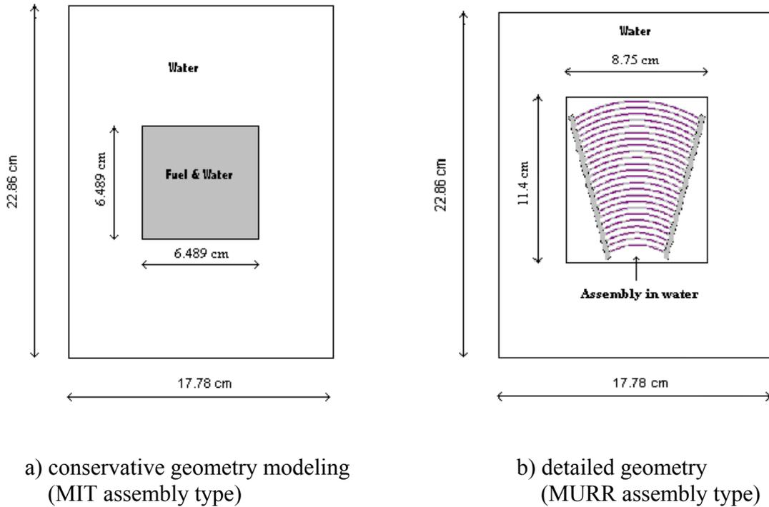
Figure 1. Typical Lattice Cell Configuration
