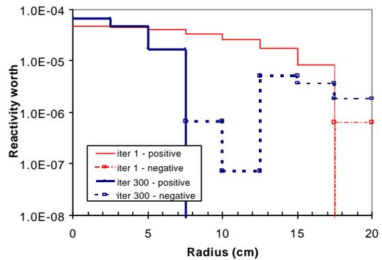
Fig. 15 Reactivity worth of Poly versus Be for Illustration # 3
