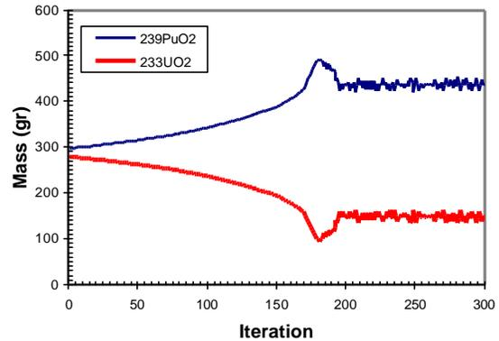
Fig. 7 Evolution of  $^{239}\text{PuO}_2$  and  $^{233}\text{U}$  mass. Illustration # 2
