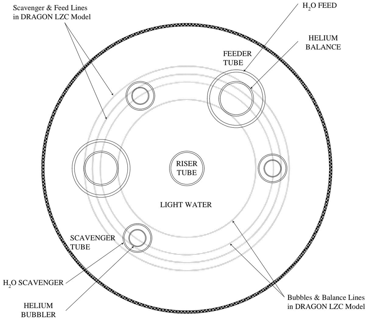
Note: The riser tube is located on the top of the calandria and does not extend into the core; therefore, it was not taken into account in the DRAGON model for zone controllers.
