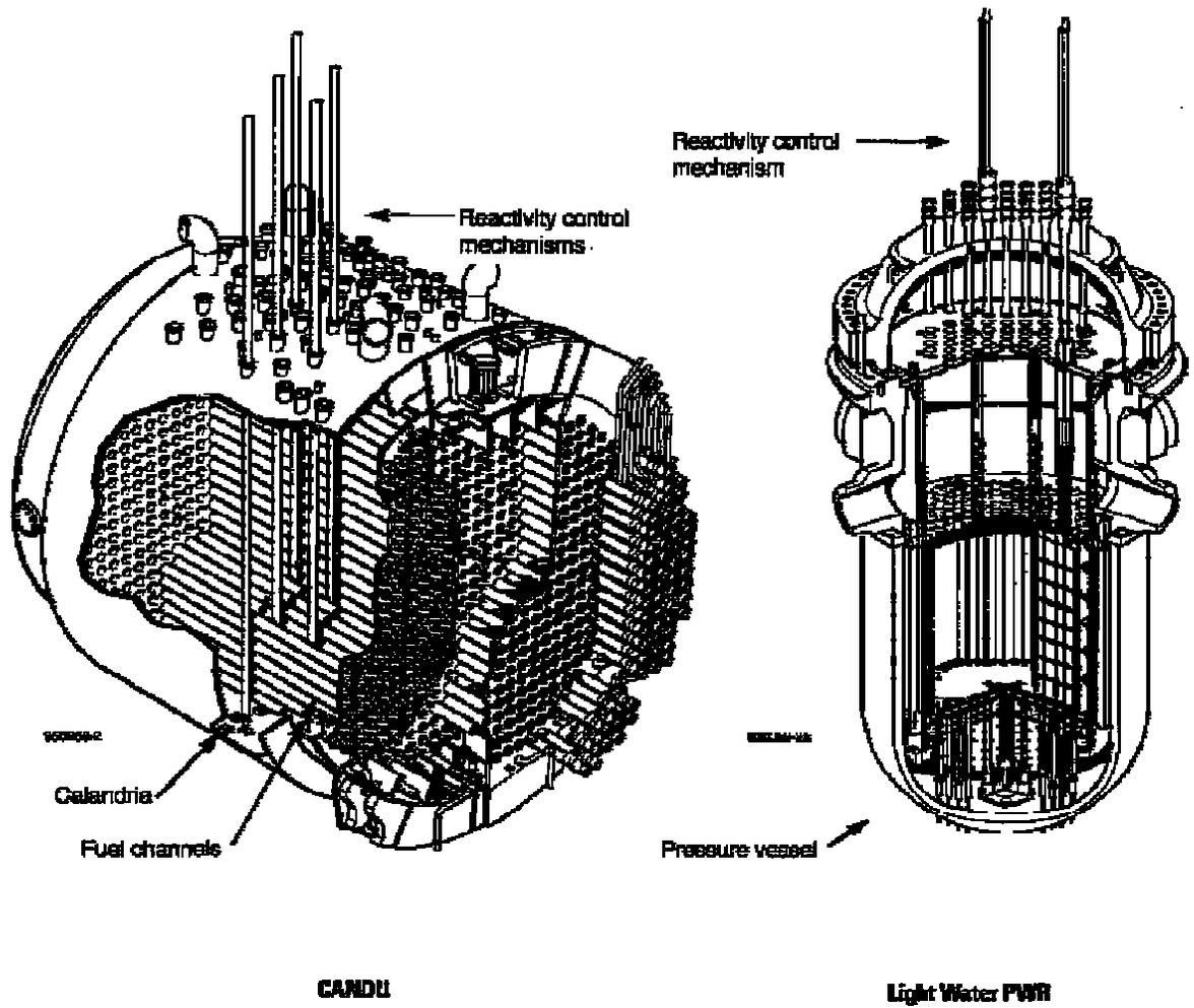
Figure 1. Layout of a CANDU-6 Reactor Compared with a PWR
