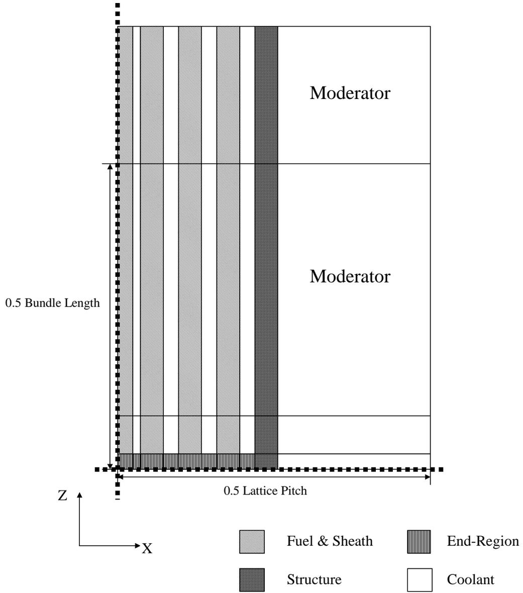
Figure 8. Supercell Modelling of End Region for 37-Element NU fuel, in Bundle-Bundle Contact Configuration (X-Z Layout, Right-half Only)
