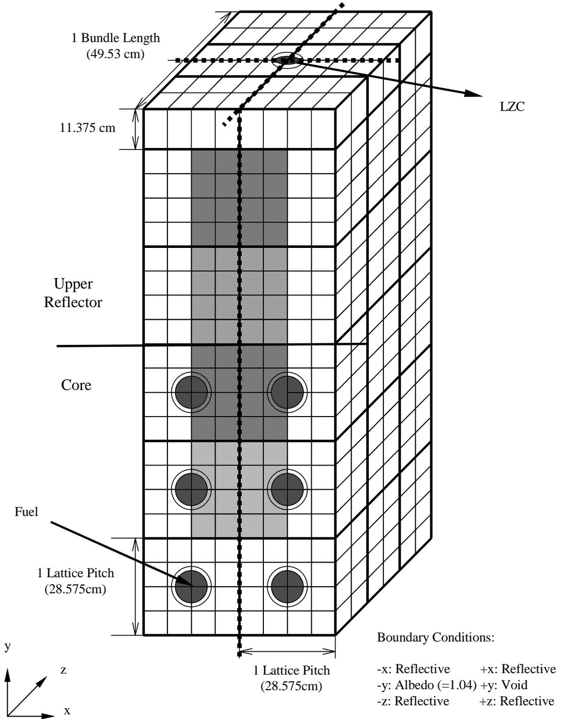
Figure 6. Supercell Modelling of a LZC in the Upper Reflector with DRAGON
