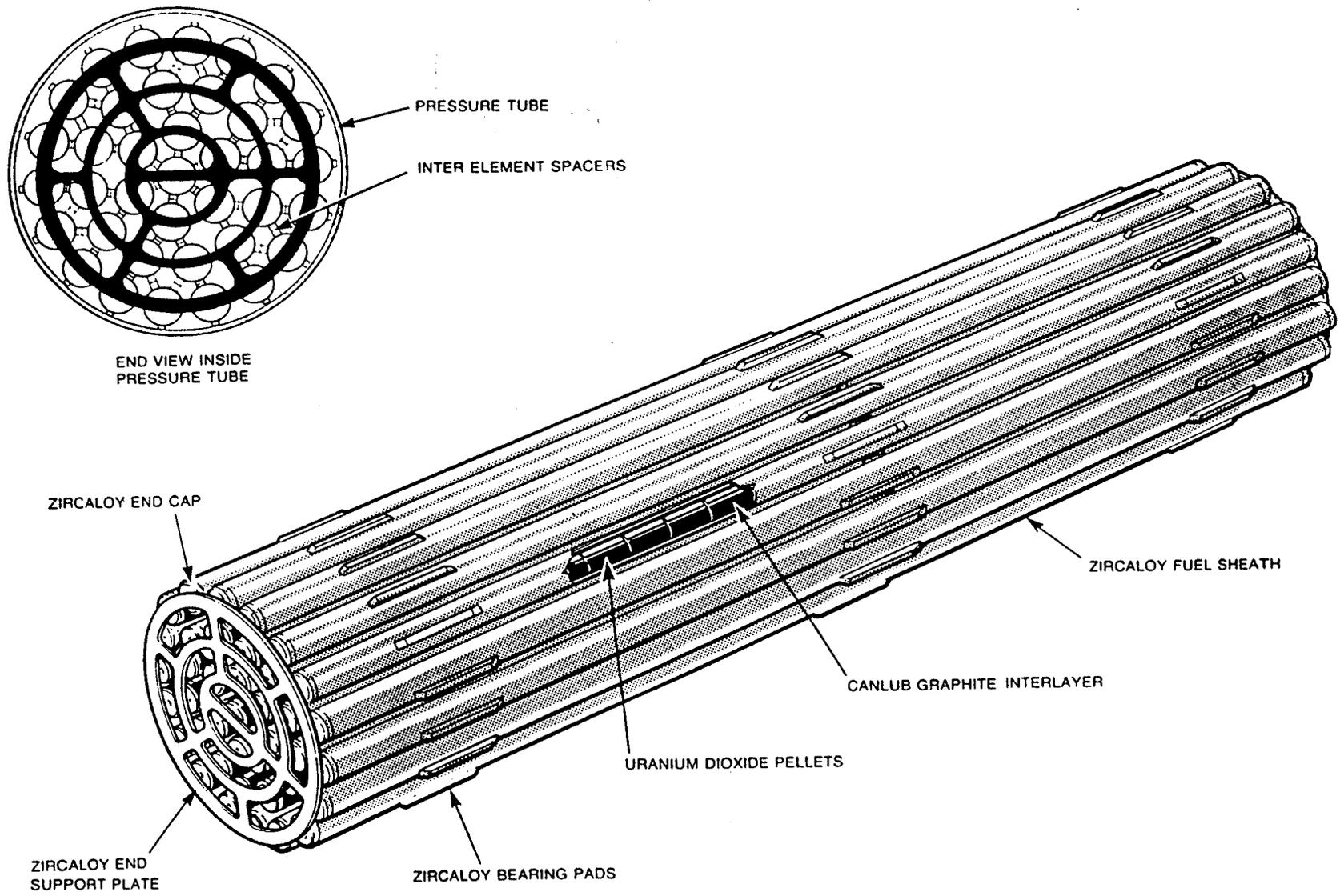
Figure 7. Schematic Representation of a CANDU-6 Fuel Bundle
